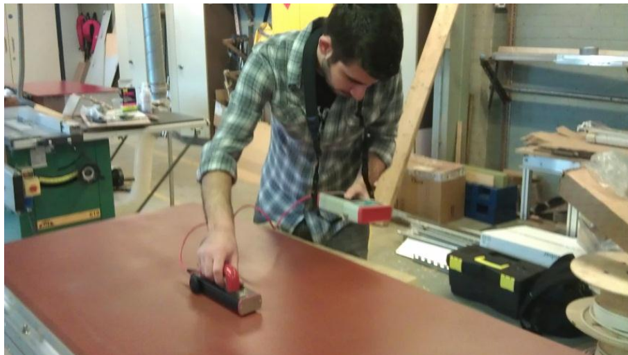
Figure 4.19: Measurement of the roughness of F0037 using a TQC Hull Roughness Gauge.
