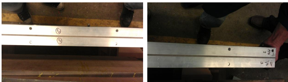
Figure 4.11: Top view of the plates with connection holes.
