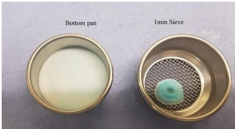
Figure 4-5 Sieving Assembly for glass beads.
