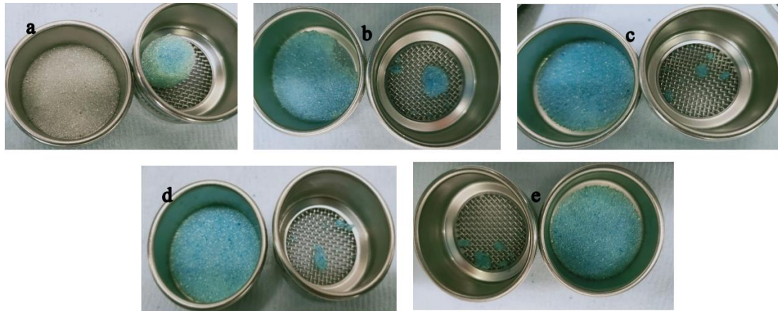
Figure 8-1 0.01 g/ml PCM/Methanol dried sample (a) after manual tapping (b) after 1st sieving cycle (c) after 2nd sieving cycle (d) after 3rd cycle of sieving (e) after 4th cycle of sieving
