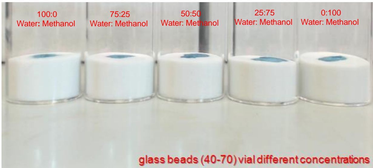
Figure 6-19 Glass beads wetted with different compositions of water & methanol solution (at the start of the Experiment)
