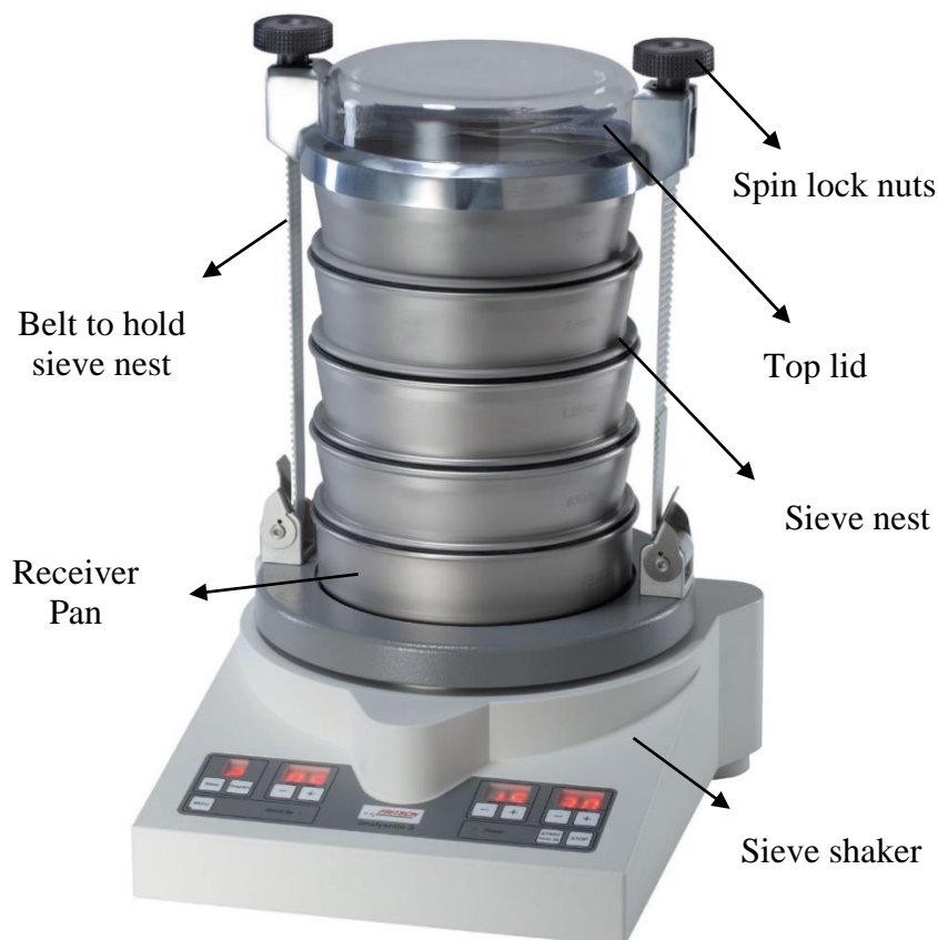
Figure 7-1 Sieve shaker assembly with sieve nest
