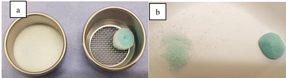
Figure 5-1 Fructose/water system (a) Sample after manual tapping (b) sample after four cycles of sieving.
