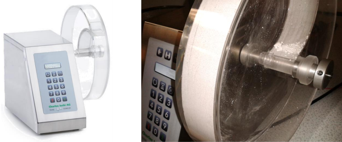
Figure 8-2 Friability tester or Friabilator (Charles Ischi AG – Testing Technology)
