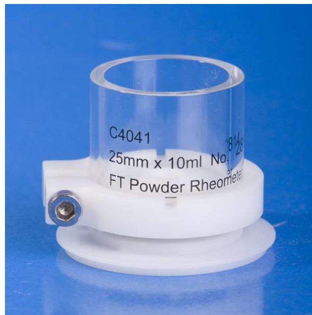
Figure 9-5 25mm x 10ml split vessel with bottom assembly (FT4 support document – 25mm Vessel Assemblies – W7021)
