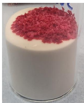
Figure 7-20 Glass beads (GB1) dried sample with the benzoic acid solution in binary mixture of heptane and ethanol (95:05)
