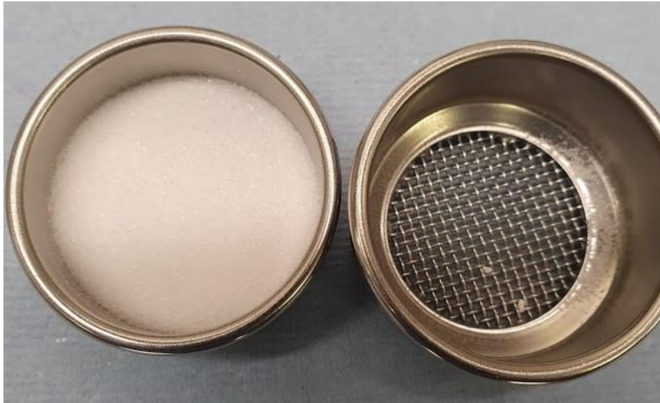
Figure 7-6 Dry sample after transferring to sieving assembly of 1mm sieve and bottom pan
