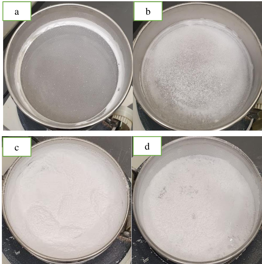
Figure 7-7 Sieved fractions of PCM with 20 cm diameter (a) 500 um sieve (b) 212um Sieve (c) 75 um sieve (d) bottom pan
