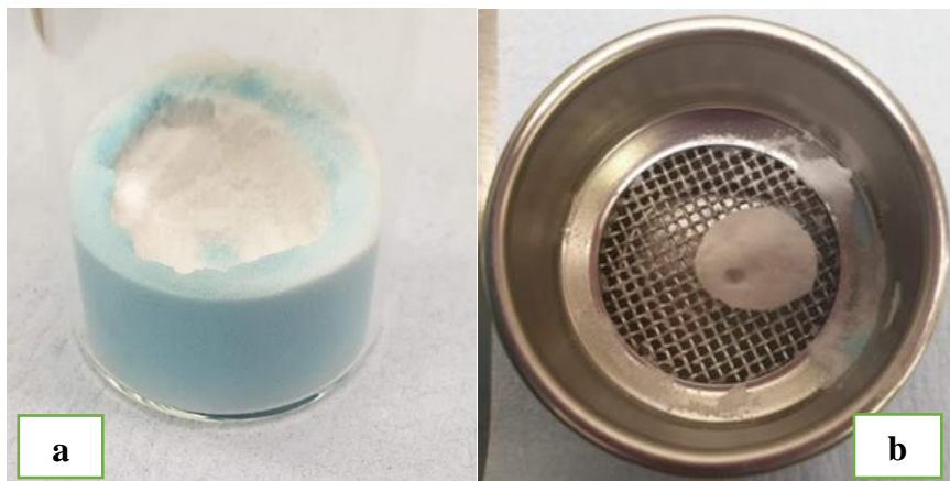
Figure 6-4 Dried sample PCM/Water system (a) dye dispersed in the loose beads transporting towards the wall (b) agglomerate formed free from dye
