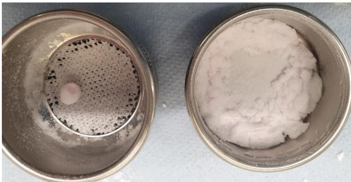
Figure 7-11 Sieving assembly after the first cycle of sieving of 75 \mu\text{m} fraction sample
