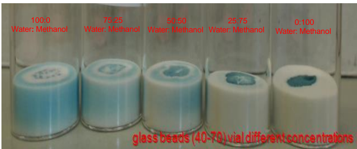
Figure 6-20 Dry samples of glass beads wetted with different compositions of water & methanol solution (after completion of the experiment)
