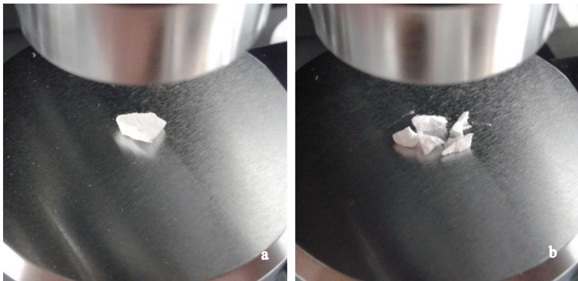
Figure 8-4 Fragmentation of particle agglomerate during compression test (Simurda, 2017)
