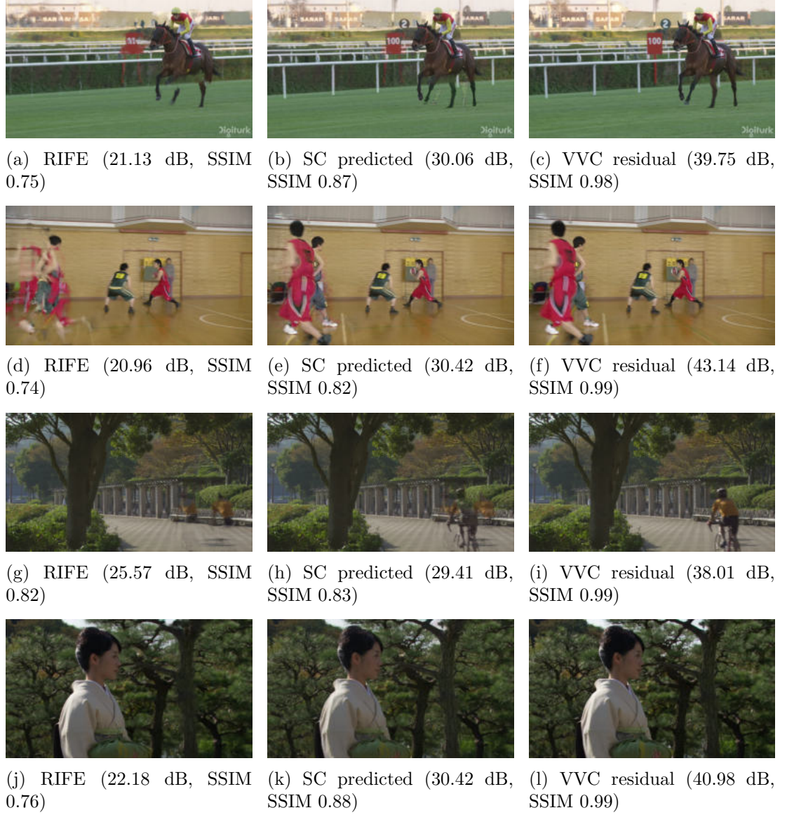
Figure 4.8: Visual comparison of progressive reconstruction quality across four representative test frames (rows). Each column shows: (left) the RIFE-based bidirectionally interpolated prediction, (centre) the context-conditioned semantic communication (SC) prediction from the autoencoder, and (right) the final reconstruction after VVC residual correction. PSNR and SSIM values are reported per frame. Quality improves monotonically from left to right across all examples, validating the complementary roles of motion-aligned interpolation, semantic encoding, and residual correction.
