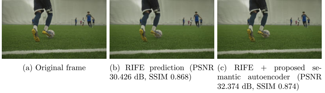
Figure 3.23: Prediction quality comparison illustrating the complementary roles of RIFE and the proposed semantic autoencoder. Combining RIFE with the per-GOP trained semantic autoencoder achieves a 1.95 dB PSNR improvement over RIFE alone [22].
