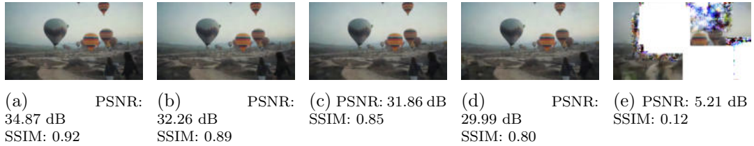
Figure 6.6: Visual comparison of SMDC reconstruction quality under different reception scenarios. From left to right: (a) all three descriptions received; (b) any two descriptions received; (c) single description without bit errors; (d) single description at \text{BER} = 0.001 ; (e) single description at \text{BER} = 0.01 .
