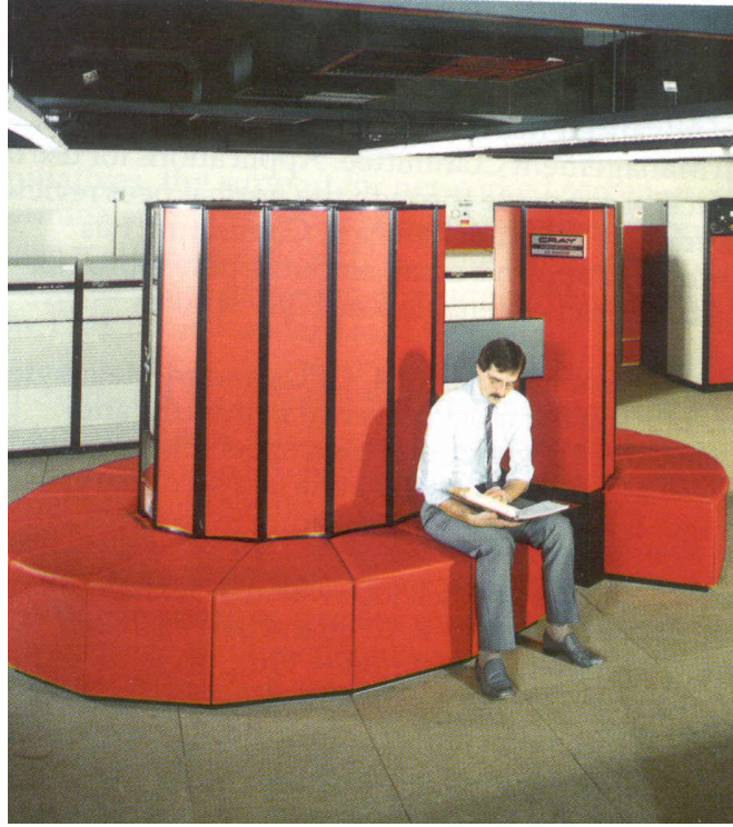
Figure 1.5: Cray X-MP, example of supercomputer design in the '80s, based on vector processors.
