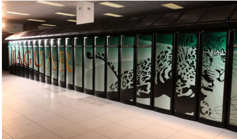
Figure 1.6: Cray Jaguar, an example of a modern MPP system, rated the third fastest supercomputer in the world in June 2011.
