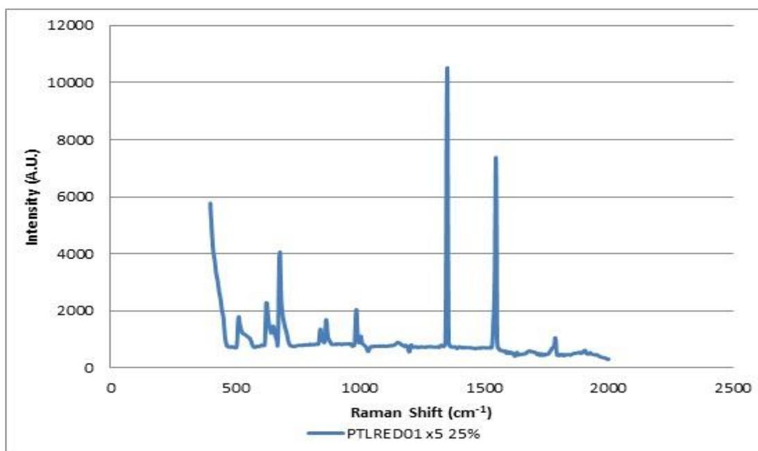
Figure 6.16: Example spectra of a PTL UK red gel ink spot on glass slide (FORAM 785 25% laser power/x 5 obj., 1.0s default scan time (no light collar))
