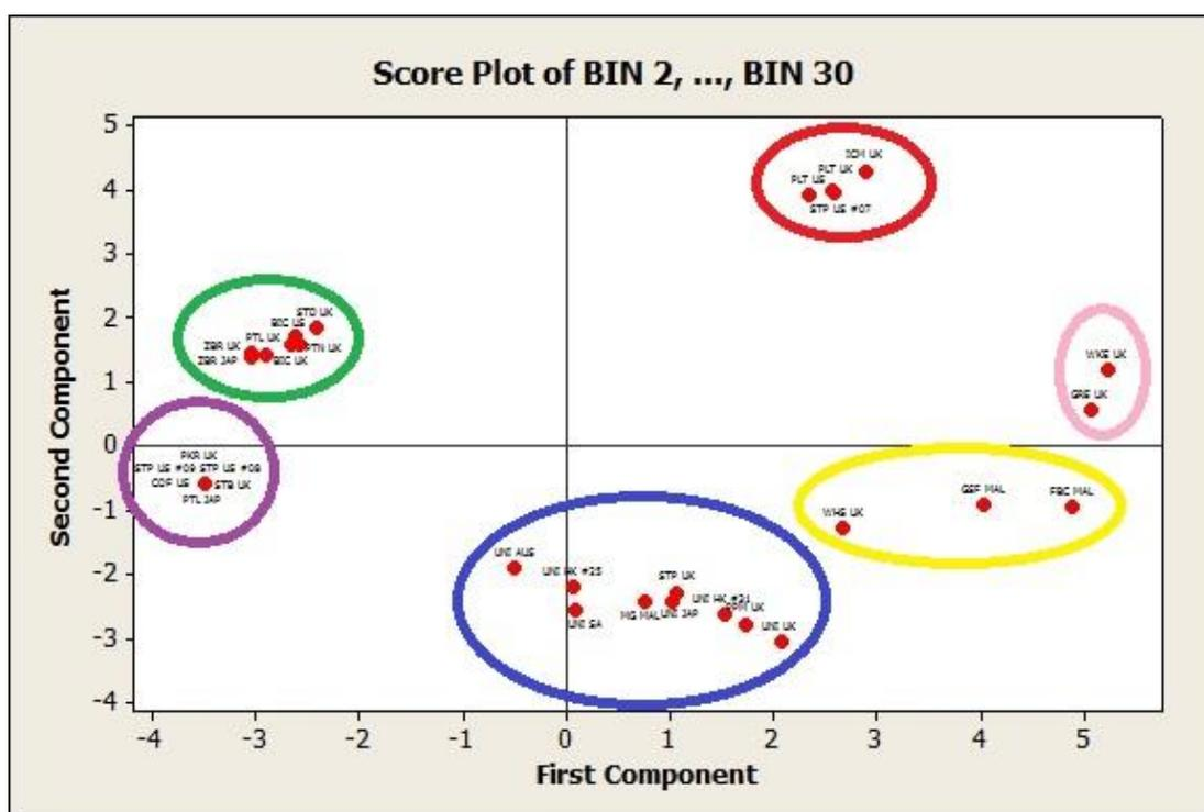
Figure 7.1: PCA score plot of blue ink group samples analysed by Renishaw InVia 514.5 nm demonstrating successful discrimination into six clusters
