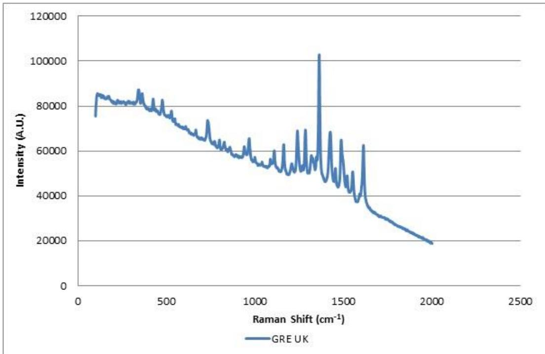
Figure 6.86: Brand/model combination of red gel ink forming Group 7 (Renishaw InVia 785 nm 100% laser power/x 50 obj.)
