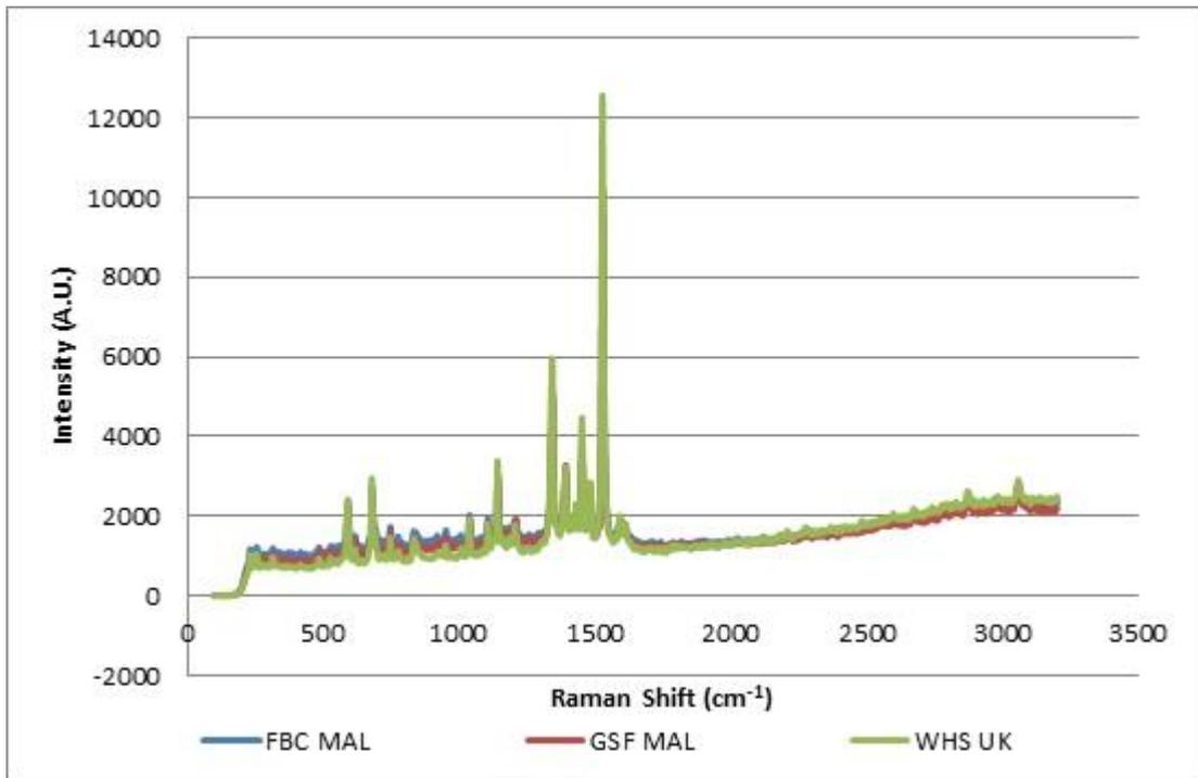
Figure 6.27: Brand/model combinations of blue gel ink forming Group 3 (Renishaw InVia 514.5 nm 10% laser power/x 20 obj.)
