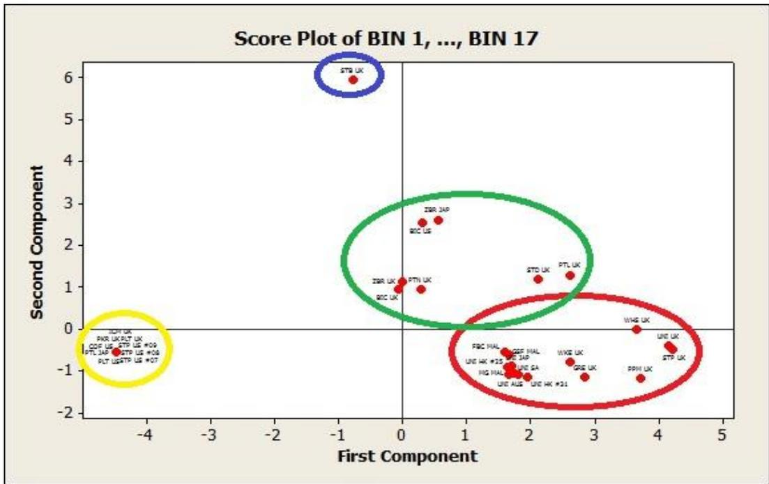
Figure 7.10: PCA score plot of blue ink group samples analysed by Renishaw InVia 785 nm demonstrating successful discrimination into four clusters
