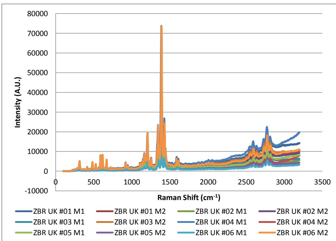
Figure 6.21: Spectra from ZBR UK pens #01 – 06 demonstrating no evidence of within brand variation, contradicting the findings at 785 nm (Renishaw InVia 514.5 nm 10% laser power/x 20 obj.)
