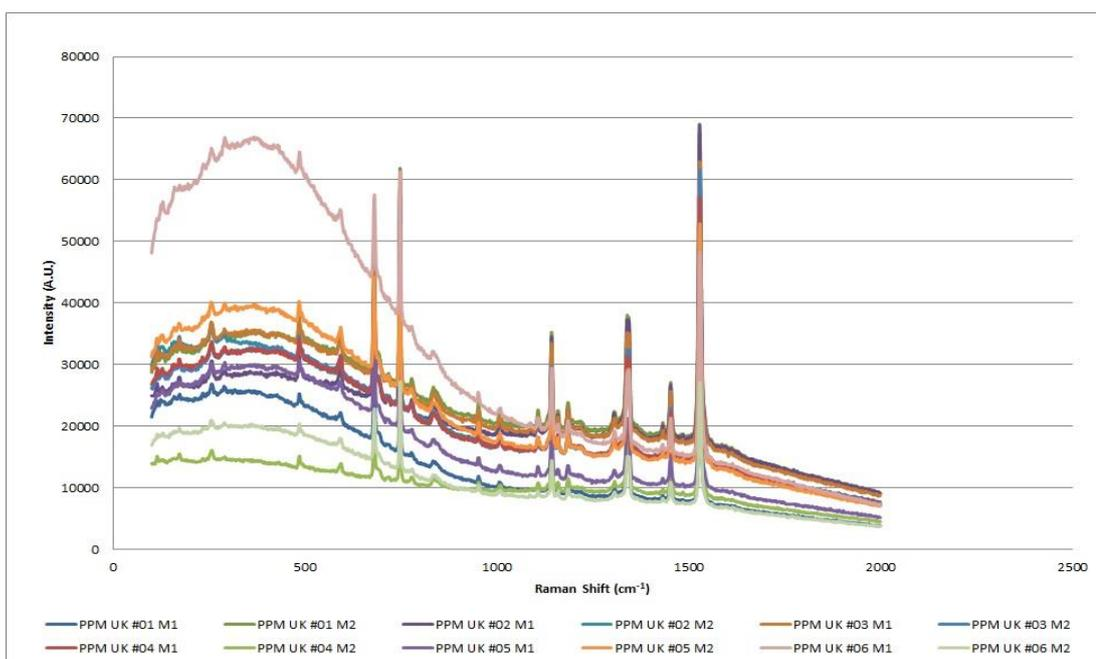
Figure 6.38: Set of 12 spectra from PPM UK blue gel ink illustrating minor variation in background fluorescence shape (Renishaw InVia 785 nm 10% laser power/x 50 obj.)
