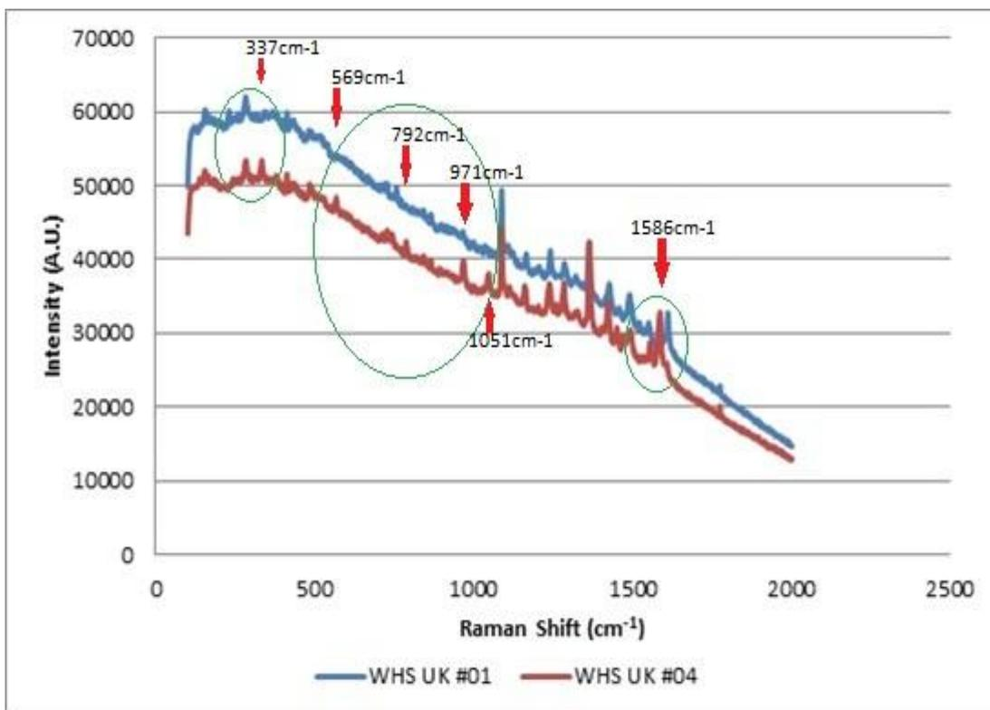
Figure 6.23: Comparison of spectra from WHS UK #01 'v' WHS UK #04 red gel ink on paper demonstrating within brand variation (Renishaw InVia 785 nm 100% laser power/x 50 obj.). Regions of difference highlighted within green circles with specific wavenumber positions identified by red arrows
