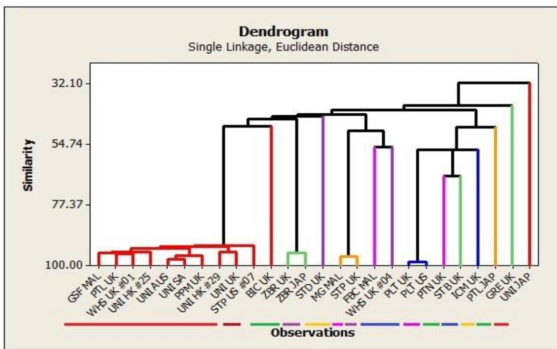
Figure 7.36: HCA dendrogram of red ink group samples analysed by FTIR-ATR demonstrating successful discrimination into 14 clusters in line with T1 level visual pattern recognition groups
