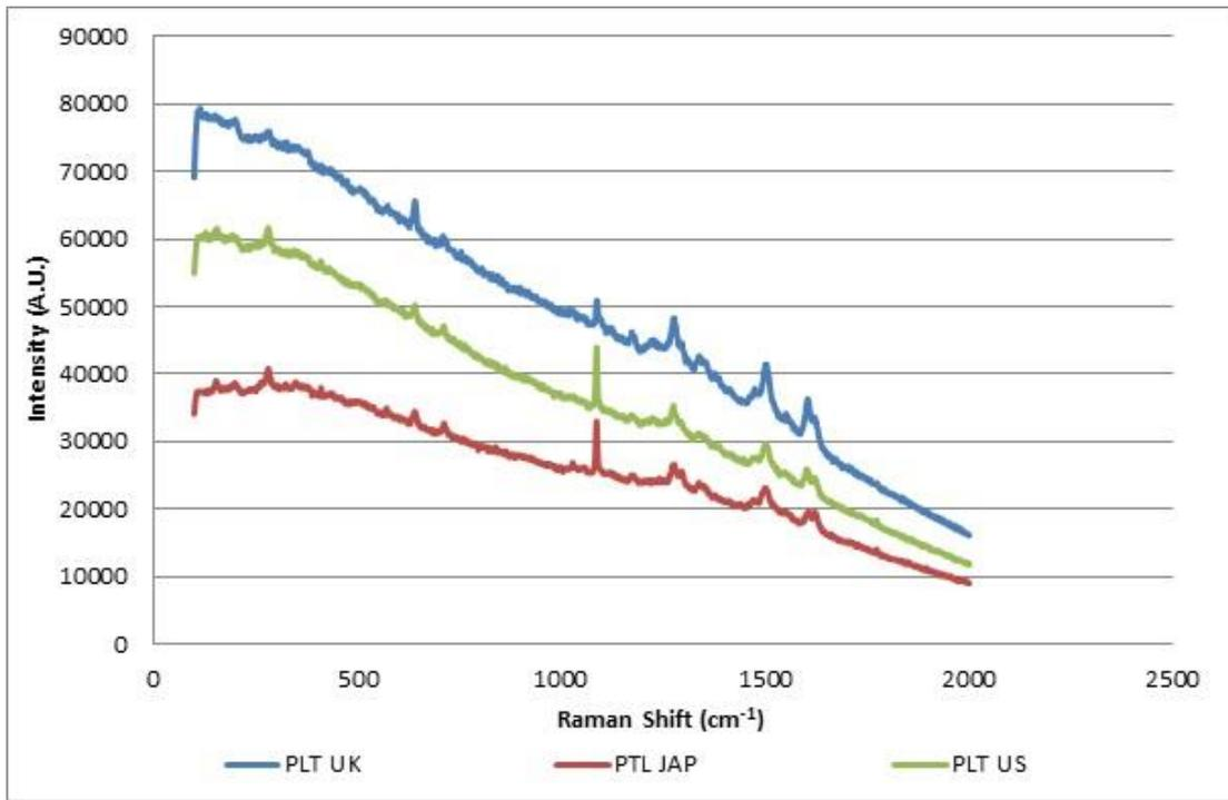
Figure 6.82: Brand/model combinations of red gel ink forming Group 3 (Renishaw InVia 785 nm 100% laser power/x 50 obj.)
