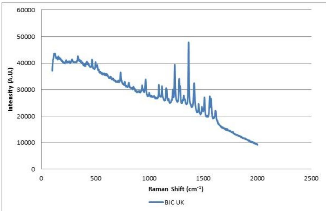
Figure 6.85: Brand/model combination of red gel ink forming Group 6 (Renishaw InVia 785 nm 100% laser power/x 50 obj.)
