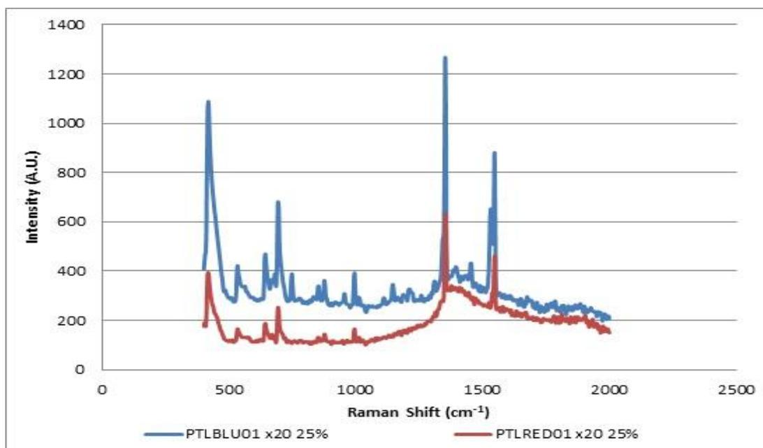
Figure 6.15: Comparison of spectra from PTL UK blue and red gel ink spot on paper demonstrating surprising similarity in spectral pattern (FORAM 785 25% laser power/x 20 obj., 1.0s default scan time)
