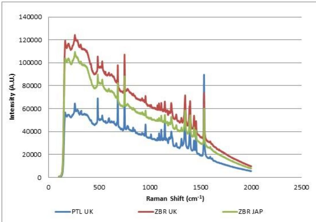
Figure 6.56: Brand/model combinations of blue gel ink forming Group 3 (Renishaw InVia 830 nm 10% laser power/x 50 obj.)
