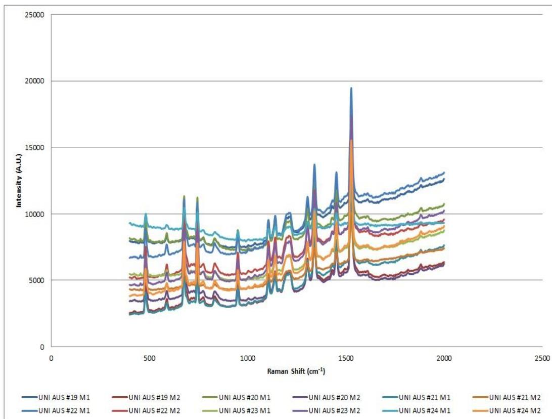
Figure 6.32: Duplicate spectra from each of blue UNI AUS pens #19 – #24 demonstrating good reproducibility and S:N ratio with only minor variation in background fluorescence shape (FORAM 685-2 10% laser power/x 20 obj., Auto Exposure)
