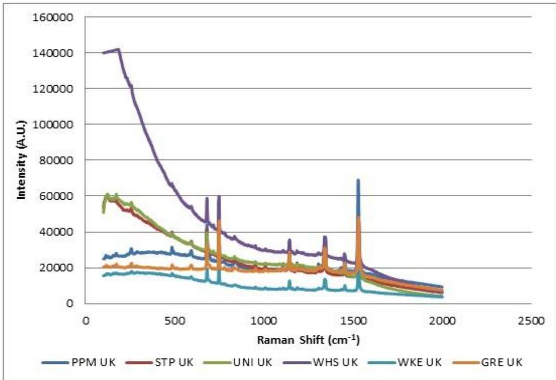
Figure 6.46: UK brand/model combinations of blue gel ink forming Group 1 (Renishaw InVia 785 nm 10% laser power/x 50 obj.)
