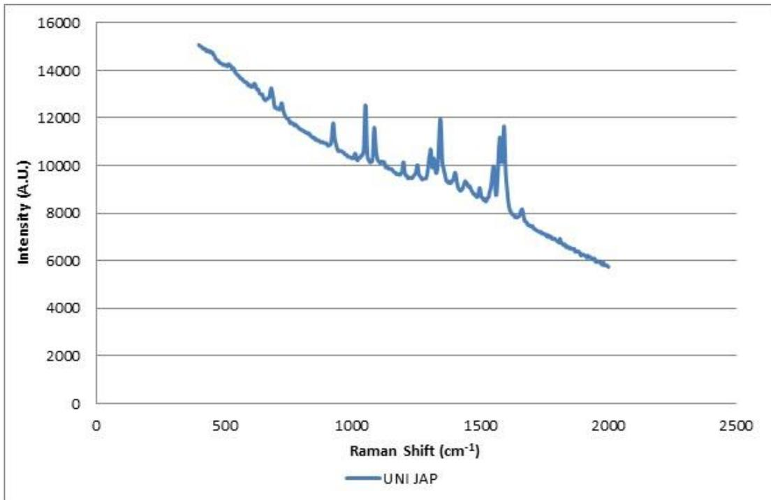
Figure 6.78: Brand/model combination of red gel ink forming Group 9 (FORAM 785 100% laser power/x 50 obj., Auto Exposure)
