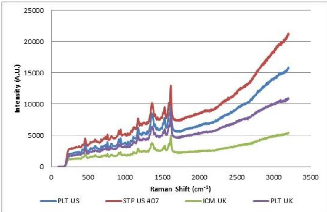
Figure 6.29: Brand/model combinations of blue gel ink forming Group 5 (Renishaw InVia 514.5 nm 10% laser power/x 20 obj.)
