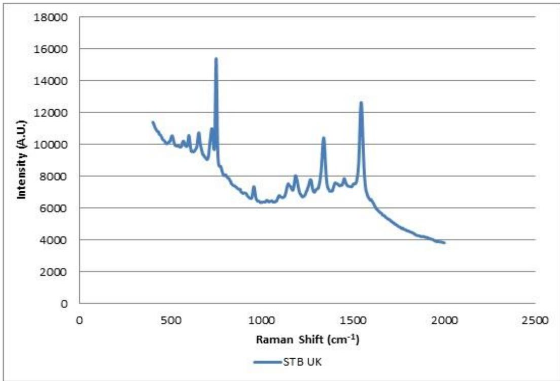
Figure 6.35: Brand/model combination of blue gel ink forming Group 3 (FORAM 685-2 10% laser power/x 20 obj., Auto Exposure)
