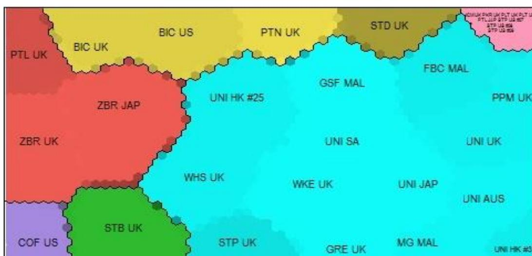
Figure 7.14: SOFM of blue ink group samples analysed by Renishaw InVia 830 nm demonstrating successful discrimination into six clusters. Variation in hue of coloured segments within a cluster indicative of subtle differences in the combined relative peak intensities for the wavenumbers characterising the ink samples within that cluster, i.e. STD UK exhibits a much greater difference to the other three ink samples within the yellow cluster representing Group 2
