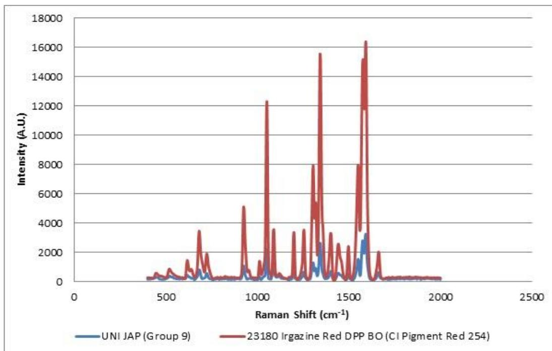
Figure 6.103: Red Ink Group 9, suggested pigment identification of Irgazine Red DPP BO (CI Pigment Red 254) (FORAM 785). NB Auto-scaling of the two sample spectra on the same axis gives a false impression of spectral differences, when spectra compared side by side a high level of similarity is observed
