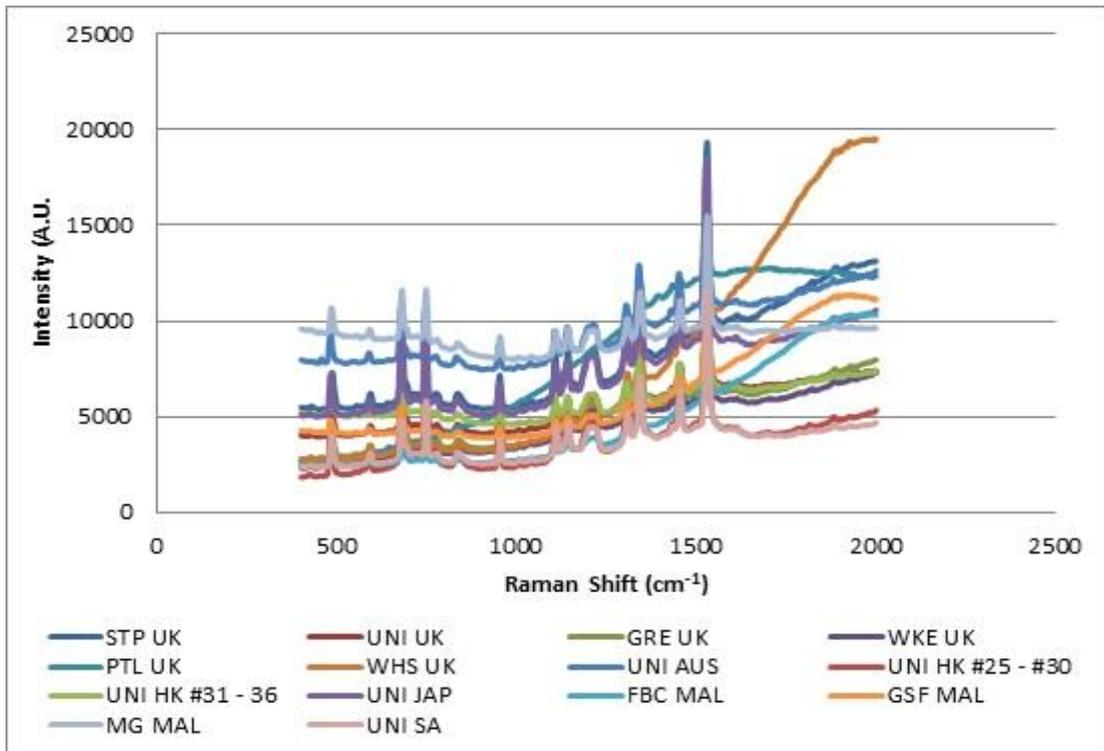
Figure 6.33: Brand/model combinations of blue gel ink forming Group 1 (FORAM 685-2 10% laser power/x 20 obj., Auto Exposure)
