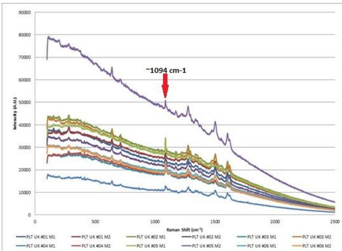
Figure 6.68: Spectra of PLT UK pens #01 - #06 red gel ink on paper demonstrating weak signal intensity (Renishaw InVia 785 nm 100% laser power/x 50 obj.). A peak attributable to the paper substrate at  $\sim 1094 \text{ cm}^{-1}$  highlighted by the red arrow
