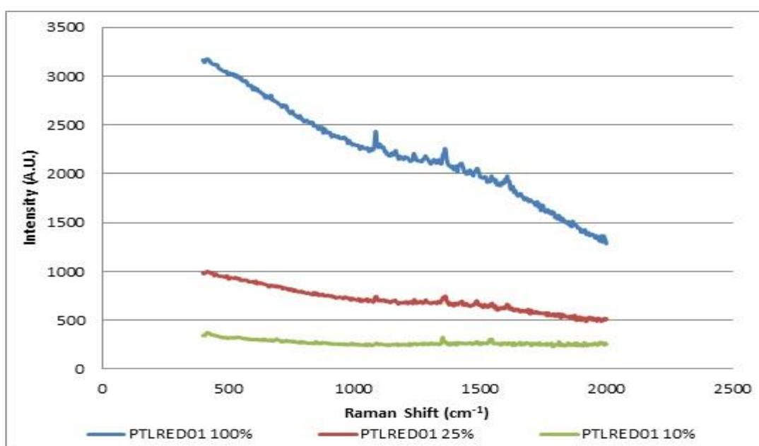
Figure 6.17: Example spectra of a PTL UK red gel ink line on office paper (FORAM 785 varied laser power/x 20 obj., 1.0s default scan time)
