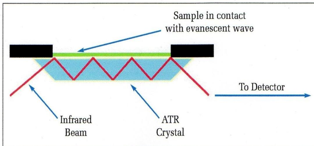
Figure 1.14: ATR sample interface schematic diagram (reproduced from [144])
