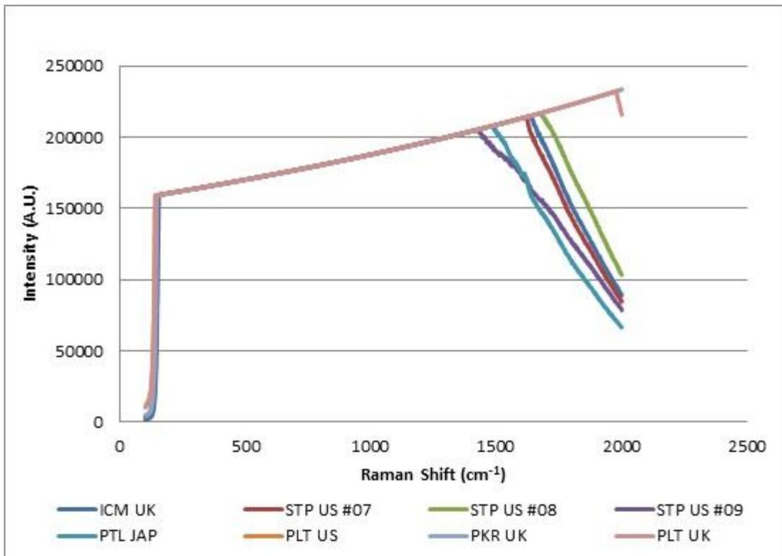
Figure 6.59: Brand/model combinations of blue gel ink forming Group 6 (Renishaw InVia 830 nm 10% laser power/x 50 obj.)
