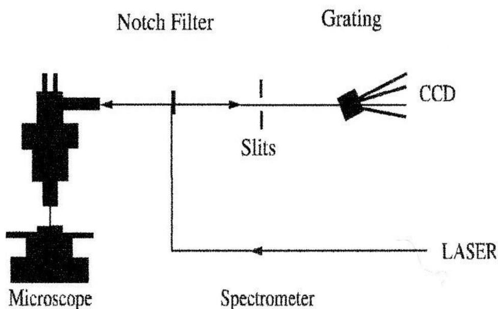
Figure 1.15: Schematic diagram of a Raman Microscope Spectrometer system (reproduced from [147])
