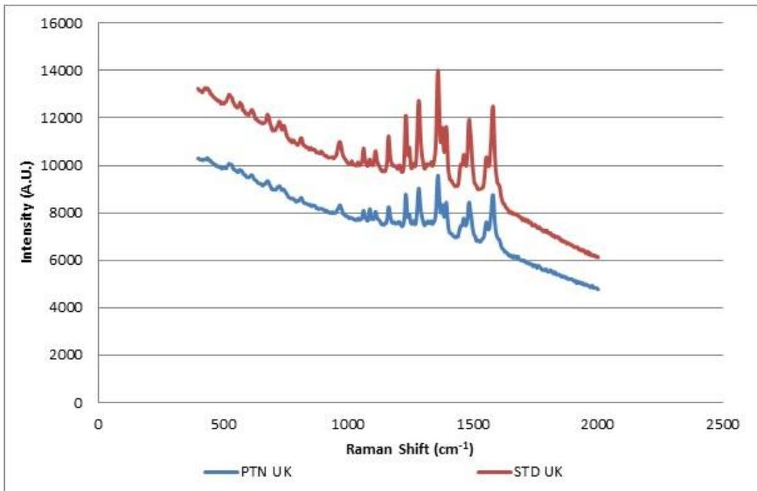
Figure 6.73: Brand/model combinations of red gel ink forming Group 4 (FORAM 785 100% laser power/x 50 obj., Auto Exposure)
