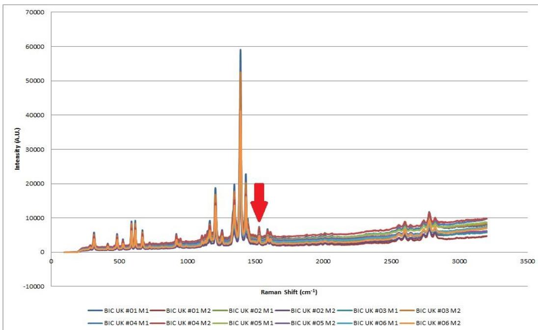
Figure 6.61: Example of a brand/model combination (BIC UK) in Group 2a exhibiting a reproducible spectral pattern with an obvious peak at  $\sim 1550\text{ cm}^{-1}$  highlighted by the red arrow (Renishaw InVia 514.5 nm 10% laser power/x 20 obj.)
