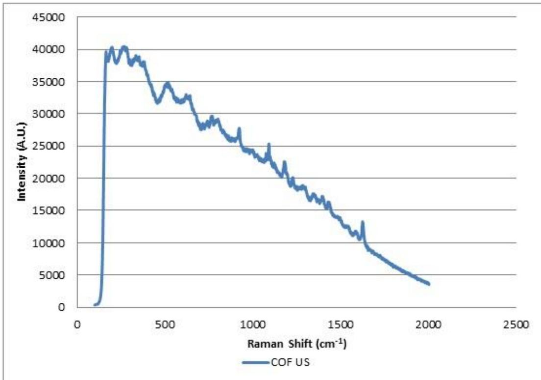
Figure 6.58: Brand/model combinations of blue gel ink forming Group 5 (Renishaw InVia 830 nm 10% laser power/x 50 obj.)
