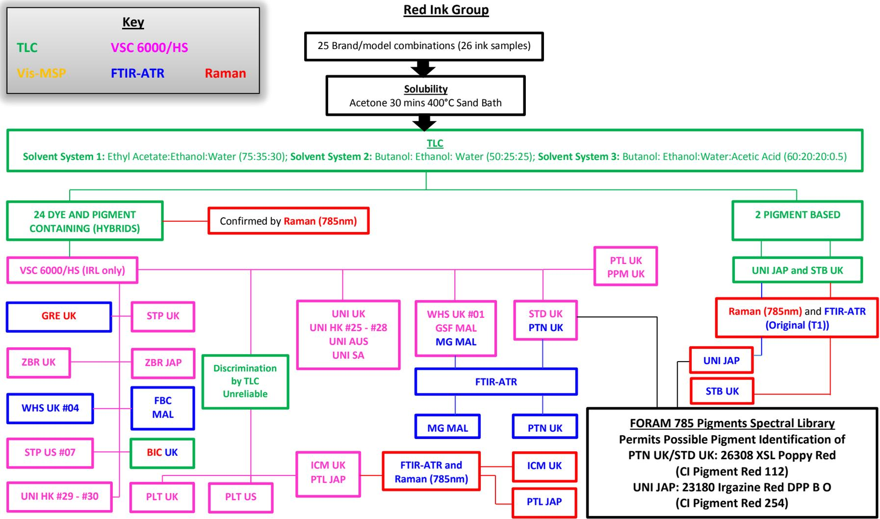
FIGURE 8.2: BETWEEN 10 – 14 GROUPS IDENTIFIED BY FTIR-ATR AND RAMAN SPECTROSCOPY (785 nm) DEPENDENT UPON TECHNIQUE
