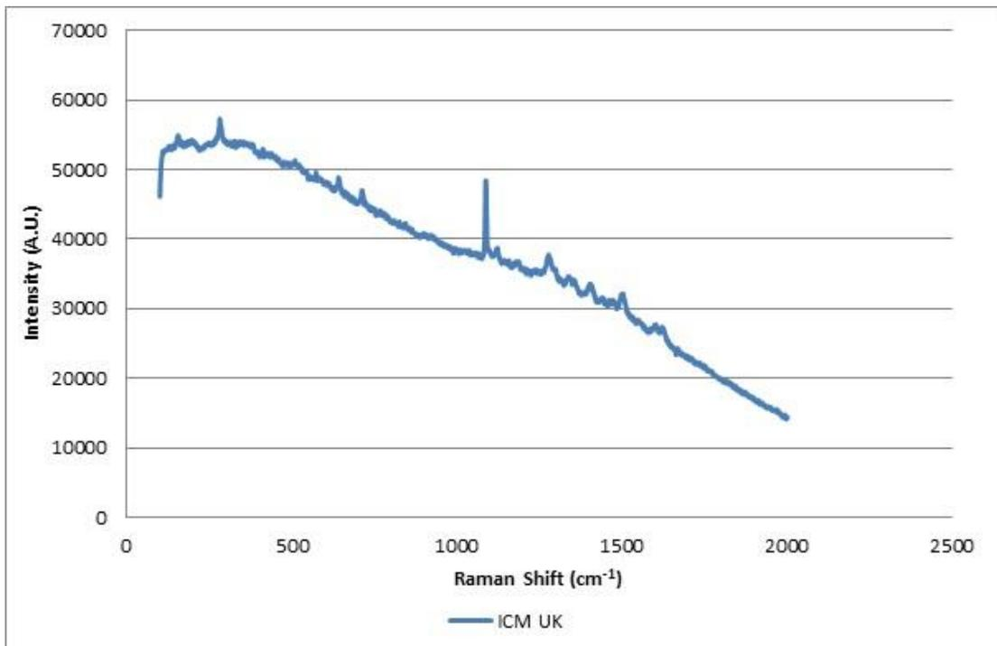
Figure 6.89: Brand/model combination of red gel ink forming Group 10 (Renishaw InVia 785 nm 100% laser power/x 50 obj.)
