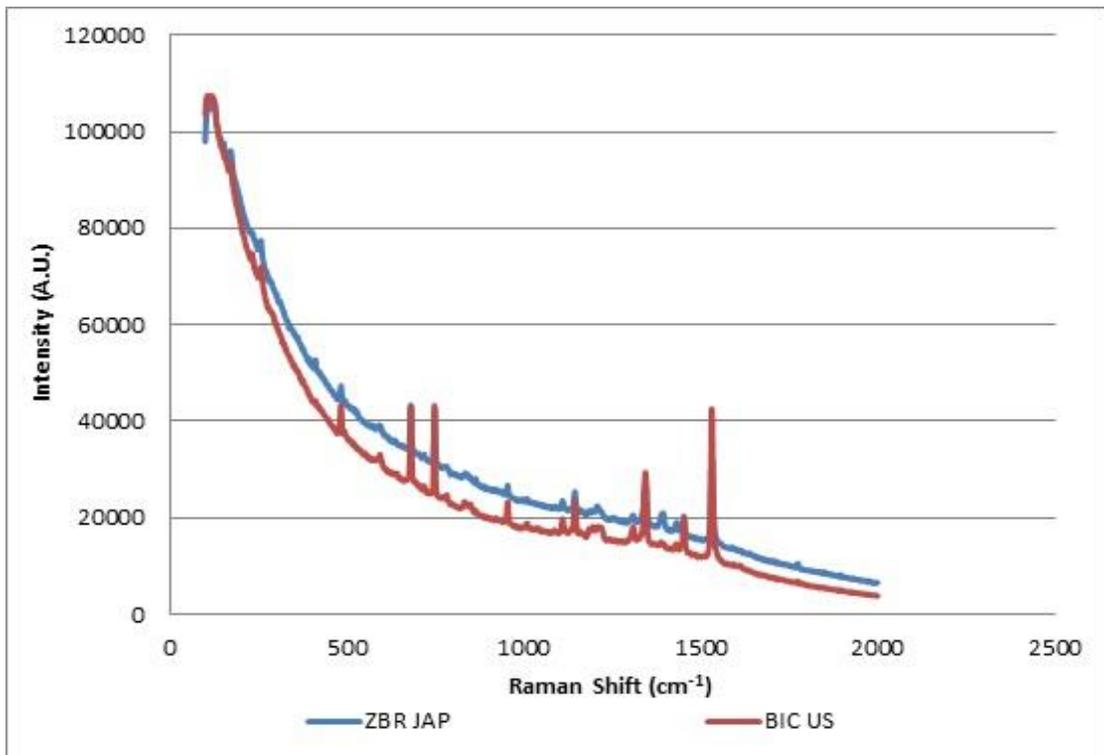
Figure 6.47: INTL brand/model combinations of blue gel ink forming Group 2 (Renishaw InVia 785 nm 10% laser power/x 50 obj.)
