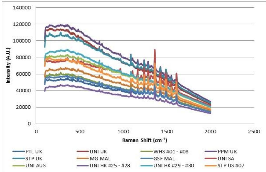
Figure 6.80: Brand/model combinations of red gel ink forming Group 1 (Renishaw InVia 785 nm 100% laser power/x 50 obj.)
