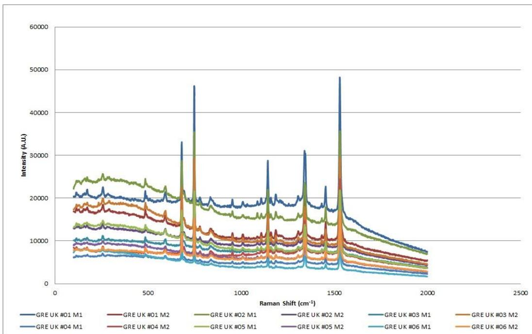
Figure 6.37: Set of 12 spectra from GRE UK blue gel ink illustrating good reproducibility with only minor spectral variation due to S:N ratio (Renishaw InVia 785 nm 10% laser power/x 50 obj.)
