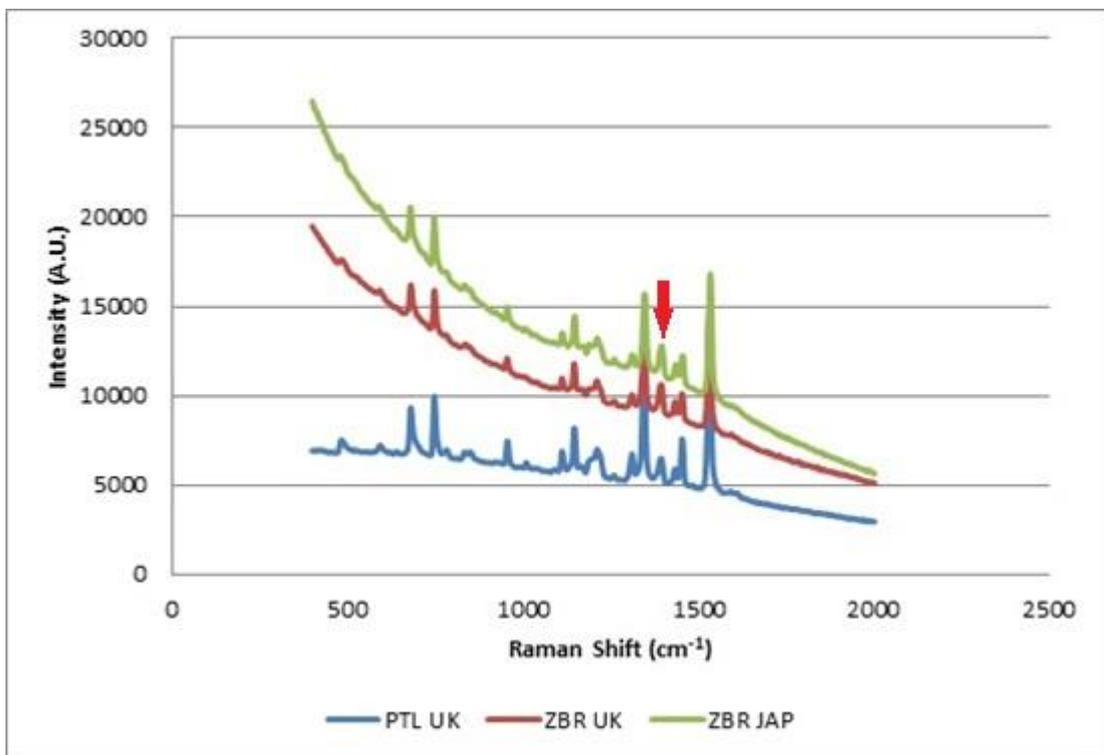
Figure 6.64: Brand/model combinations of blue gel ink forming Group 2b based on relative peak intensity at  $\sim 1390\text{ cm}^{-1}$  highlighted by the red arrow (FORAM 785 100% laser power/x 50 obj., Auto Exposure)
