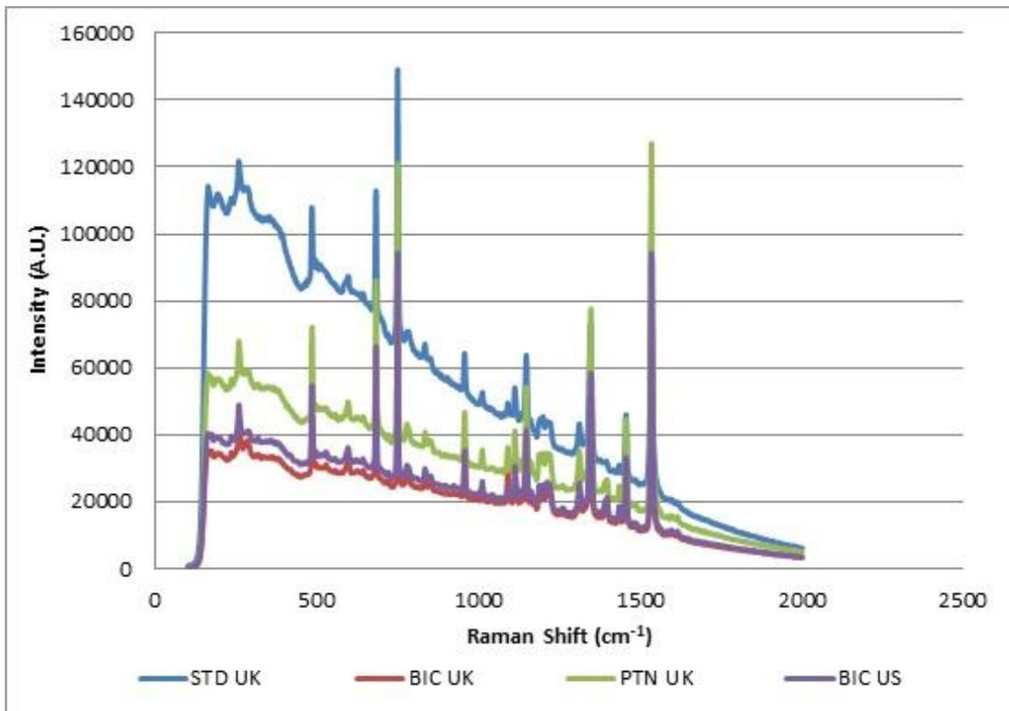
Figure 6.55: Brand/model combinations of blue gel ink forming Group 2 (Renishaw InVia 830 nm 10% laser power/x 50 obj.)
