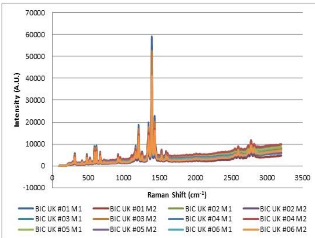
Figure 6.24: Comparison of duplicate spectra from six BIC UK blue gel ink pen lines on paper demonstrating good reproducibility and strong Raman signals (Renishaw InVia 514.5 nm 10% laser power/x 20 obj.)
