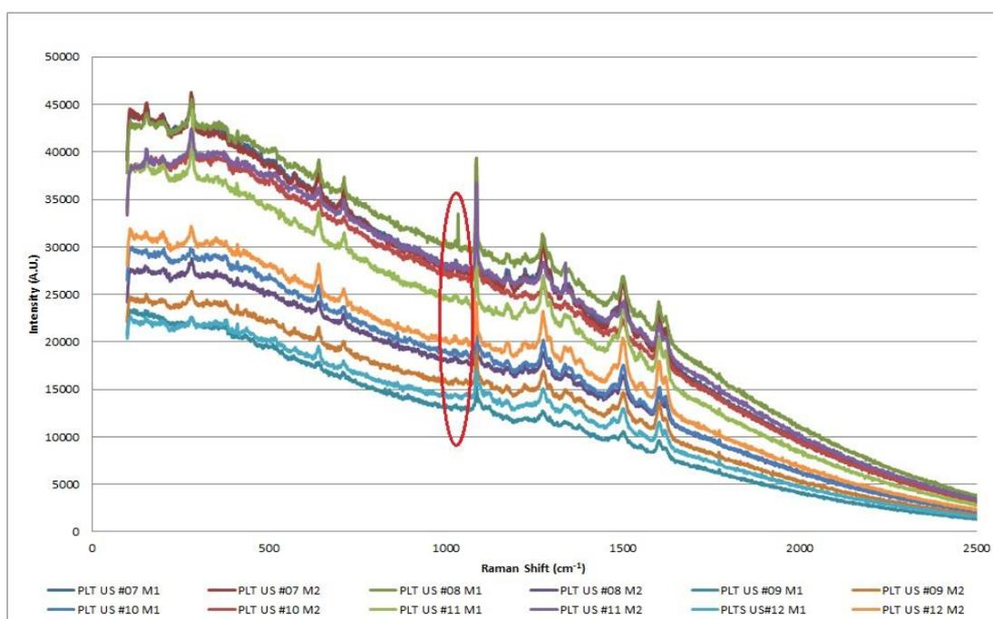
Figure 6.99: Spectra of PLT US pens #07 - #12 red gel ink on paper exhibiting a stray peak at  $\sim 1035\text{ cm}^{-1}$  highlighted in the red circle (Renishaw InVia 785 nm 100% laser power/x 50 obj.)
