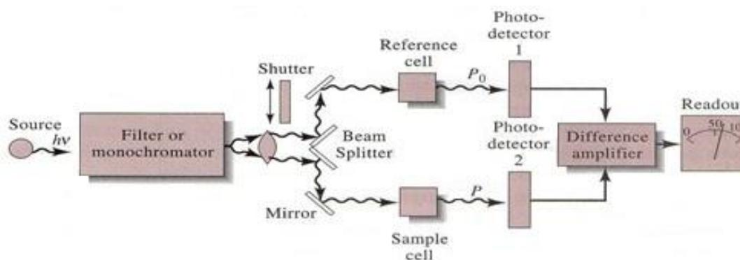
Figure 1.12: Double beam dispersive IR Spectrometer schematic diagram (reproduced from [138])
