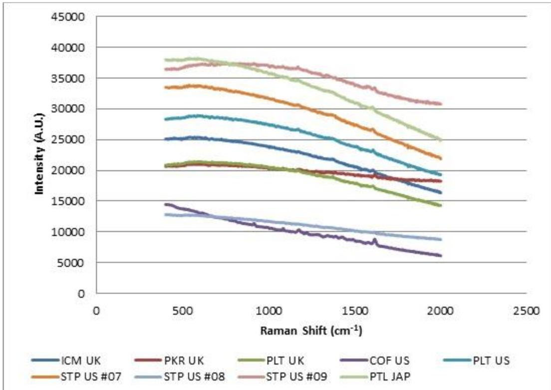
Figure 6.44: Brand/model combinations of blue gel ink forming Group 4 (FORAM 785 100% laser power/x 50 obj., Auto Exposure)
