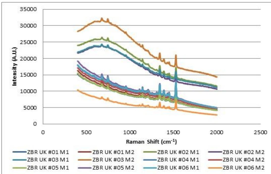
Figure 6.19: Duplicate spectra taken from each of blue ZBR UK pens #01 - #06 on paper demonstrating reproducible differences in background fluorescence shape suggestive of within brand variation (FORAM 785 100% laser power/x 20 obj., Auto Exposure)
