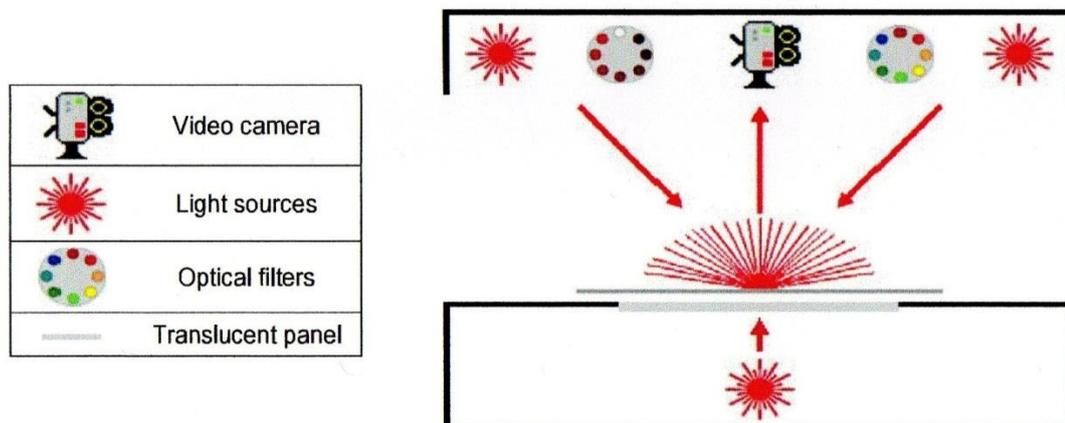
Figure 3.4: Basic hardware component set up inside the VSC 6000/HS [161, 162]
