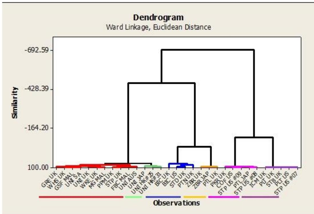
Figure 7.32: HCA dendrogram of blue ink group samples analysed by FTIR-ATR presented in a 32 BIN data matrix format reflecting T2 level visual pattern recognition groups. HCA resulted in successful discrimination into six clusters in line with T2 level visual discrimination when using a combination of Ward Linkage and Euclidean Distance
