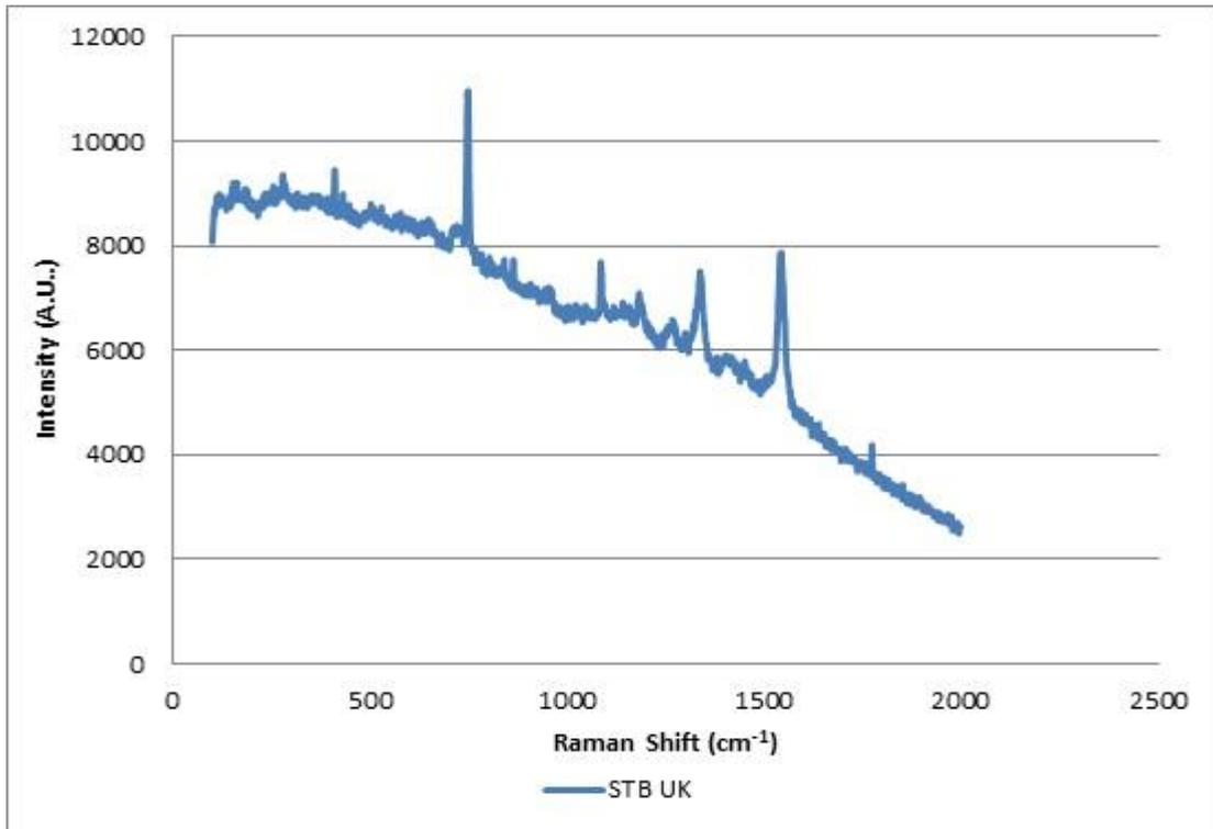
Figure 6.49: UK brand/model combinations of blue gel ink forming Group 3 (Renishaw InVia 785 nm 10% laser power/x 50 obj.)
