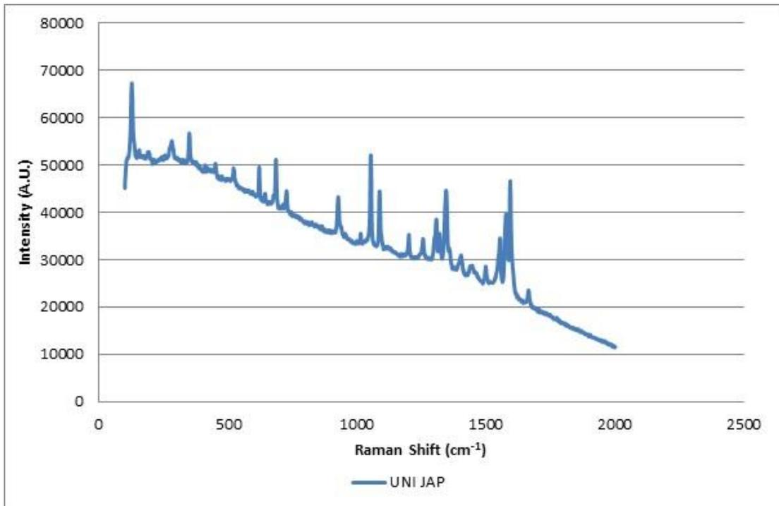
Figure 6.88: Brand/model combination of red gel ink forming Group 9 (Renishaw InVia 785 nm 100% laser power/x 50 obj.)
