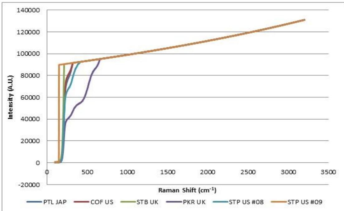
Figure 6.30: Brand/model combinations of blue gel ink forming Group 6 (Renishaw InVia 514.5 nm 10% laser power/x 20 obj.)
