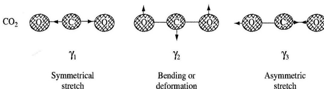
Figure 1.7: Stretching of chemical bonds in a carbon dioxide molecule (reproduced from [137])
