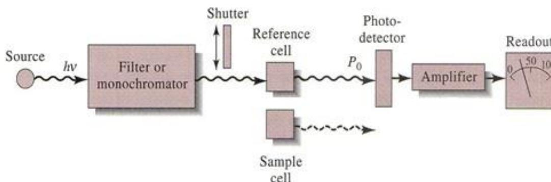
Figure 1.11: Single beam dispersive IR Spectrometer schematic diagram (reproduced from [138])
