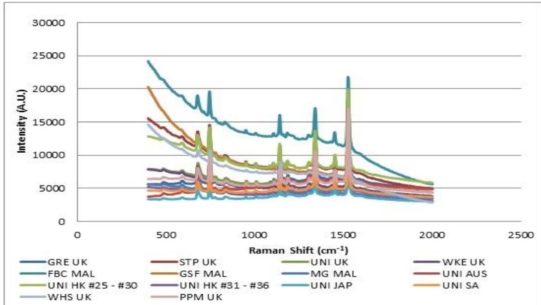
Figure 6.41: Brand/model combinations of blue gel ink forming Group 1 (FORAM 785 100% laser power/x 50 obj., Auto Exposure)
