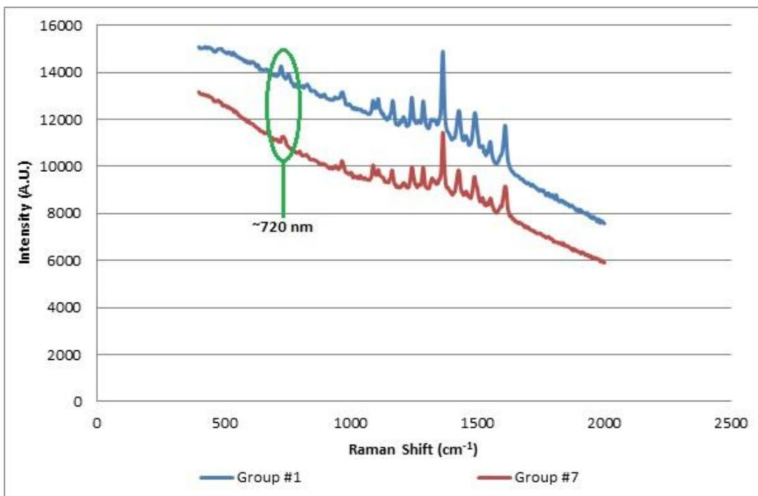
Figure 6.90: Highly similar spectral pattern representing Group 1 and Group 7 red gel ink brand/model combinations distinguishable by an additional peak at ~720 nm observed in Group 1 spectra (FORAM 785 100% laser power/x 50 obj., Auto Exposure)
