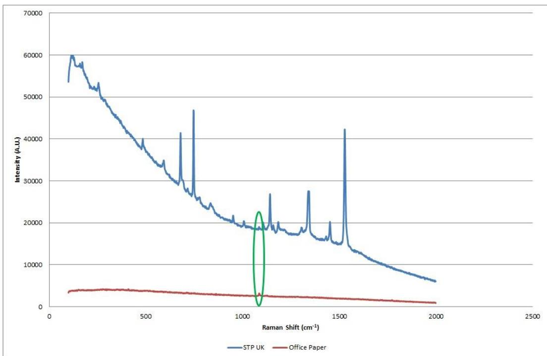
Figure 6.40: An example spectrum of STP UK blue gel ink on paper compared to a spectrum of the un-inked paper illustrating minimal spectral interference from the paper substrate except for a minor peak at  $\sim 1094 \text{ cm}^{-1}$  highlighted within the green circle (Renishaw InVia 785 nm 10% laser power/x 50 obj.)
