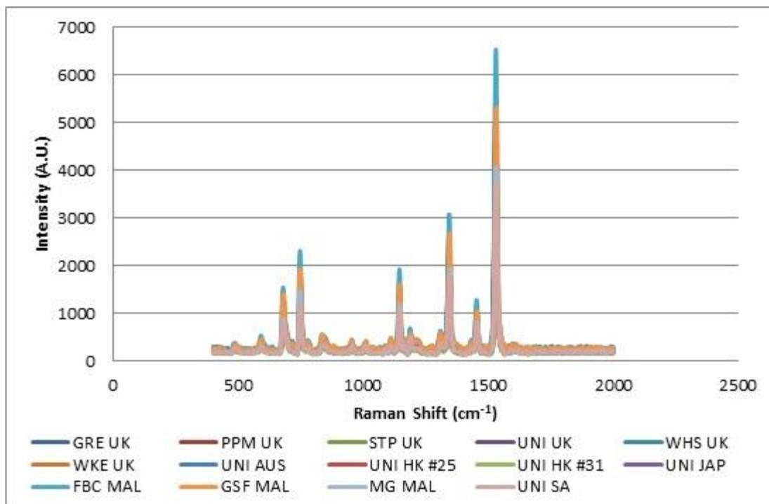
Figure 6.60: Brand/model combinations of blue gel ink forming Group 1 showing an indistinguishable spectral pattern after baseline correction and smoothing applied (FORAM 785 100% laser power/x 20 obj., 1.0s default scan time)
