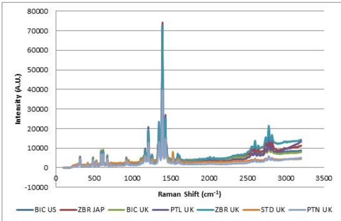
Figure 6.26: Brand/model combinations of blue gel ink forming Group 2 (Renishaw InVia 514.5 nm 10% laser power/x 20 obj.)
