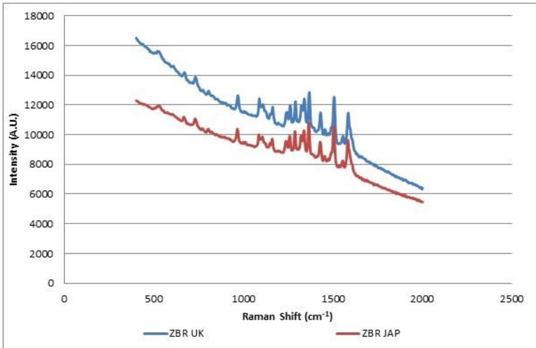
Figure 6.74: Brand/model combinations of red gel ink forming Group 5 (FORAM 785 100% laser power/x 50 obj., Auto Exposure)
