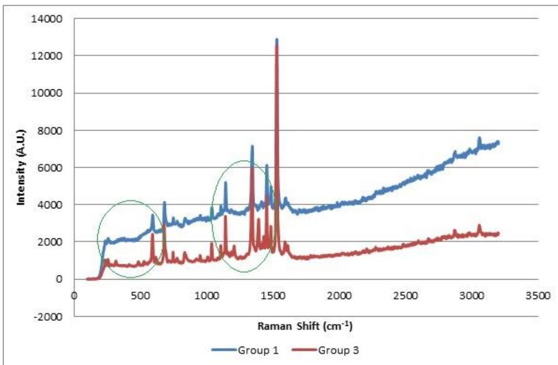
Figure 6.31: Comparison of Group 1 and Group 3 spectra for blue gel ink samples, spectral differences highlighted within green circles (Renishaw InVia 514.5 nm 10% laser power/x 20 obj.)
