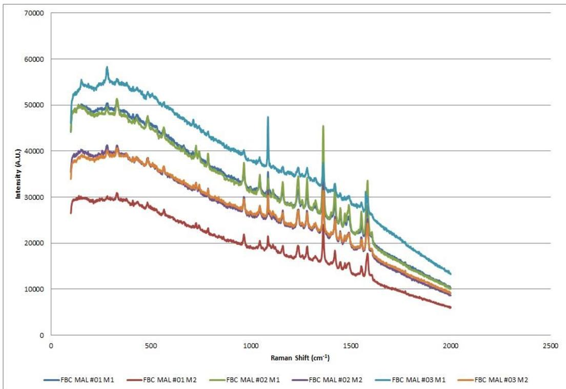
Figure 6.97: Duplicate spectra of FBC MAL pens #01 - #03 red gel ink on paper (Renishaw InVia 785 nm 100% laser power/x 50 obj.)
