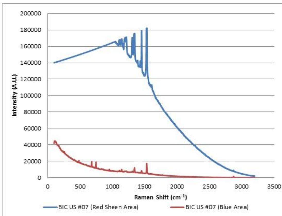
Figure 6.65: Spectra of BIC US blue gel ink on paper illustrating an excessive spectral intensity from the red sheen area of the blue ink line (Renishaw InVia 785 nm 100% laser power/x 50 obj.)
