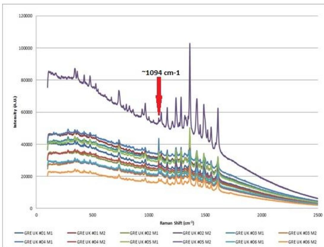
Figure 6.67: Spectra of GRE UK pens #01 – #06 red gel ink on paper demonstrating strong signal intensity and good reproducibility (Renishaw InVia 785 nm 100% laser power/x 50 obj.). A peak attributable to the paper substrate at  $\sim 1094\text{ cm}^{-1}$  highlighted by the red arrow
