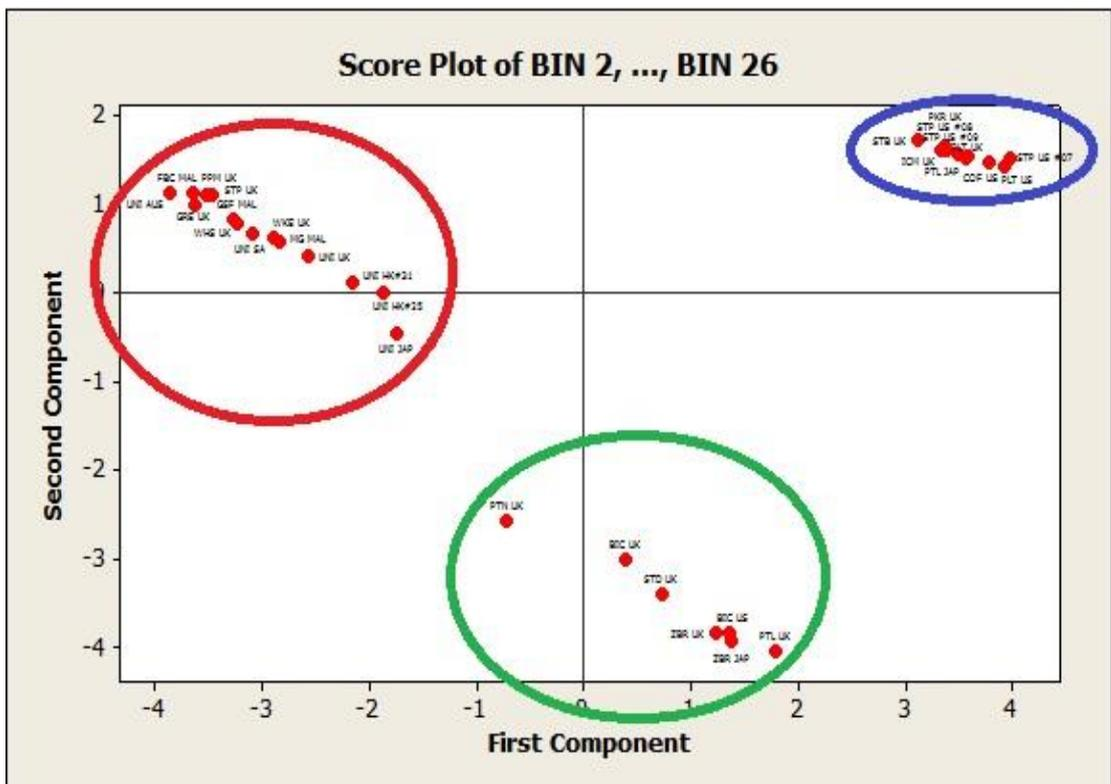
Figure 7.22: PCA score plot of blue ink group samples analysed by FTIR-ATR presented in a 32 BIN data matrix format demonstrating three clearly well resolved clusters in line with T1 level visual pattern recognition groups
