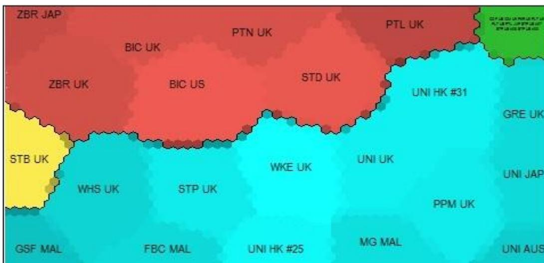
Figure 7.9: SOFM of blue ink group samples analysed by FORAM 785 demonstrating successful discrimination into four clusters, with variations in colour hue within the blue and red clusters highlighting subtle differences in combined relative peak intensities associated with the wavenumbers characterising the ink samples within the two spectral groups
