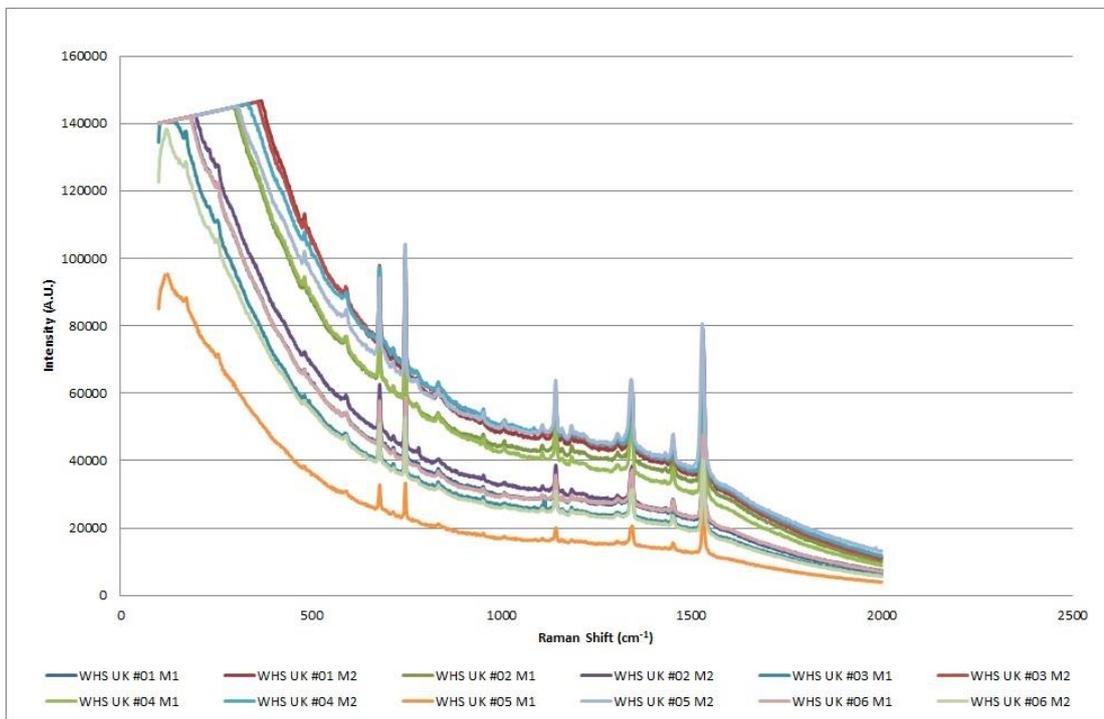
Figure 6.39: Set of 12 spectra from WHS UK blue gel ink illustrating partial detector overload in several measurements (Renishaw InVia 785 nm 10% laser power/x 50 obj.)
