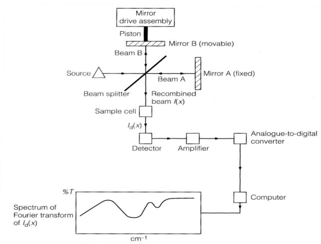
Figure 1.13: Schematic diagram of the components of an FTIR Spectrometer (reproduced from [141])
