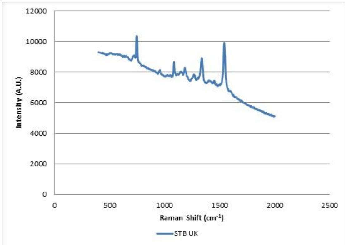
Figure 6.43: Brand/model combinations of blue gel ink forming Group 3 (FORAM 785 100% laser power/x 50 obj., Auto Exposure)
