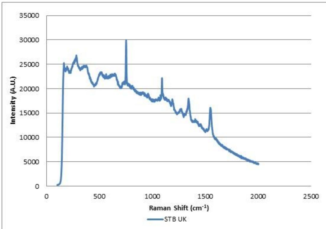
Figure 6.57: Brand/model combinations of blue gel ink forming Group 4 (Renishaw InVia 830 nm 10% laser power/x 50 obj.)
