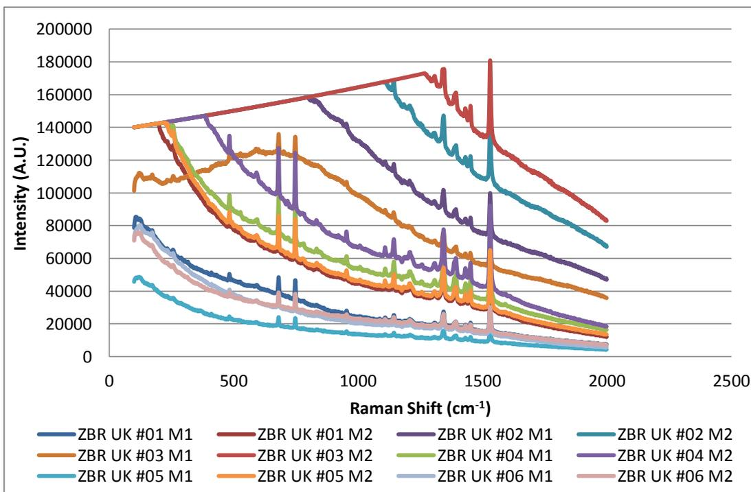
Figure 6.20: Duplicate spectra from each of blue ZBR UK pens #01 – 06 demonstrating some evidence of within brand variation (Renishaw InVia 785 nm 10% laser power/x 50 obj.)
