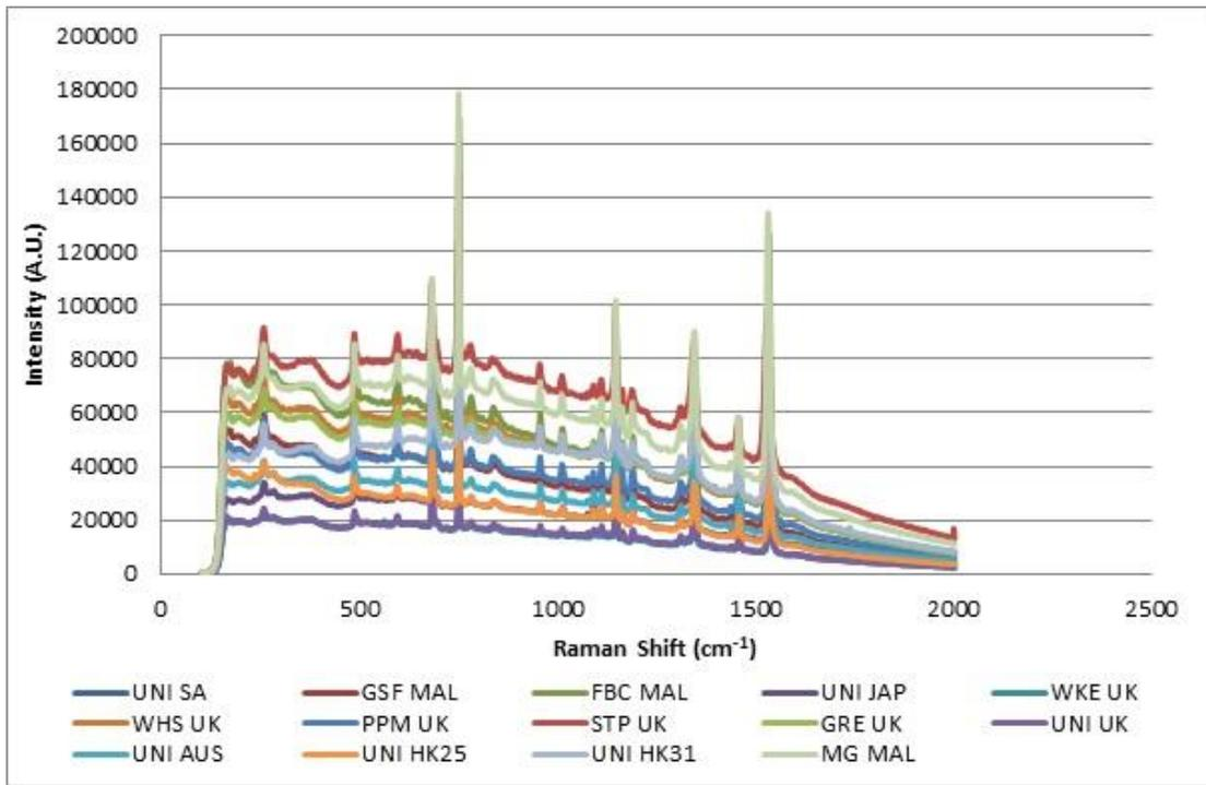
Figure 6.54: Brand/model combinations of blue gel ink forming Group 1 (Renishaw InVia 830 nm 10% laser power/x 50 obj.)
