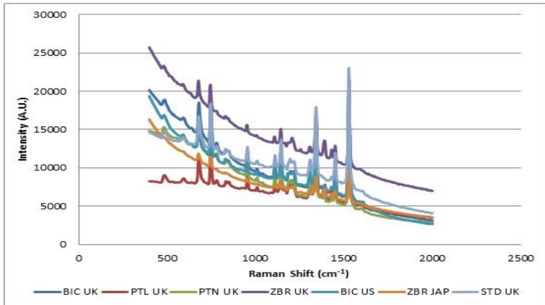
Figure 6.42: Brand/model combinations of blue gel ink forming Group 2 (FORAM 785 100% laser power/x 50 obj., Auto Exposure)
