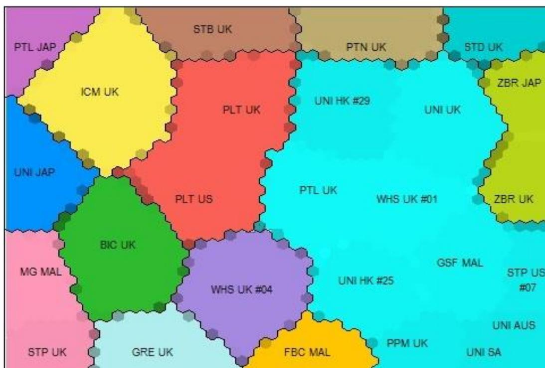
Figure 7.39: SOFM of red ink group samples analysed by FTIR-ATR demonstrating successful discrimination into 14 clusters in line with T1 level visual pattern recognition groups. Minimal variation in colour hue within a cluster containing multiple ink samples demonstrates a high degree of similarity between samples within that cluster
