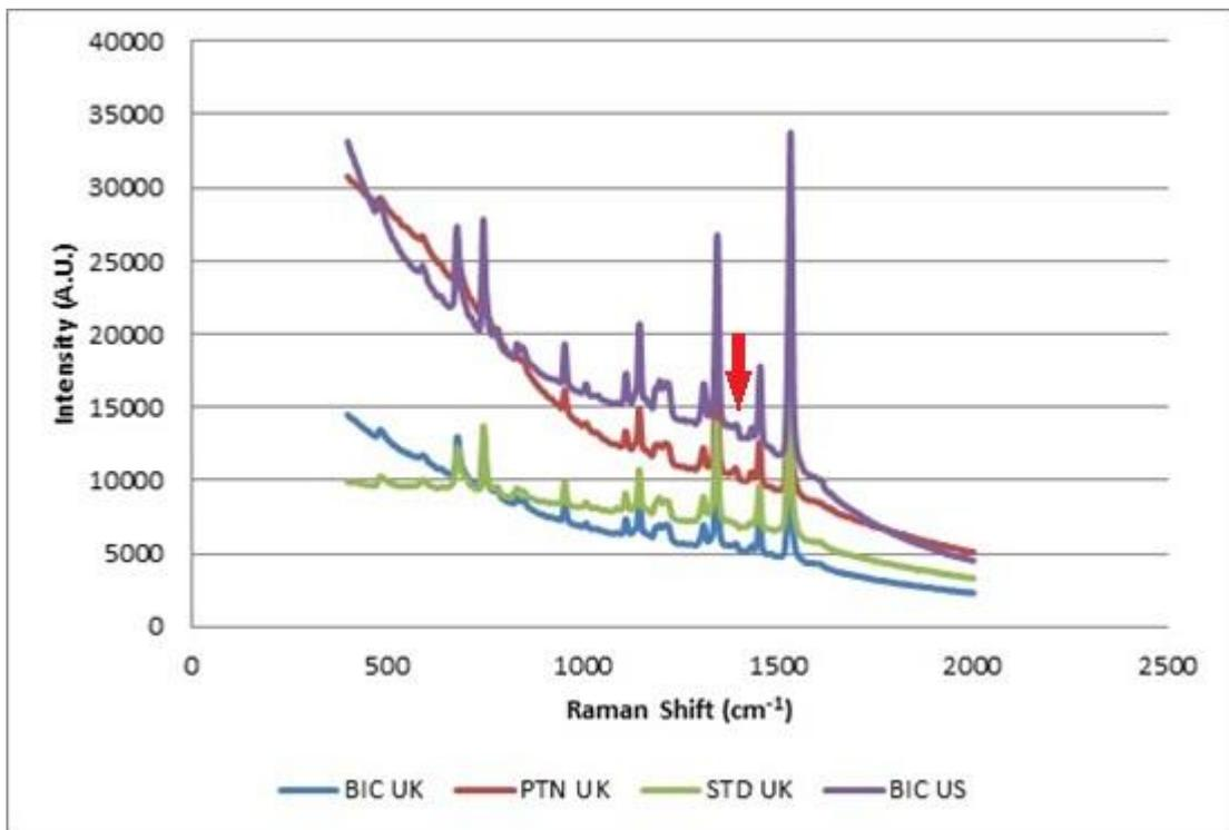
Figure 6.63: Brand/model combinations of blue gel ink forming Group 2a based on relative peak intensity at  $\sim 1390\text{ cm}^{-1}$  highlighted by the red arrow (FORAM 785 100% laser power/x 50 obj., Auto Exposure)
