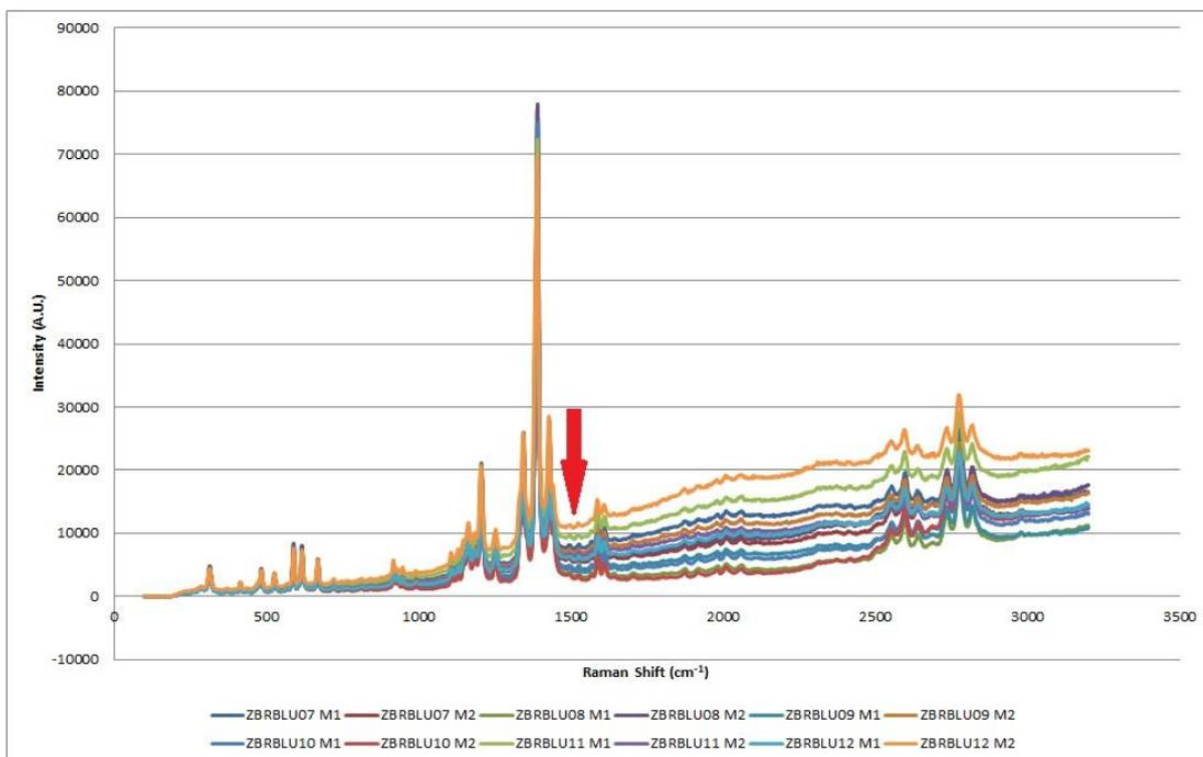
Figure 6.62: Example of a brand/model combination (ZBR JAP) in Group 2b exhibiting a reproducible spectral pattern without an obvious peak at  $\sim 1550\text{ cm}^{-1}$  highlighted by the red arrow (Renishaw InVia 514.5 nm 10% laser power/x 20 obj.)
