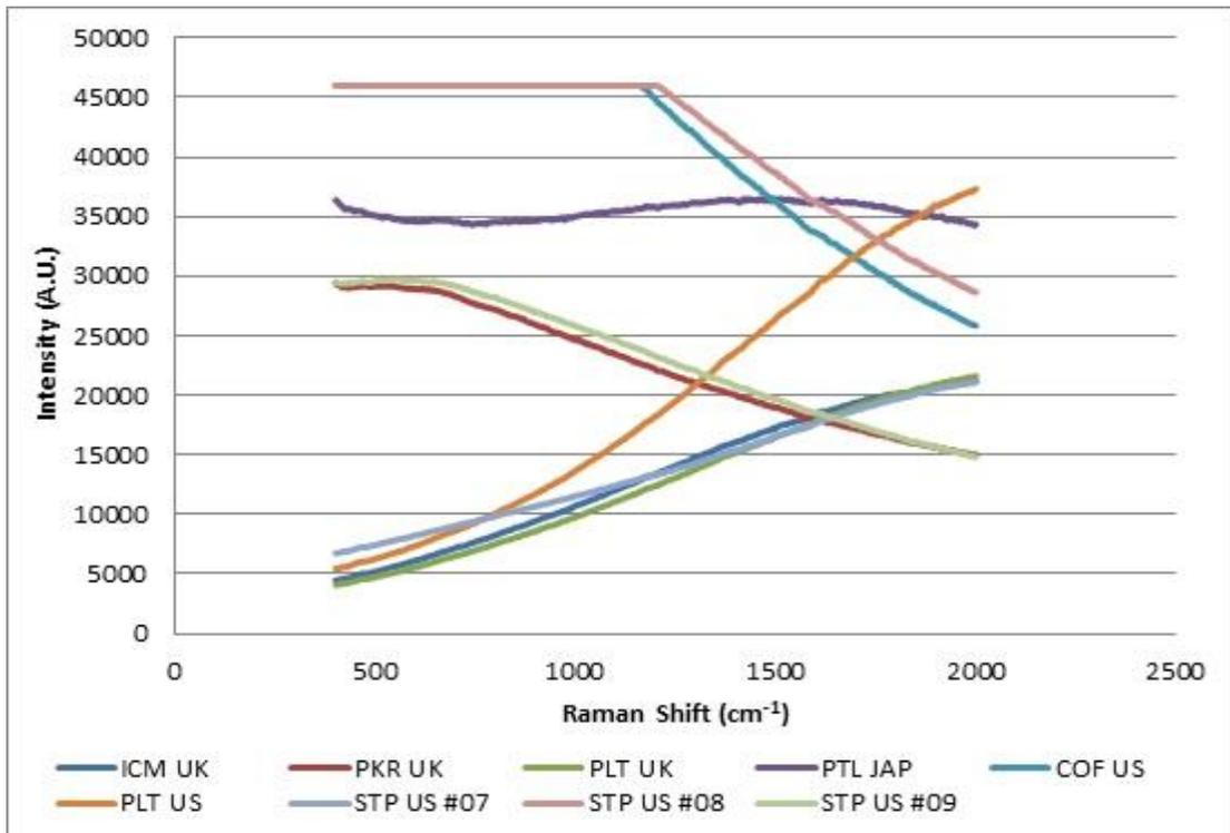
Figure 6.36: Brand/model combinations of blue gel ink forming Group 4 (FORAM 685-2 10% laser power/x 20 obj., Auto Exposure)
