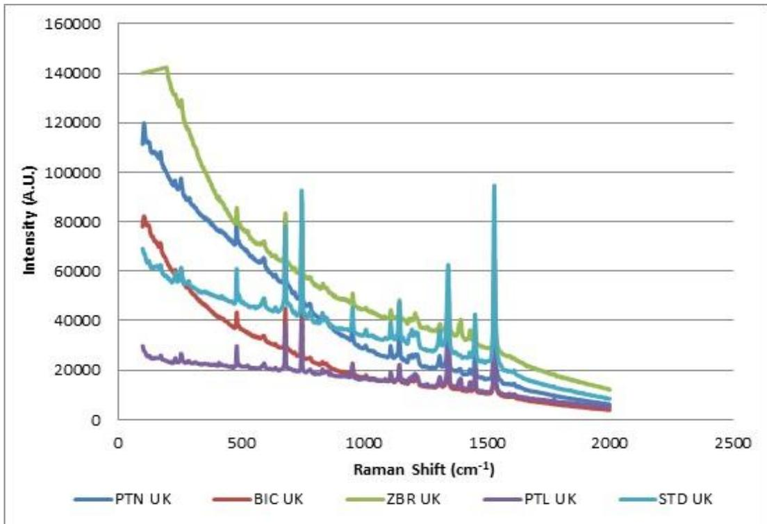
Figure 6.48: UK brand/model combinations of blue gel ink forming Group 2 (Renishaw InVia 785 nm 10% laser power/x 50 obj.)
