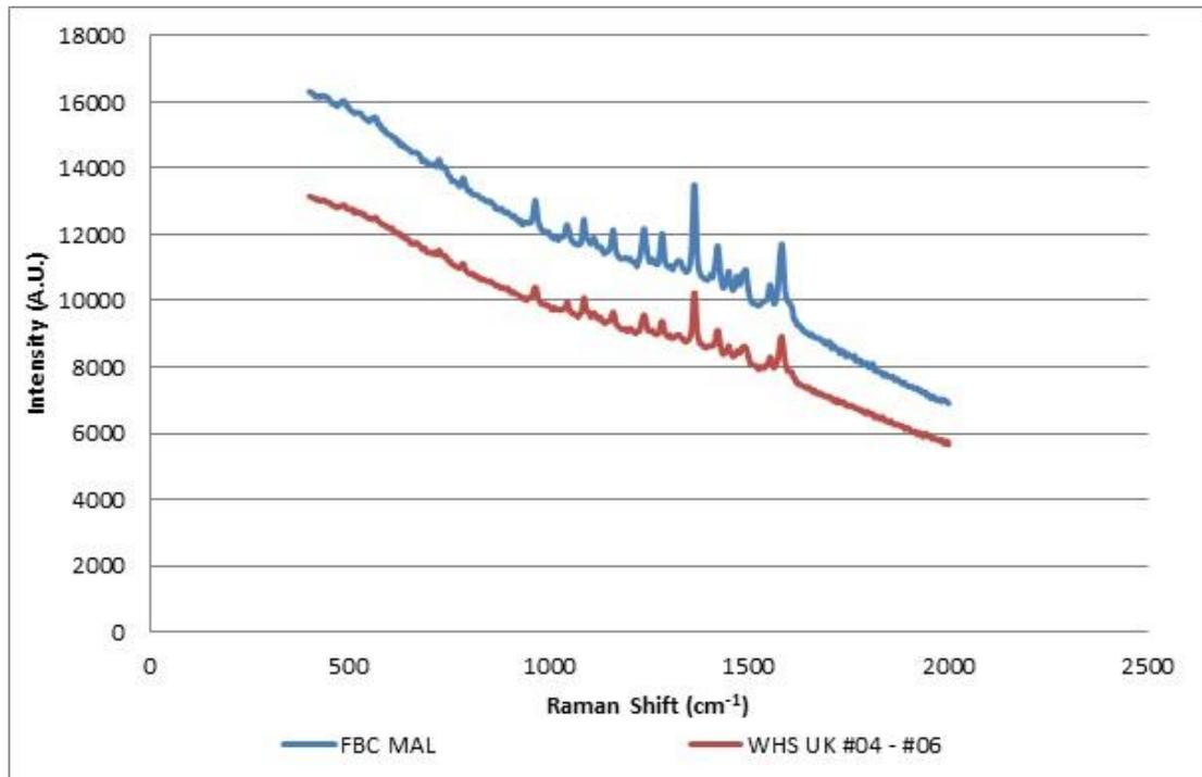
Figure 6.71: Brand/model combinations of red gel ink forming Group 2 (FORAM 785 100% laser power/x 50 obj., Auto Exposure)
