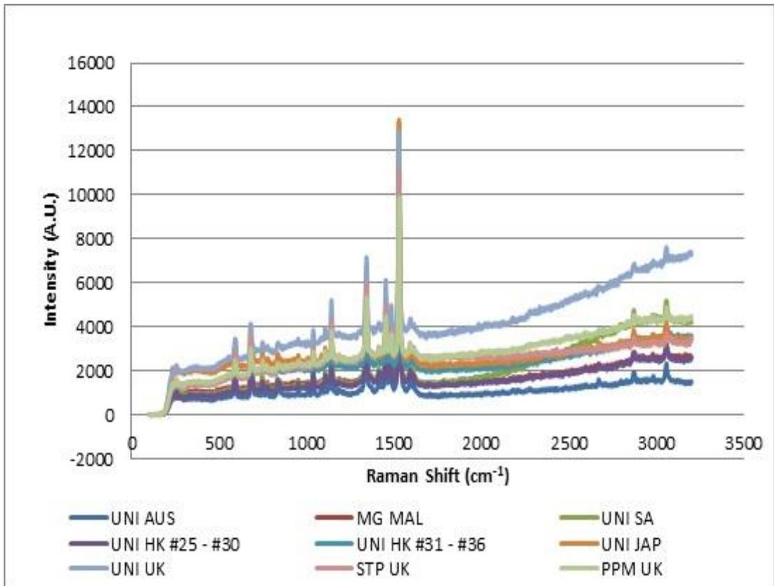
Figure 6.25: Brand/model combinations of blue gel ink forming Group 1 (Renishaw InVia 514.5 nm 10% laser power/x 20 obj.)
