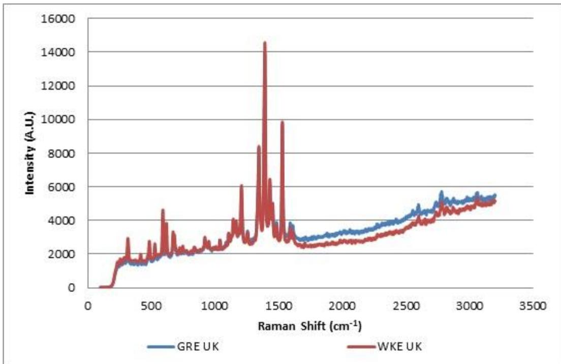
Figure 6.28: Brand/model combinations of blue gel ink forming Group 4 (Renishaw InVia 514.5 nm 10% laser power/x 20 obj.)
