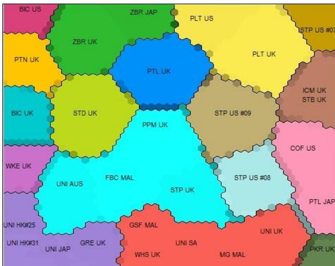
Figure 7.25: SOFM of blue ink group samples analysed by FTIR-ATR presented in a 32 BIN data matrix format reflecting T4 level visual pattern recognition groups. SOFM resulted in misclassification of samples inconsistent with the expected 17 clusters distinguished by visual pattern recognition
