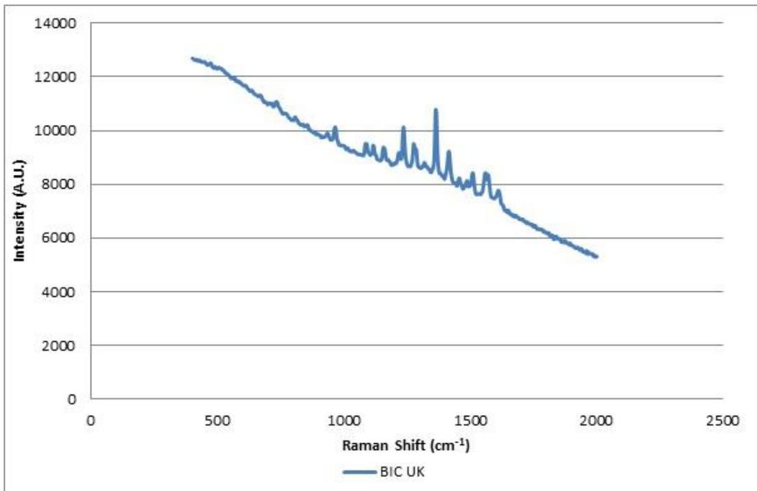
Figure 6.75: Brand/model combination of red gel ink forming Group 6 (FORAM 785 100% laser power/x 50 obj., Auto Exposure)
