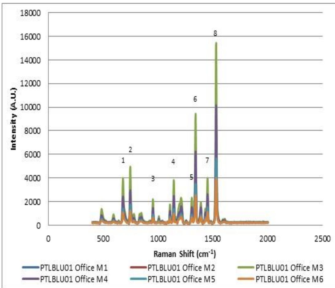
Figure 6.18: Eight randomly selected peaks used to calculate % RSD for validation to analyse blue gel ink lines on office paper (FORAM 785 100% laser power/x 20 obj., 1.0s default scan time, baseline corrected and smoothed)
