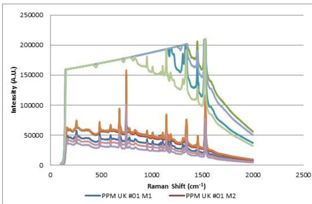
Figure 6.53: Example of a spectrum exhibiting detector overload and/or an unusually high spectral intensity in comparison to other spectra for the blue PPM UK brand/model combination (Renishaw InVia 830 nm 10% laser power/x 50 obj.)
