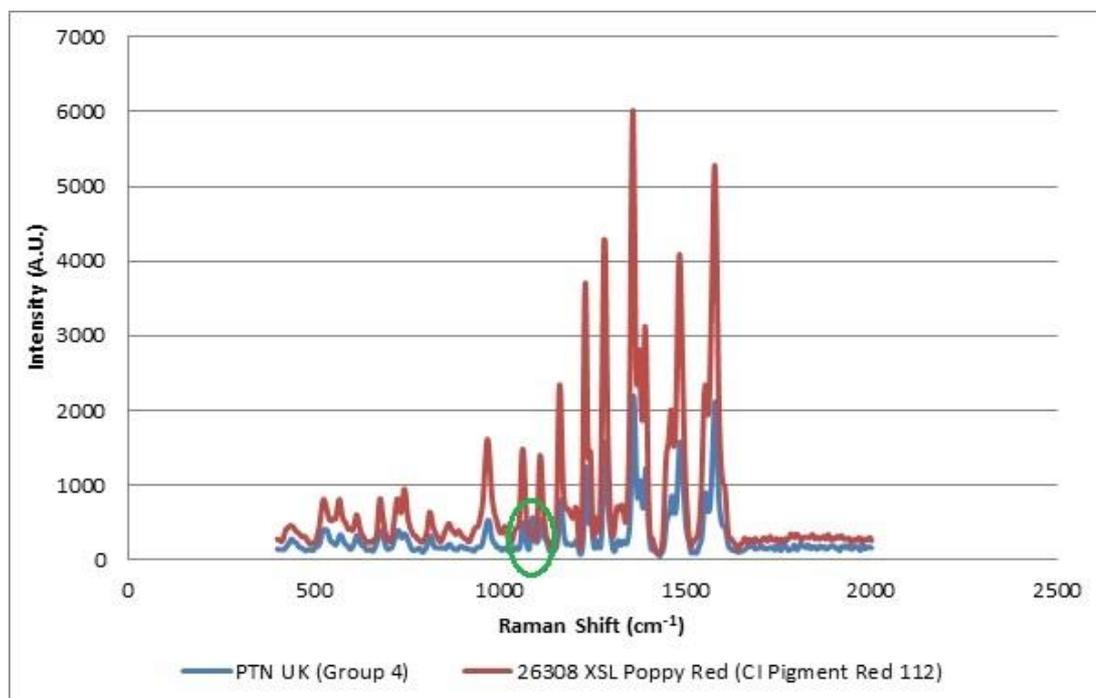
Figure 6.102: Red Ink Group 4, suggested pigment identification of XSL Poppy Red (CI Pigment Red 112) (FORAM 785). A peak at  $\sim 1094\text{ cm}^{-1}$  attributable to the paper substrate and observed in the ink spectrum, but not the pigment spectrum is highlighted within the green circle.
