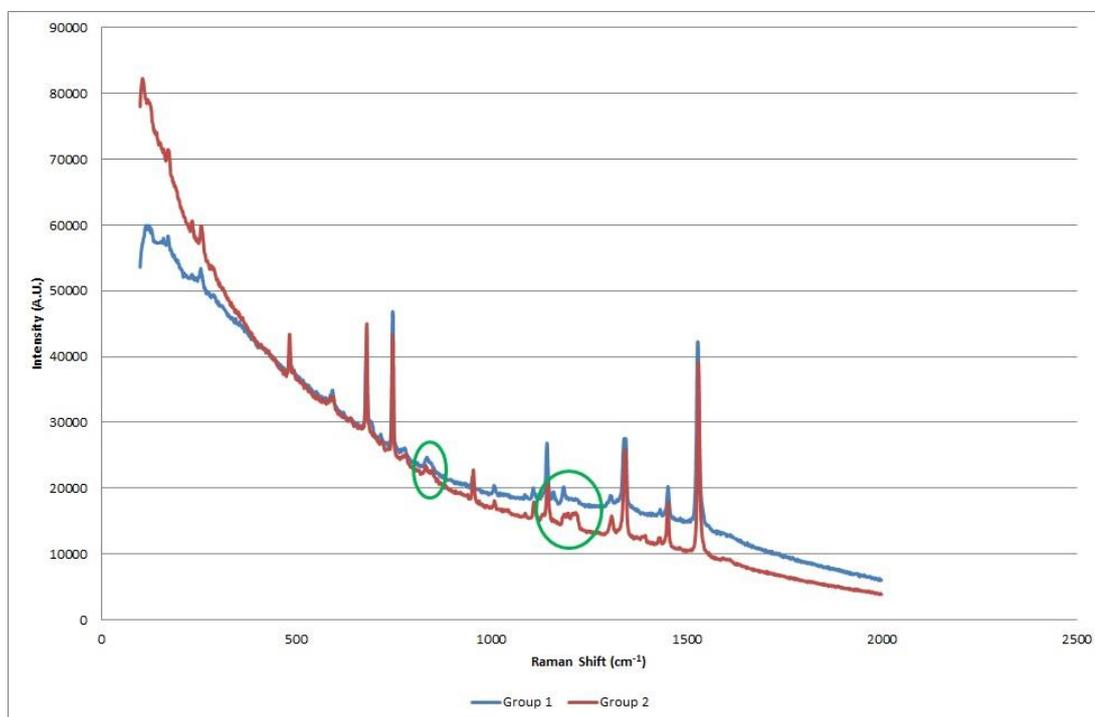
Figure 6.52: Example spectra representing Group 1 and Group 2 highlighting (within the green circles) subtle spectral variations permitting discrimination between the two (Renishaw InVia 785 nm 10% laser power/x 50 obj.)
