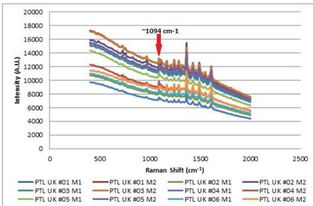
Figure 6.66: Spectra from PTL UK red gel ink on paper demonstrating good reproducibility but some peak intensity variation (FORAM 785 100% laser power/x 50 obj., Auto Exposure). A peak attributable to the paper substrate at  $\sim 1094\text{ cm}^{-1}$  highlighted by the red arrow
