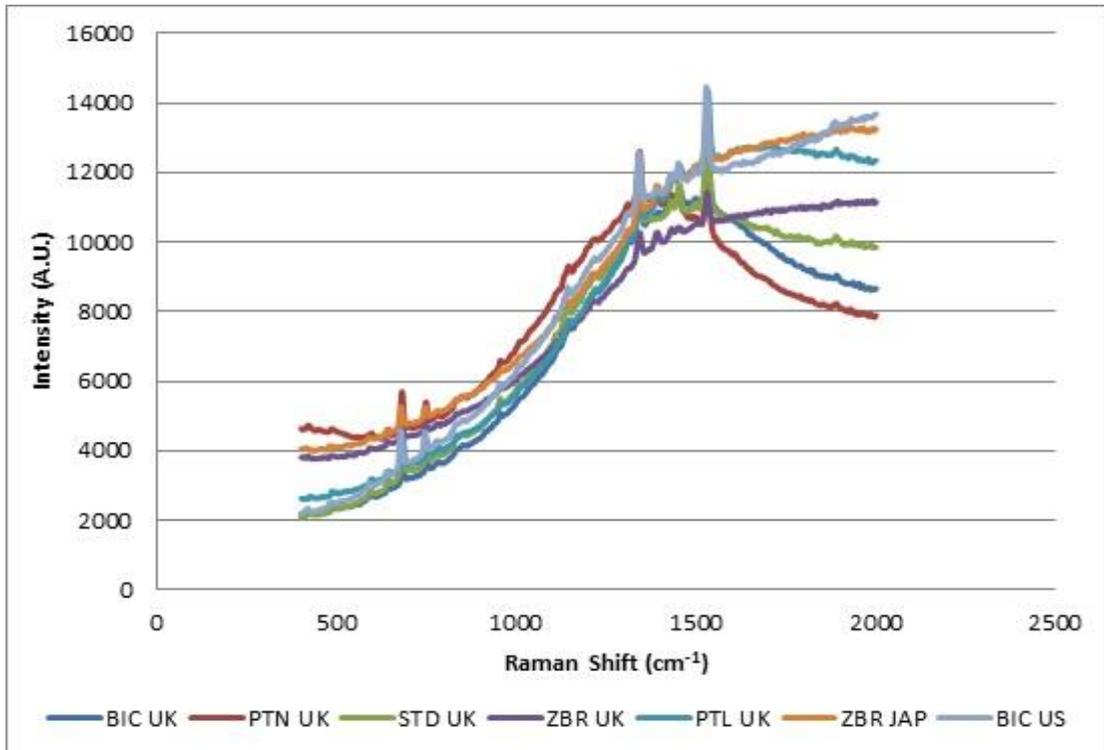
Figure 6.34: Brand/model combinations of blue gel ink forming Group 2 (FORAM 685-2 10% laser power/x 20 obj., Auto Exposure)
