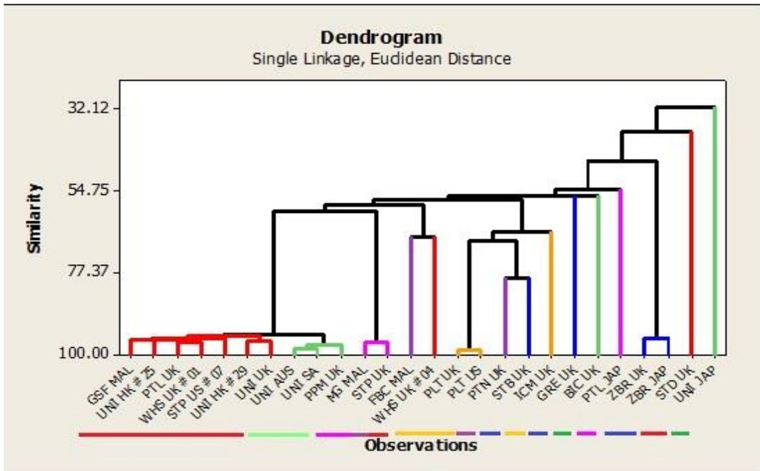
Figure 7.37: HCA dendrogram of red ink group samples analysed by FTIR-ATR demonstrating discrimination into 15 clusters. The expected discrimination between STP UK and MG MAL samples is not observed, instead sub-division of the largest group (n = 10) occurs. This demonstrates inconsistency between multivariate profiling and visual pattern recognition observations suggesting relative peak intensity differences used to discriminate the STP UK and MG MAL samples could not be validated
