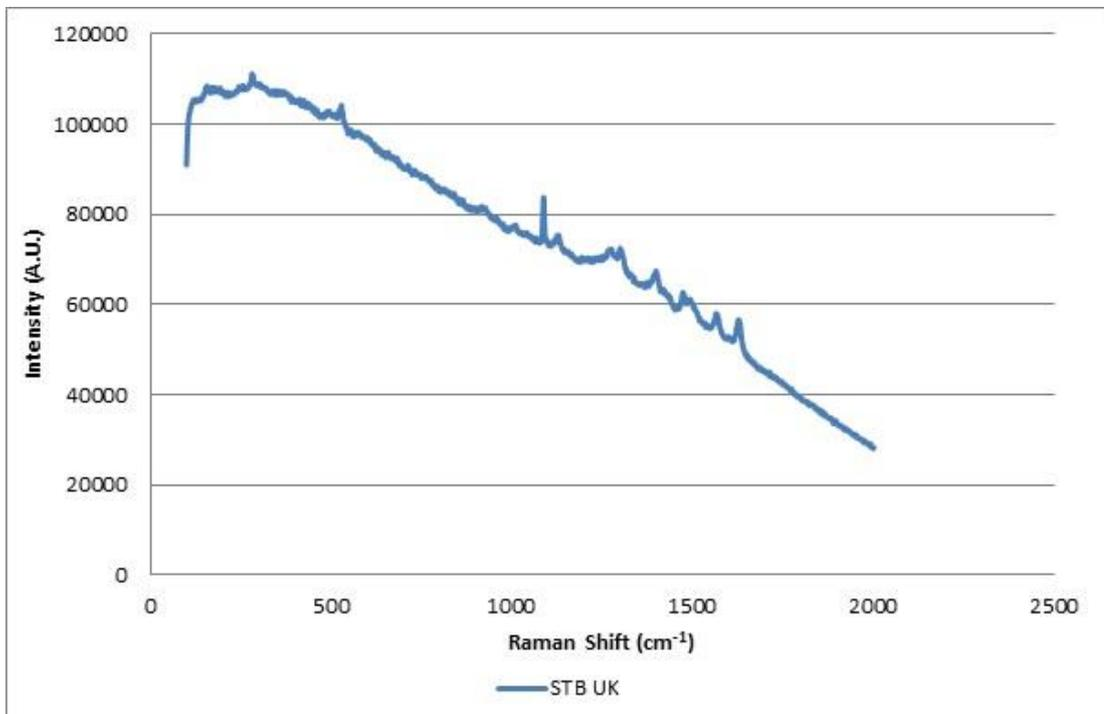
Figure 6.87: Brand/model combination of red gel ink forming Group 8 (Renishaw InVia 785 nm 100% laser power/x 50 obj.)
