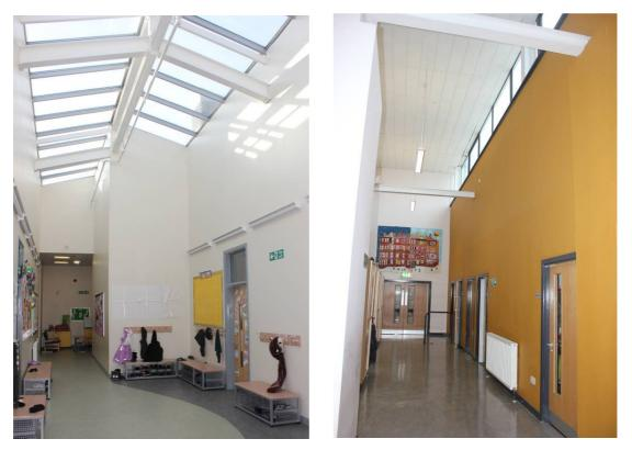
Image 4.34: Photos showing examples of systems used for introducing daylight into corridors in two primary schools.
