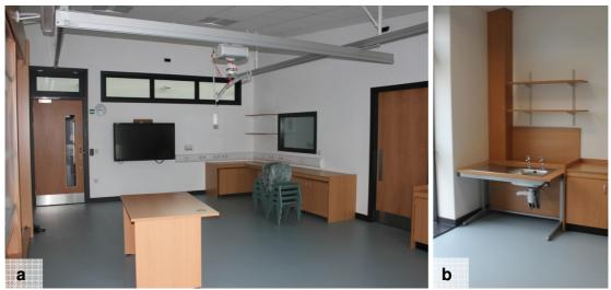
Image 6.27: Classroom showing (a) H-frame wheelchair tracking, door & window to retreat room & touchscreen, & (b) wheelchair accessible, height-adjustable sink.
