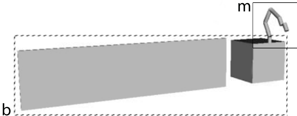
Figure 6.1: Space multibody system composed by the spacecraft platform (bus and solar panel) and the manipulator.
