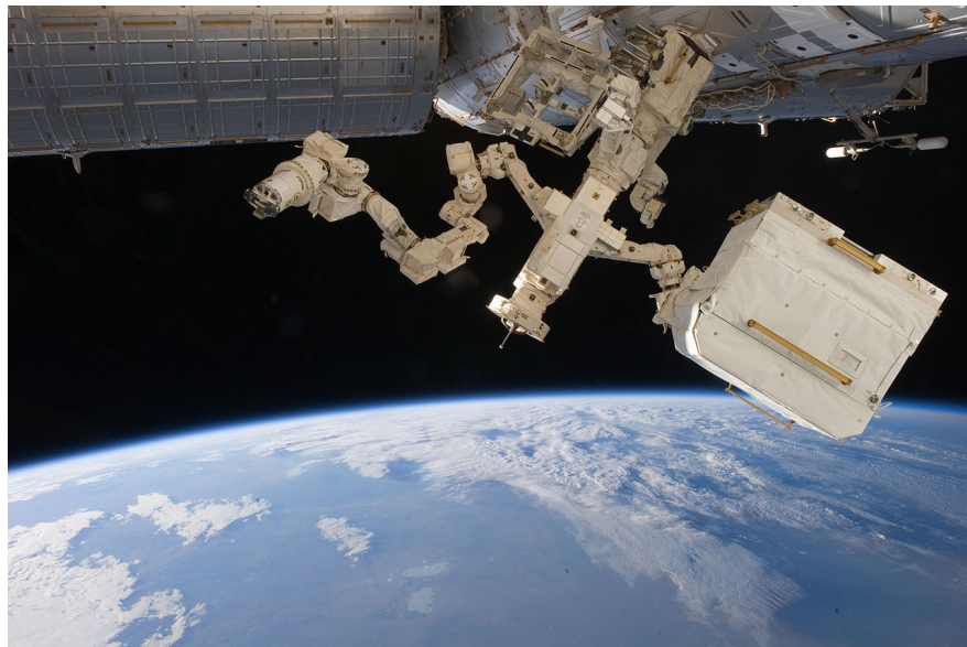
Figure 1.2: The Special Purpose Dexterous Manipulator, the last module added to the Canada's Mobile Servicing System. Image Credit: NASA
