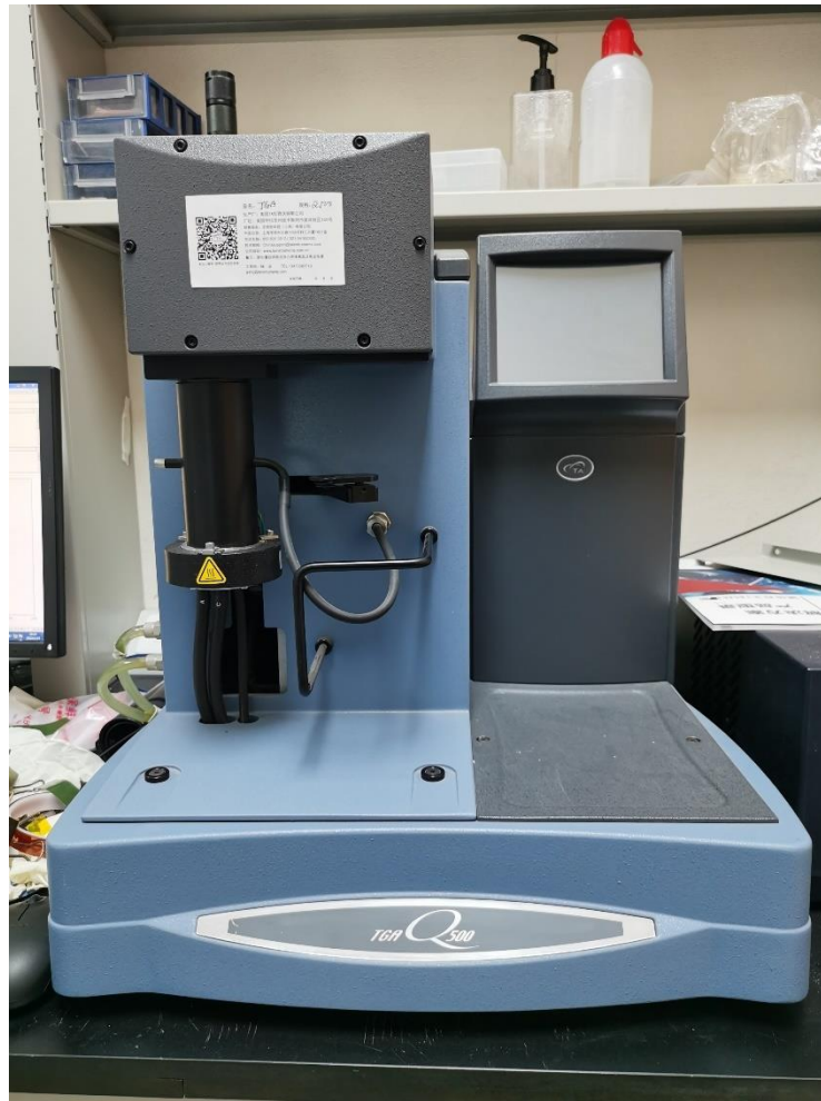
Figure 3.5 The diagram of TGA device (TA Q500)
