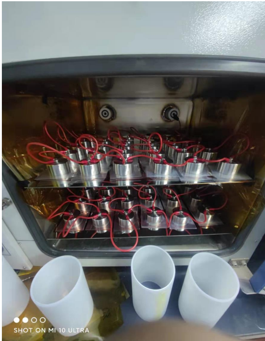
Figure 8.2 The picture of electro-thermal aging process for PP and OpPOSS/PP nanocomposites
