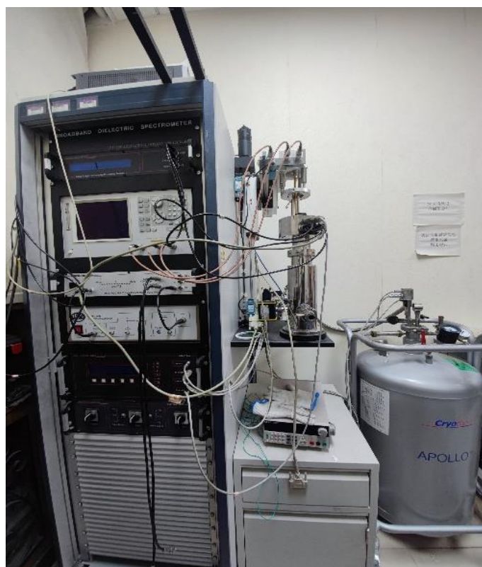
Figure 3.11 The configuration of TSDC measurement system
