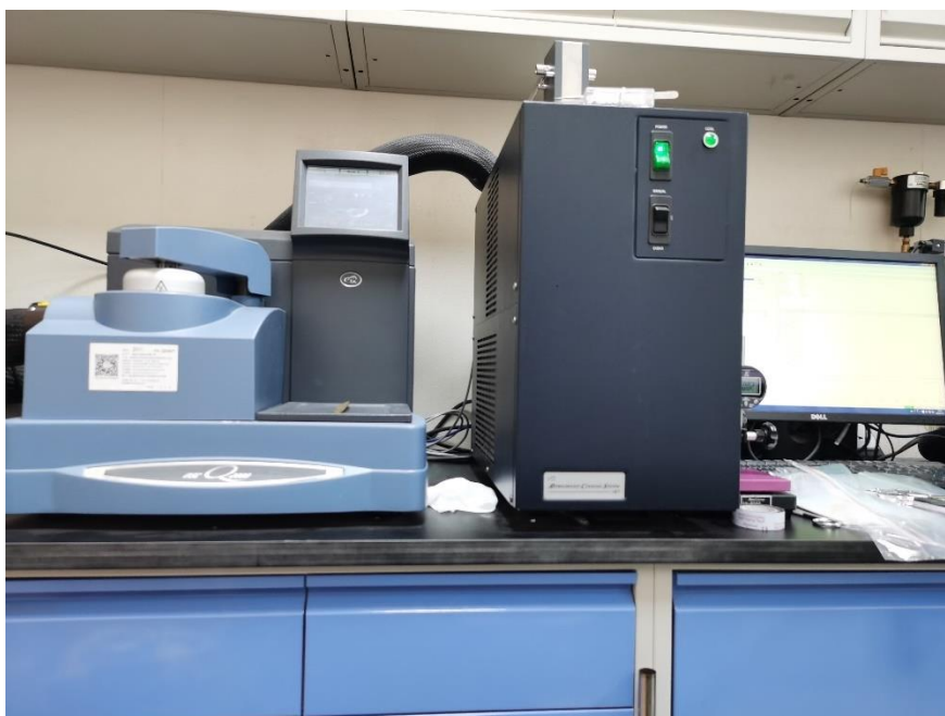
Figure 3.10 The diagram of DSC devices (TA Q2000, USA)
