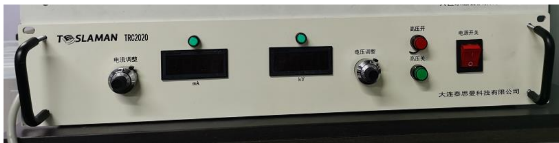
Figure 8.15 the DC power supply in lifespan estimation of PP and OpPOSS/PP nanocomposites
