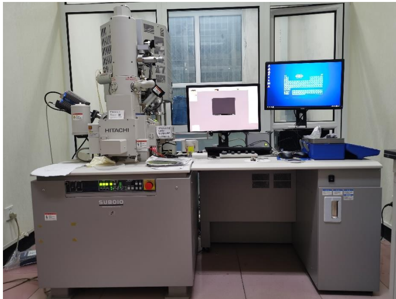
Figure 3.2 The diagram of FE-SEM (Hitachi 8010, Japan)
