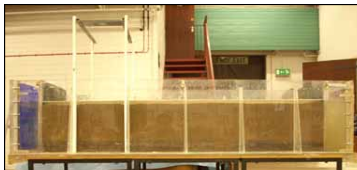
Fig. 2.15: Flooding the model to remove any air bubbles in the soil and settle the sand on a homogeneous horizontal plane.
