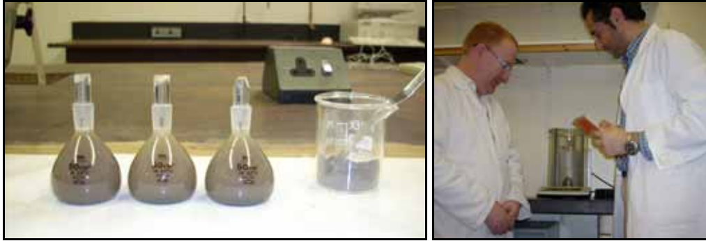
Figs. 2.7 & 2.8: Preparation and measurement phases related to the definition of the specific gravity of soil particles used in the hydrometer test.
