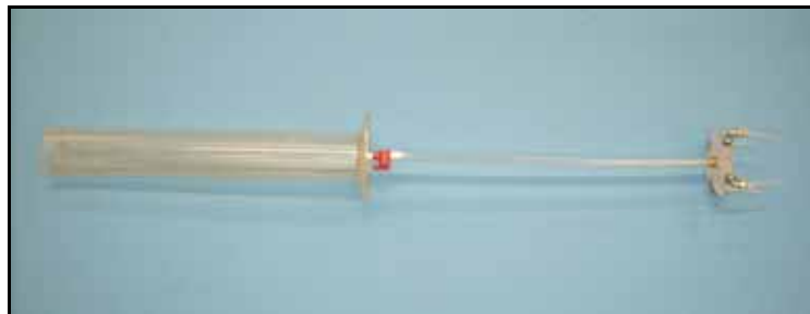
Fig. 2.25: Cylinder to spill pollutant in the sandy layer.
