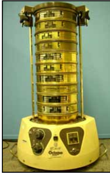
Fig. 2.12: Sieve shaker used to determine the sand fraction passing through a series of sieves with decreasing mesh size.
