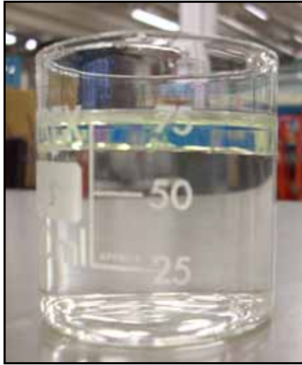
Fig. 2.20: Diesel on the top of the water table.
