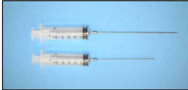
Fig. 2.29: Syringe with a long needle used to sample the groundwater with minimal disturbance to the physical-chemical trim of the model.
