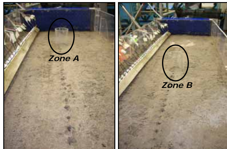
Fig. 2.23: Location of Zona A-B where water and soil specimens were sampled in order to determine the pollutant concentration before barrier installation.
