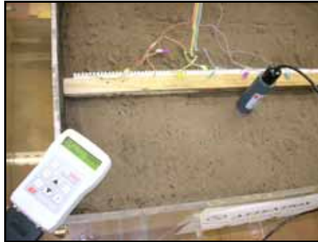
Fig. 2.30: Moisture content meter used to determine the moisture in the sandy and clay soil in different model zones and with different groundwater levels.
