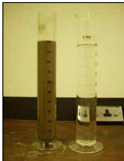
Fig. 2.6: The sedimentation particle size method using a specific gravity hydrometer to measure the soil density in a suspension of water at various time intervals.
