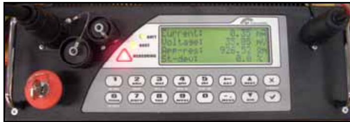
Fig. 3.8: Resistivity meter displaying data recorded during the measurement process (i.e. Current mA; Voltage mV; Standard Deviation %).
