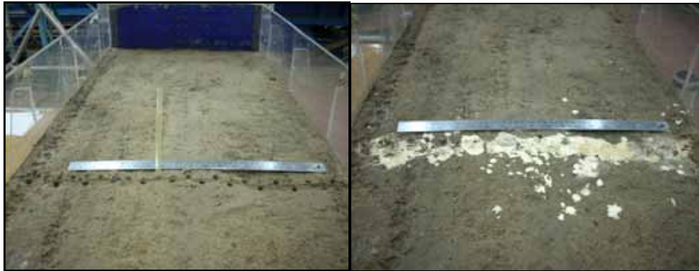
Fig. 2.24: Location of 24 mini-boreholes before and after ORC-Adv injection.
