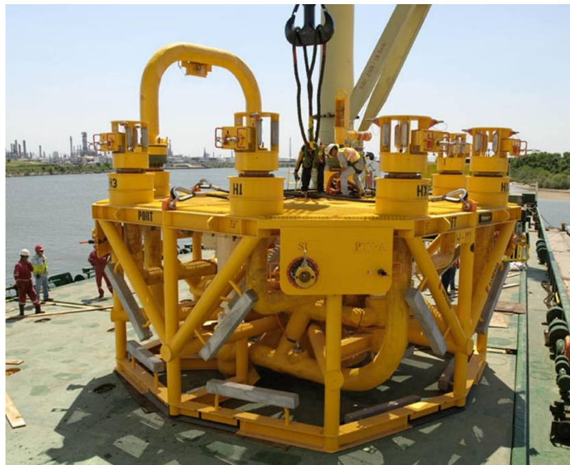
Figure 5.4 Subsea Manifold, OneSubsea-Schlumberger (OneSubsea, 2019)
