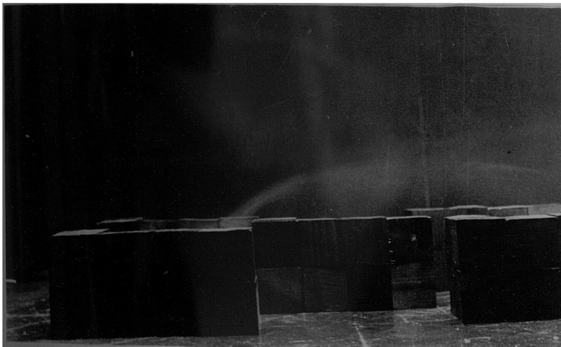
Figure (6.14) Flow pattern around groups of L-shaped blocks, \theta = 90^\circ .
