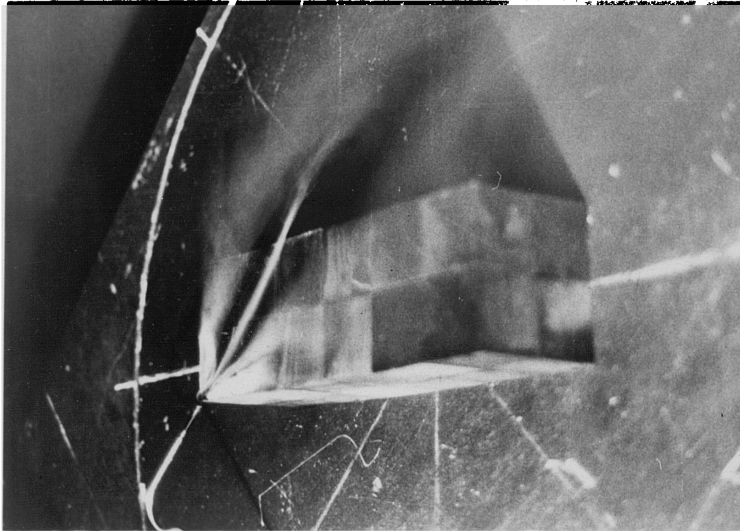
Figure (6.11) Details of regions in the flow pattern around a simple block, \theta = 45^\circ .
