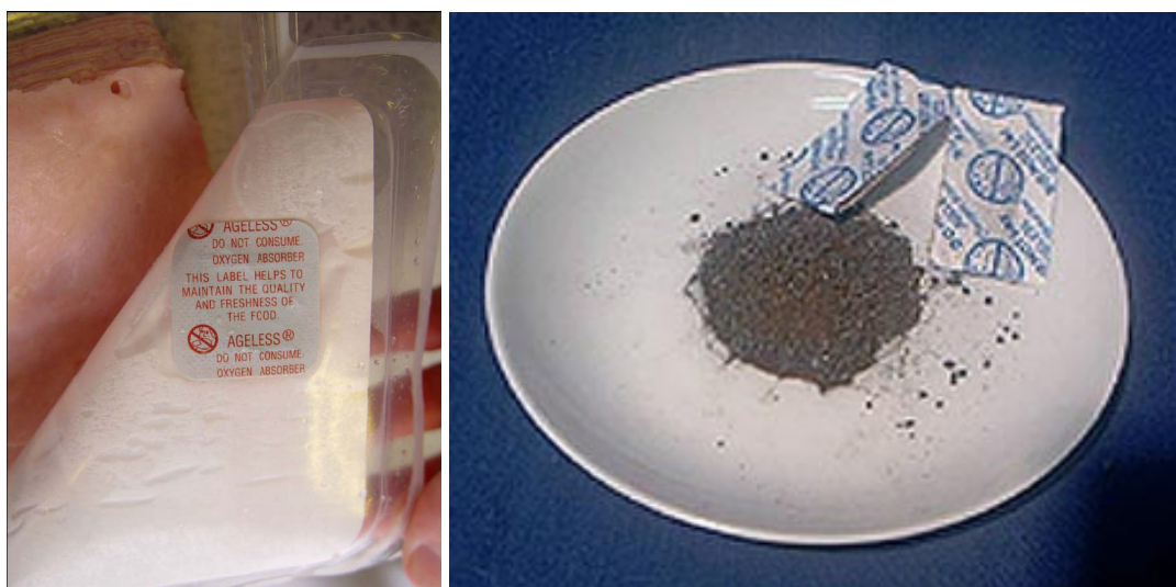
Figure 1.1 Typical oxygen scavenger sachet in a food package; in this case, ham sold by Marks & Spencer, UK. (left), the oxygen scavenger inside the sachet (right). 9
