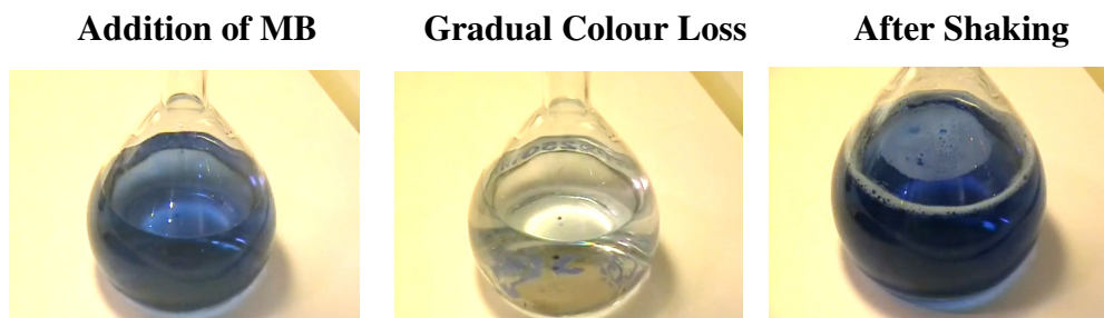
Figure 1.3 The ‘blue bottle’ experiment. A stoppered solution of alkaline glucose with \text{MB}^+ added loses its colour on standing. After shaking the solution, oxygen is re-introduced into solution and oxidises the colourless LMB back to \text{MB}^+ .
