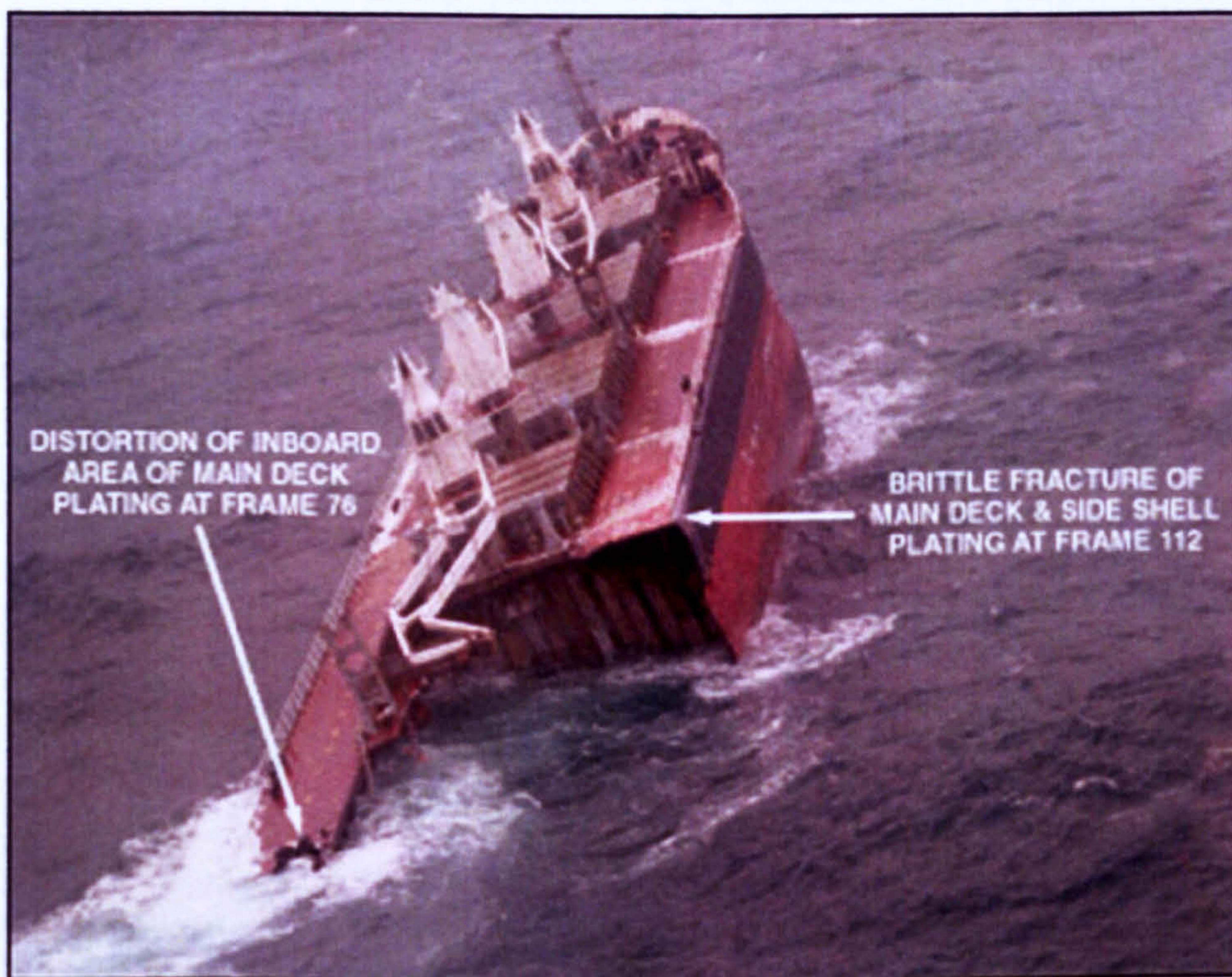
Figure 1-4 Forward section of Flare following brittle fracture
