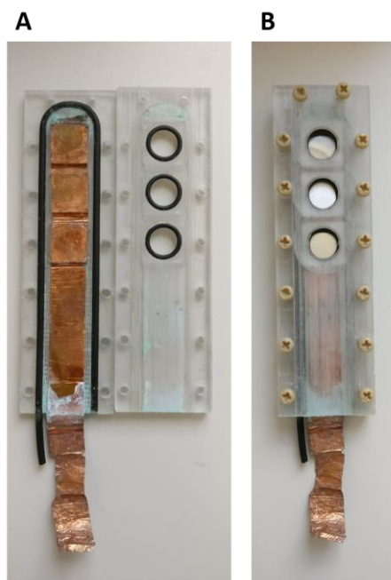
Figure I.13 – (A) Anodisation holder with a copper tape to connect the electrode to the samples. (B) Holder with 3 aluminium samples.
