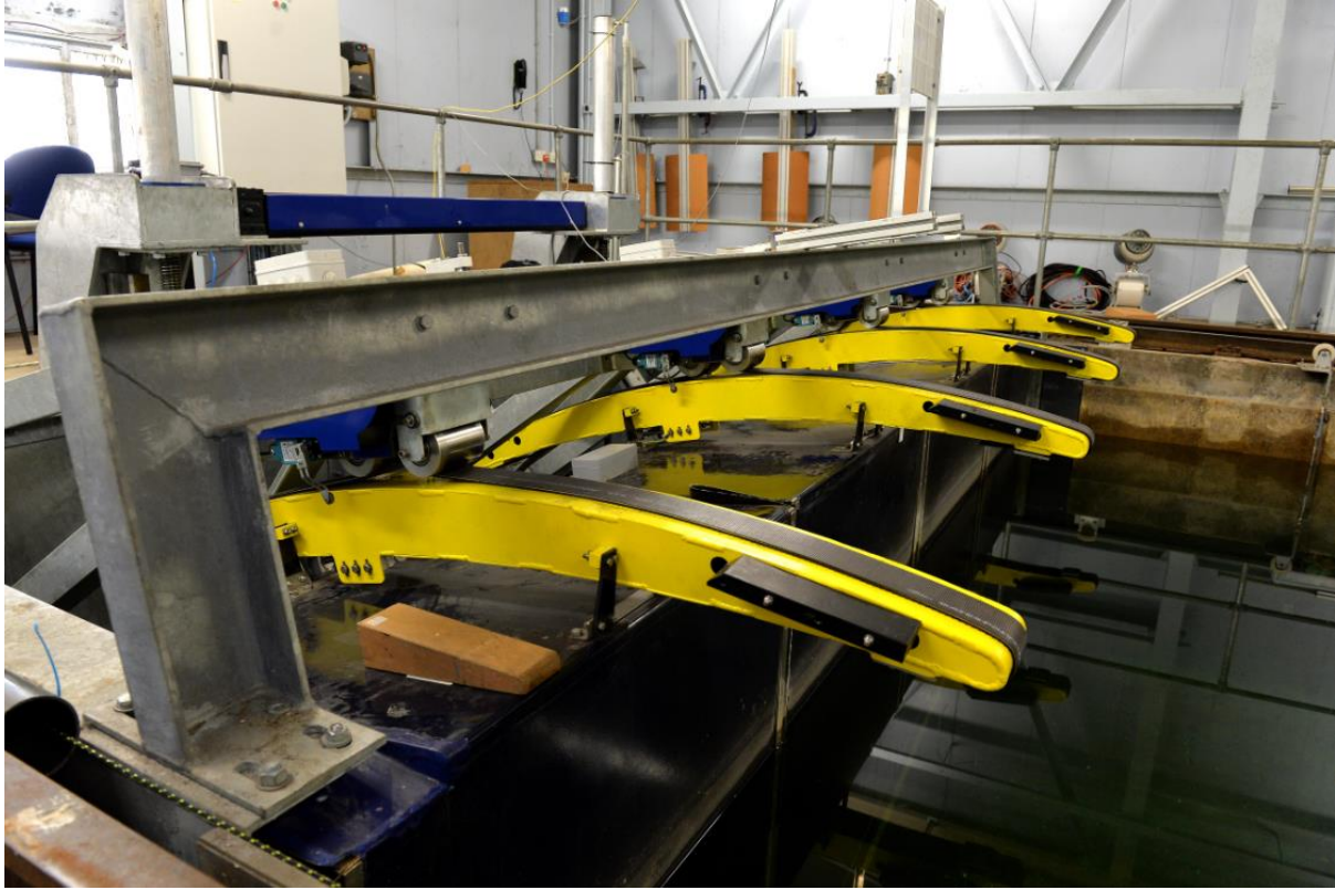
Figure 3-2 Absorbing Wavemaker at Kelvin Hydrodynamics Laboratory
