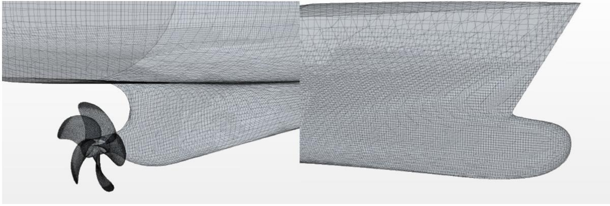
Figure 6-17 Surface mesh on bow and propeller of the hull
