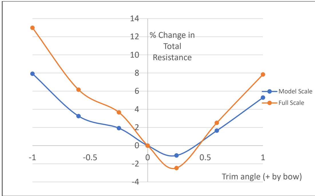
Figure 4-32 Total Resistance differences at Model and Full Scale KCS for different trim angles at 24 Knots at design draft
