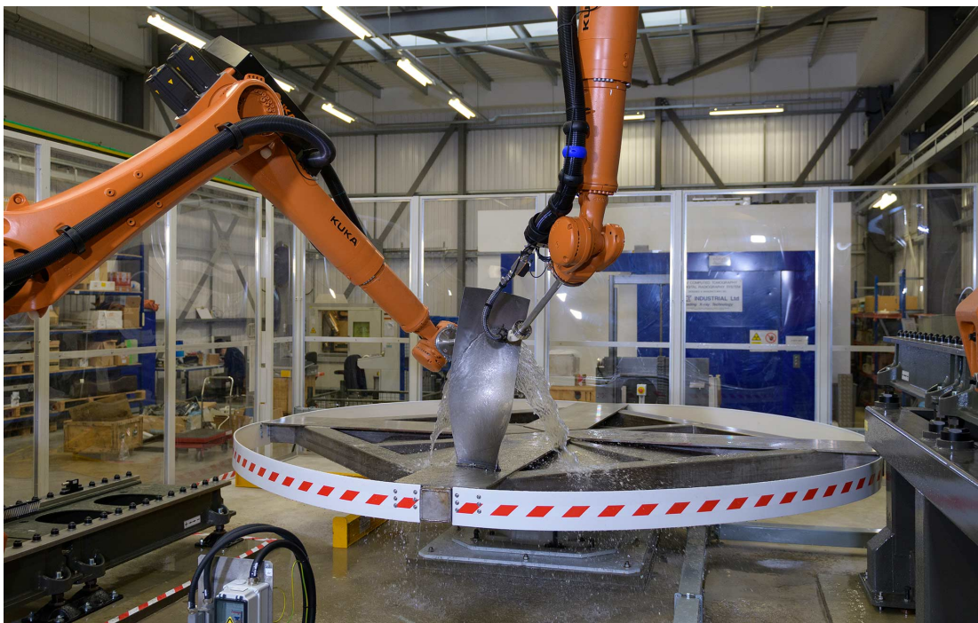
Figure 1.3: Dual robotic cell within TWI undergoing through transmission of a wing part mounted to a rotary table.
