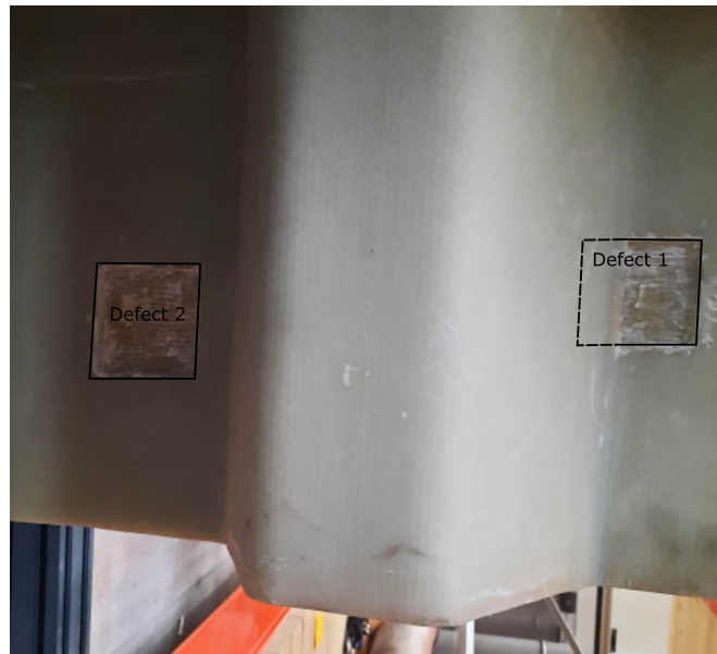
Figure 6.6: View of the part from behind showing the artificial defects embedded within the surface. Their dimensions are 100\text{mm} \times 100\text{mm} since defects below this threshold are not considered critical. Defect one represents a delamination of the stiffener member, cutting through the stiffener and intersecting the non-structural core with a depth of 2\text{mm} from the outside of the hull. A portion of the defect is present under the structural foam, represented by the dotted line. Defect two represents internal tear and wear to the hull's skin with a depth of 5\text{mm} from the outside of the hull. The image is reflected and rotated anti-clockwise by 90^\circ relative to the images produced as a result of scanning later.
