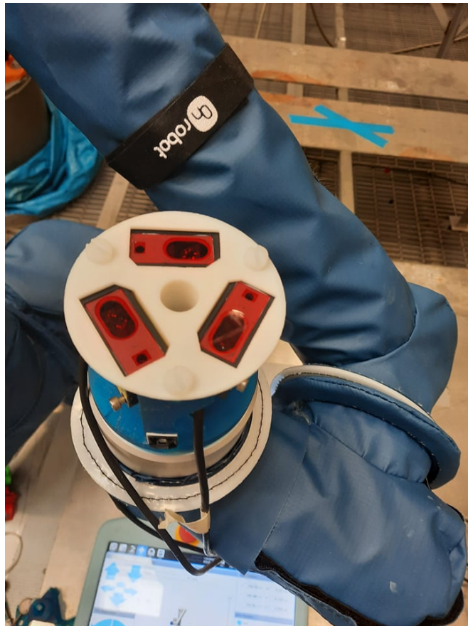
Figure 3.17: The tri-laser holder, attached to the UR10e flange. The design with rotational symmetry around axis 6 of the robot minimised the footprint of the tool.
