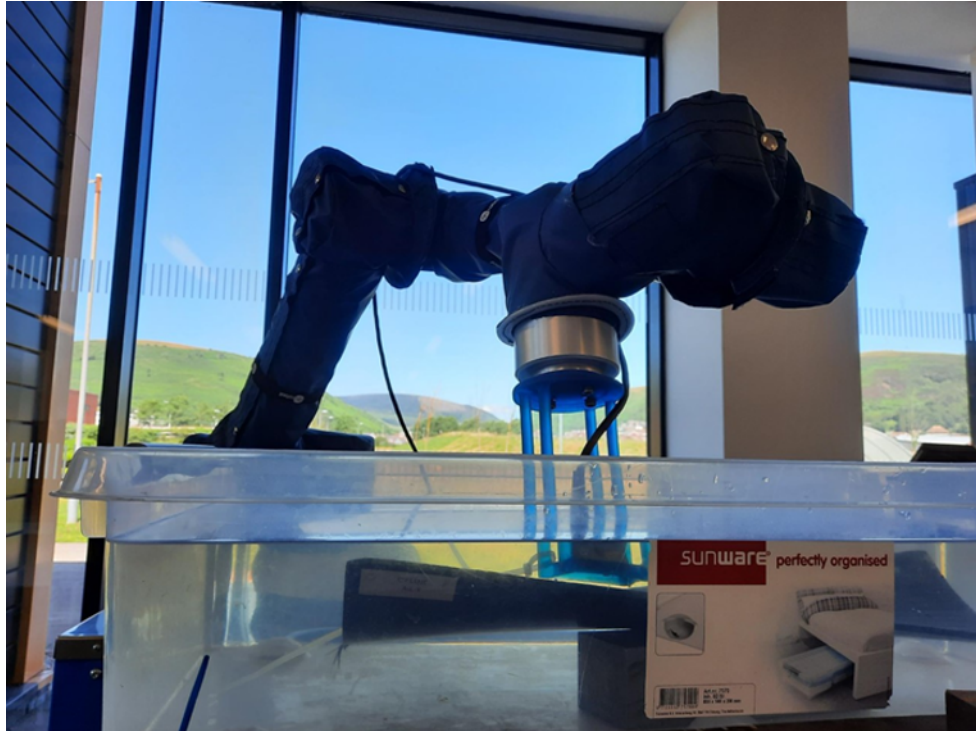
Figure 3.14: Immersion bath set-up of a 5MHz linear PA sensor mounted to an UR10e robotic platform. Flange height and orientation as well as speed limits were in place to prevent submersion or leakage onto the robotic controller.
