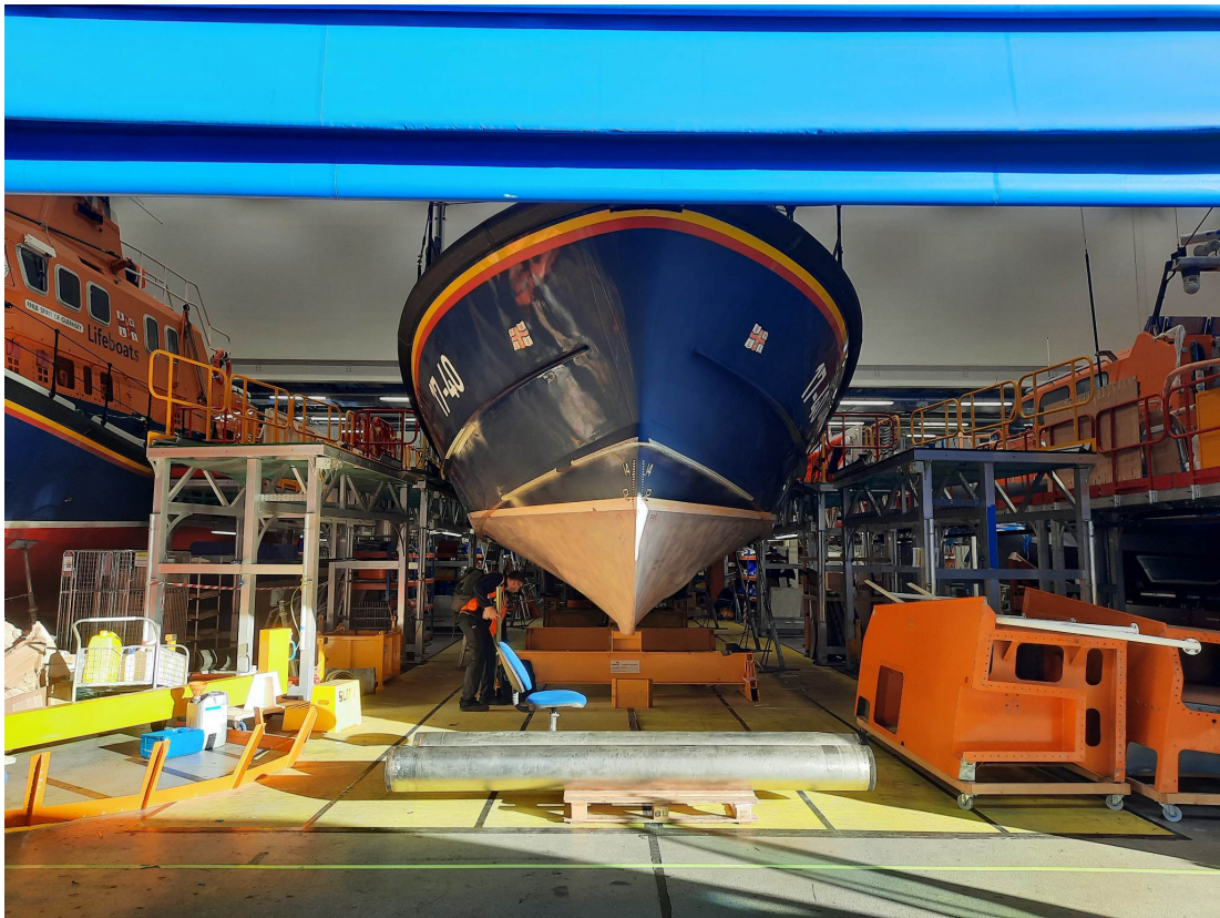
Figure 7.1: A Severn-class lifeboat hull mounted within a dry dock environment. Support structures limited the working volume and provided potential sources of collisions.
