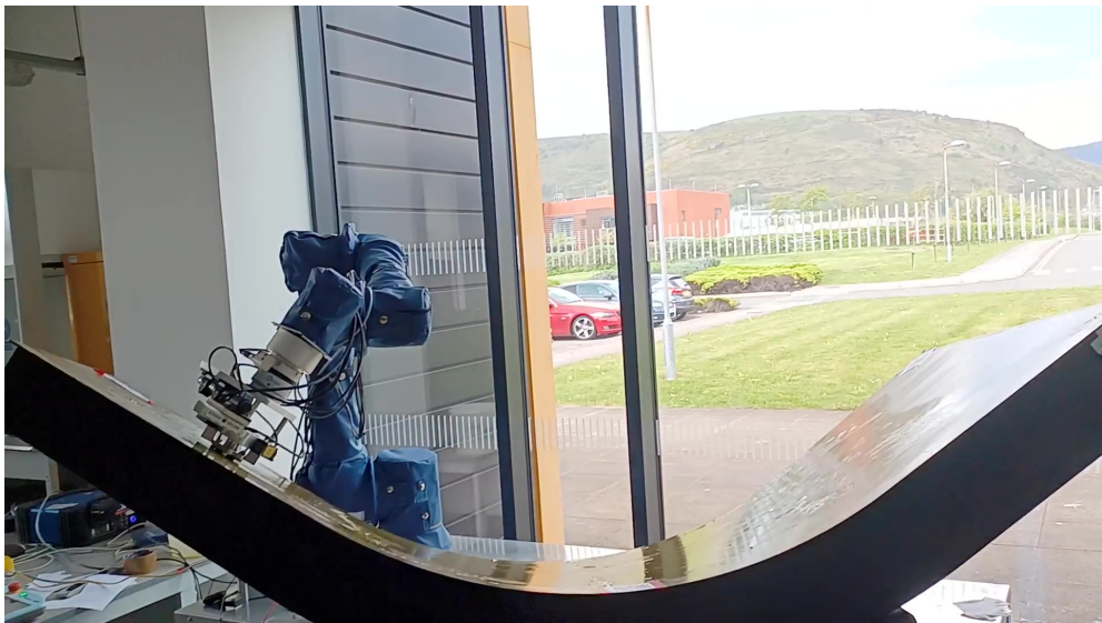
Figure 5.10: Image of the part within the robot cell. The part had to be moved between scans to allow full coverage.
