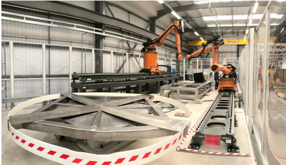
Figure 2.5: TWI's table and track assisted cooperating KUKA KR120 work-cell. The table in the foreground is capable of full revolutions, with the integrated track mounts extending the effective working range of the KUKAs to the entire cell.
