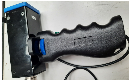
Figure 6.9: EVOTIS Instrumented Tap Testing device features a square faced contact aperture to ensure the strike is normal to the surface, consistent force application, and collects both force and sound time histories.
