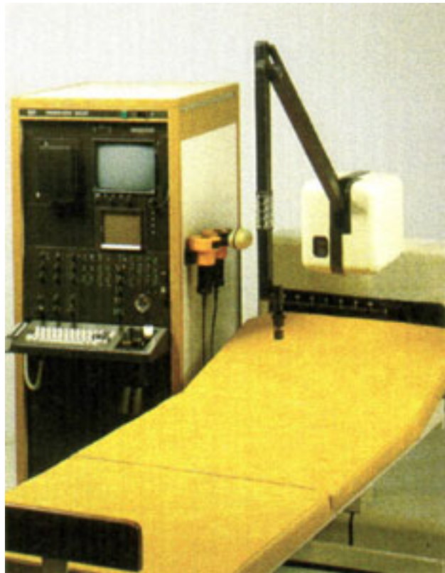
Figure 1.2: The Combison 202 Kretz device would enable recordings of UT data linked to both the position and pose of the device while an operator guided it along portions of a patient's body.
