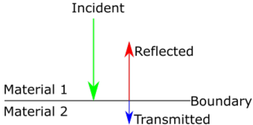
Figure 2.1: Illustration of energy transmission through media. The arrow size represent the proportion of the initial energy incident at the boundary.
