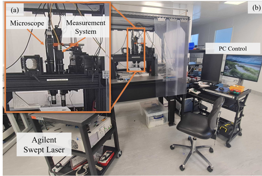
Figure 5.3: Configuration of Transfer Printer for in-situ PhCC measurements. Overview of transfer printer setup. (a) Inset of showing the dual column setup of microscope for print alignment and cross-polarised measurement system for device testing. (b) Wide-view showing swept laser system and PC control interface.
