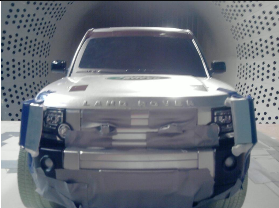
Figure 83 - side turning vanes
