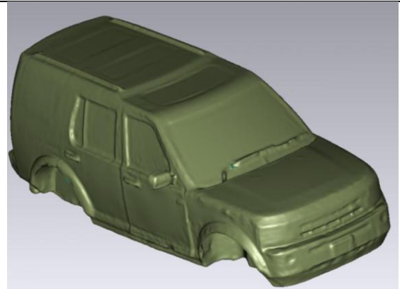
Figure 16 - Initial NURBS surface creation in Geomagic
