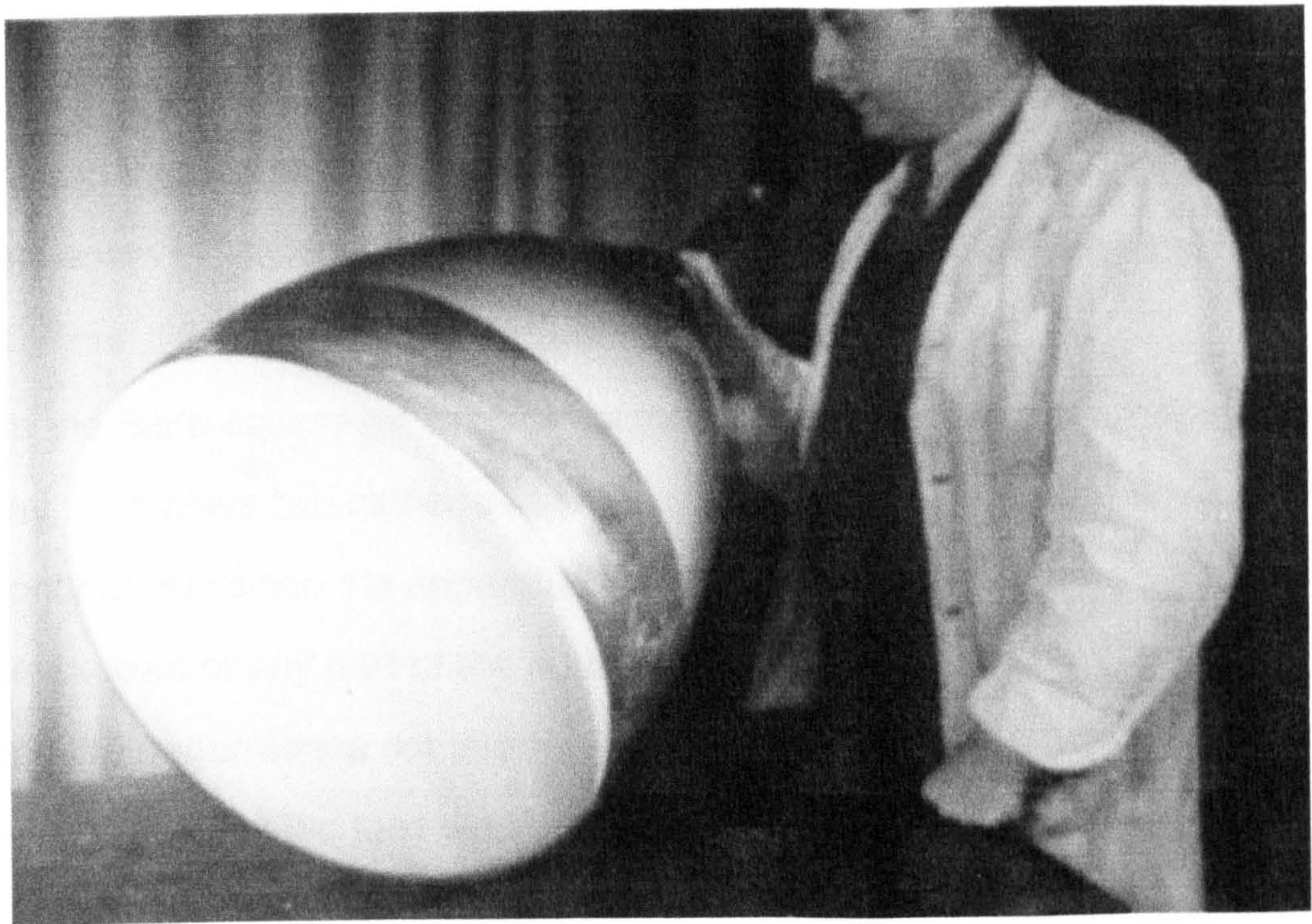
5.20: Szegho's 22 inch Baird Cathode-ray Tube
