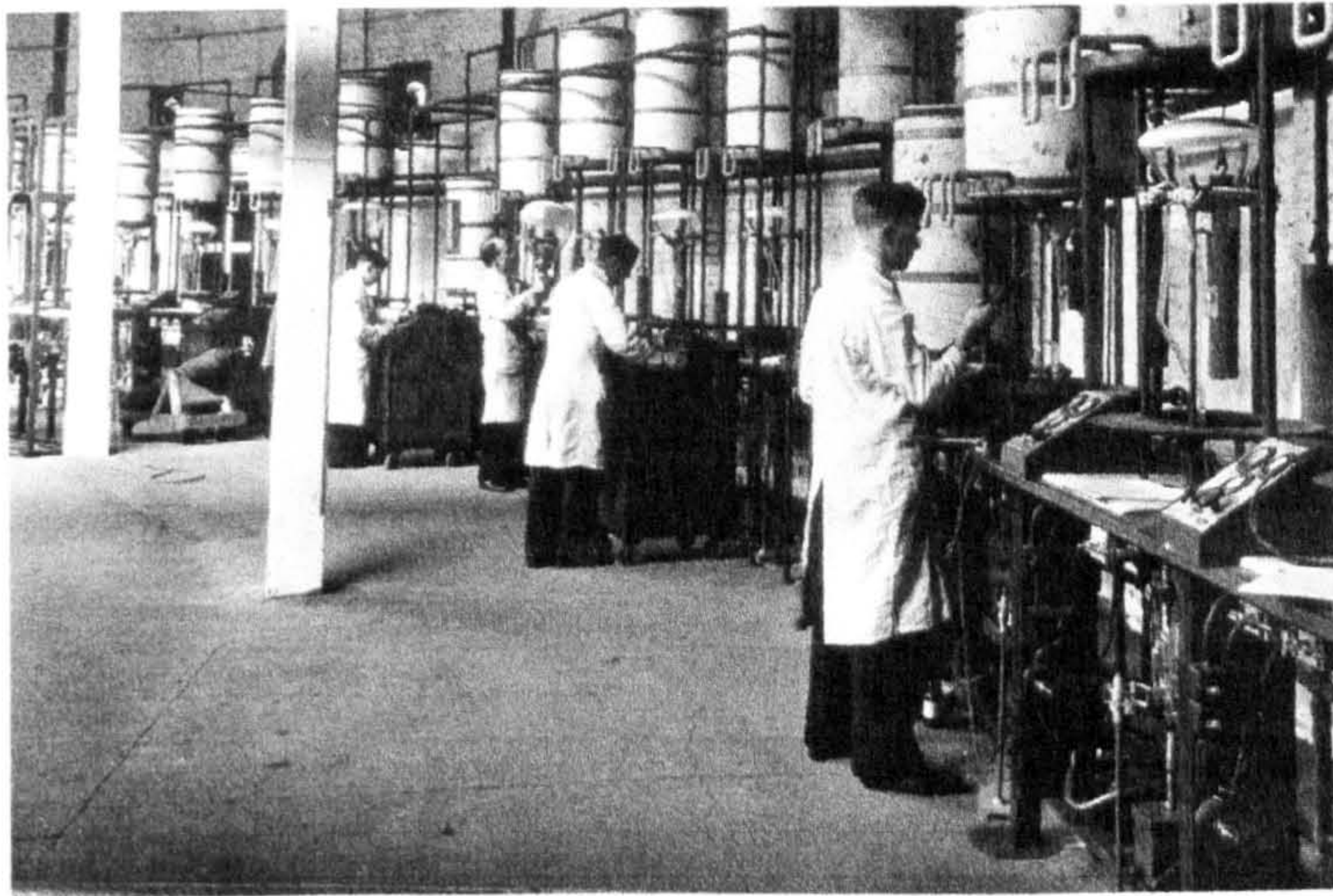
Figure 3.39: Using an Eddy Current Heater to Outgas the electrode structures and activate the cathode.
