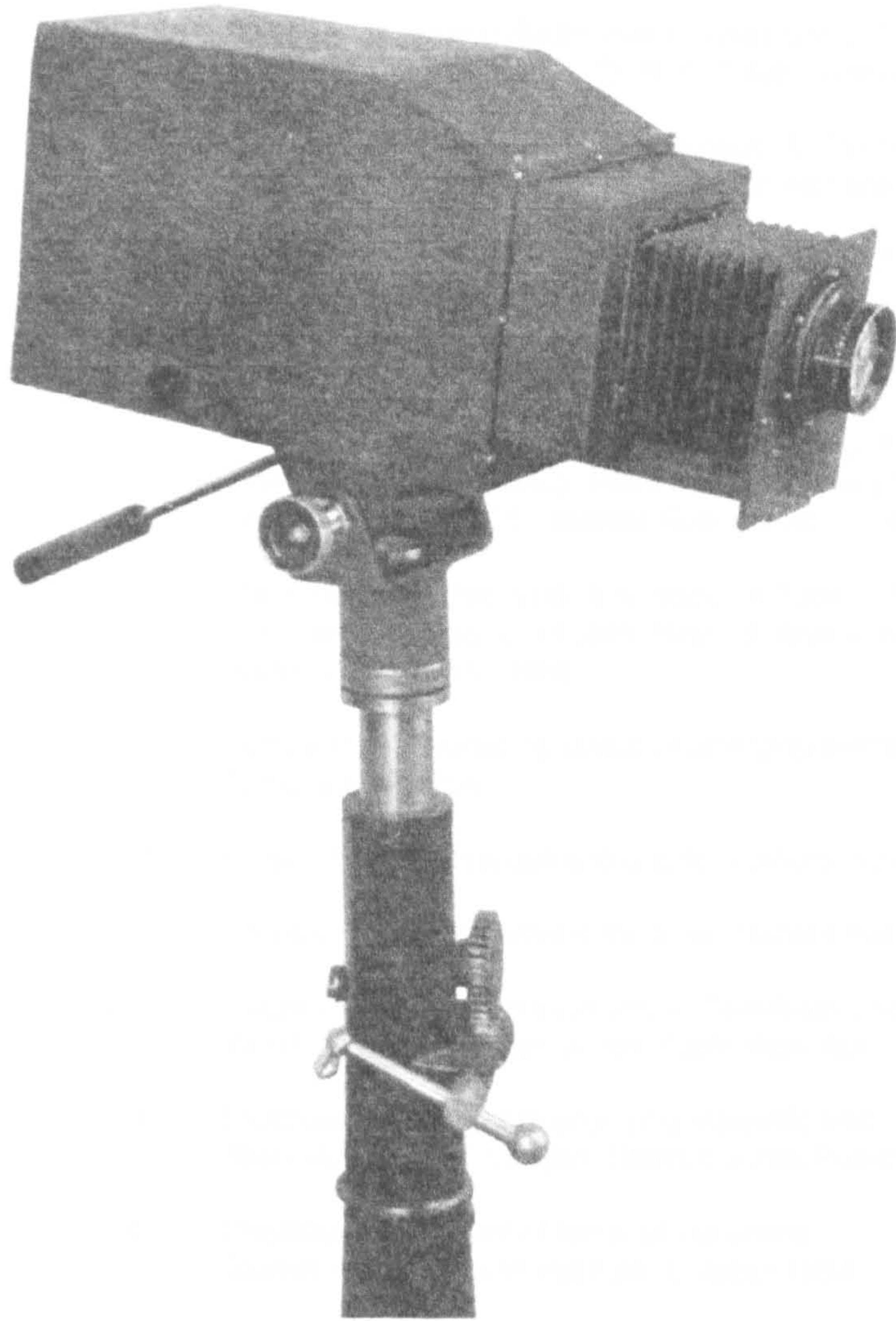
Figure 2.1: Farnsworth's Dissector-Multiplier Camera October 1934
