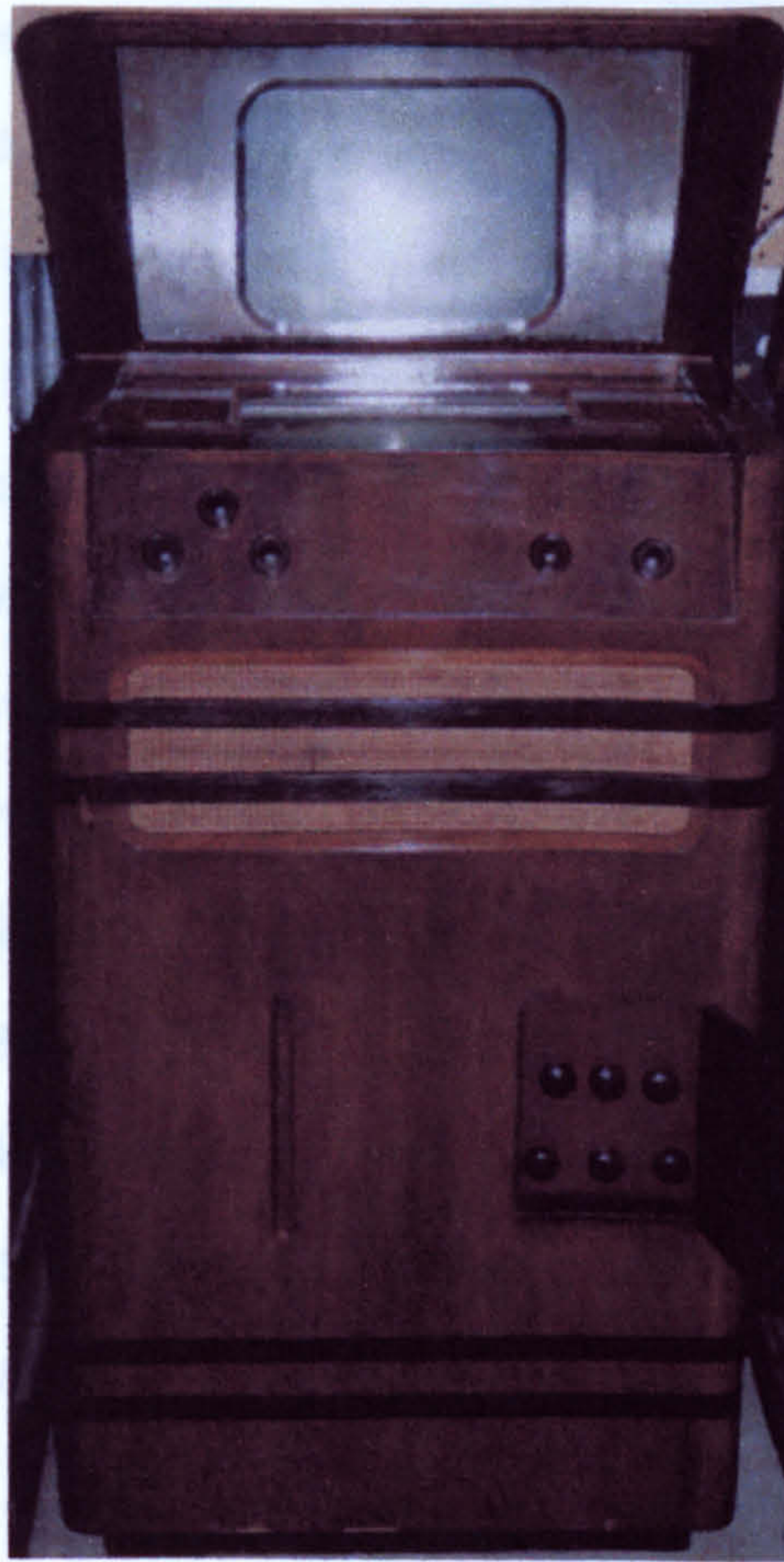
Figure 4.2: The Baird T.5 (1936) with the vertically mounted 15inch 15 WMI Baird cathovisor Tube
