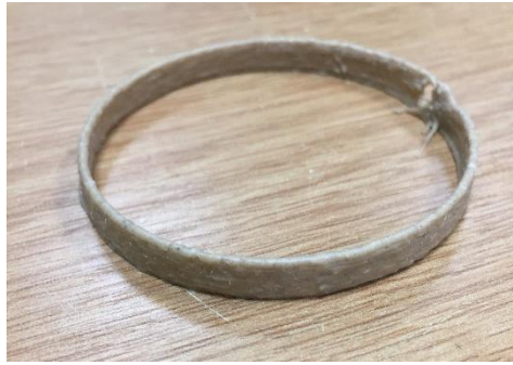
Figure 4.11 – Ten layer printed buildability ring.
