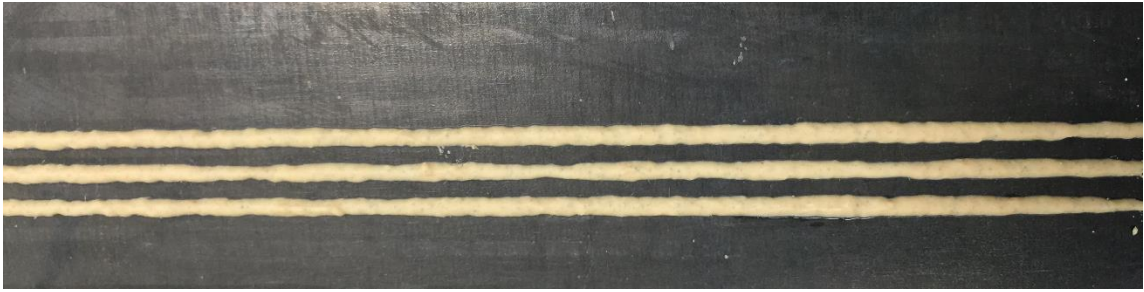
Figure 4.8 – Extrudability assessment of mix design by printing three 200 mm lines.
