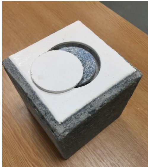
Figure A.5 – Delamination of patch during coring for adhesion tests.
