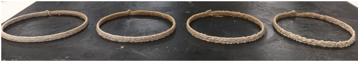
Figure 4.5 – Printed objects with different surface quality due head distance issues (head distance increases from left to right).
