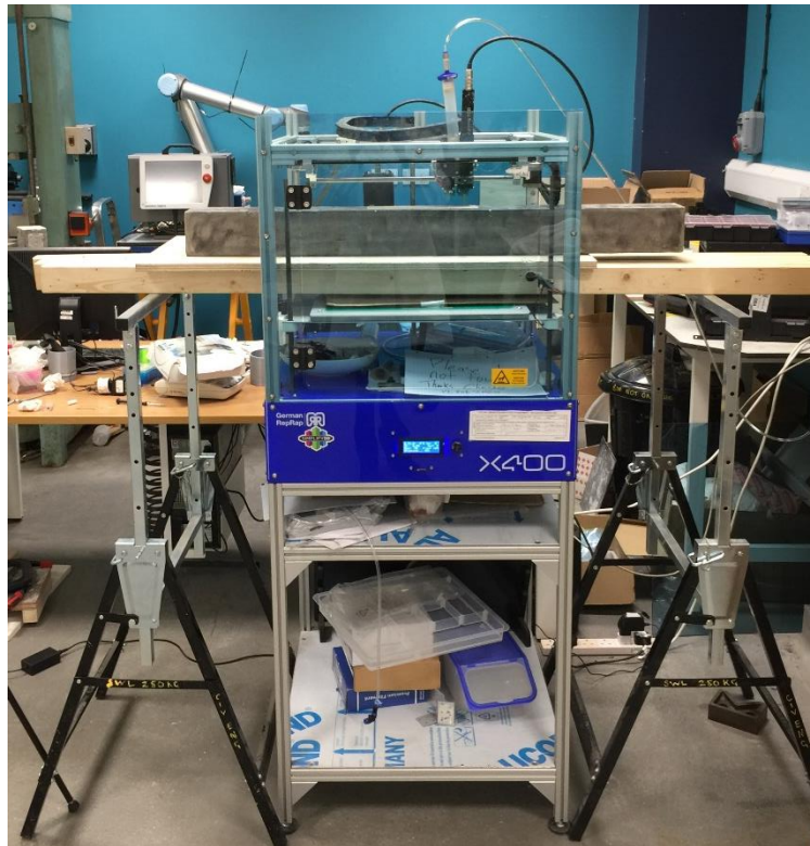
Figure 7.2 – Extrusion of patch onto 1000 mm concrete beam with the use of stationary 3D printer. The walls of the printer were removed and supports were used to accommodate the size and weight requirements of this application.
