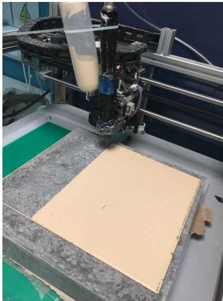
Figure 7.1 – Patch printed onto 200 mm \times 200 mm concrete slab.
