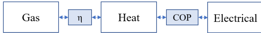
Figure 4-12 Gas, Direct Heat and Electrical heat type demands and their associated conversion factors \eta (gas to heat conversion efficiency) and COP (coefficient of performance, heat to electrical heat conversion efficiency)
