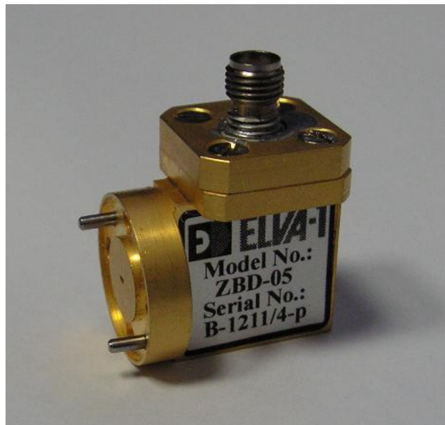
Figure 4.7: Zero-biased detector for 140 - 220 GHz signals.
