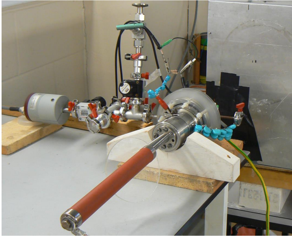
Figure 5.25: Experimental setup of BWO frequency determination experiments.
