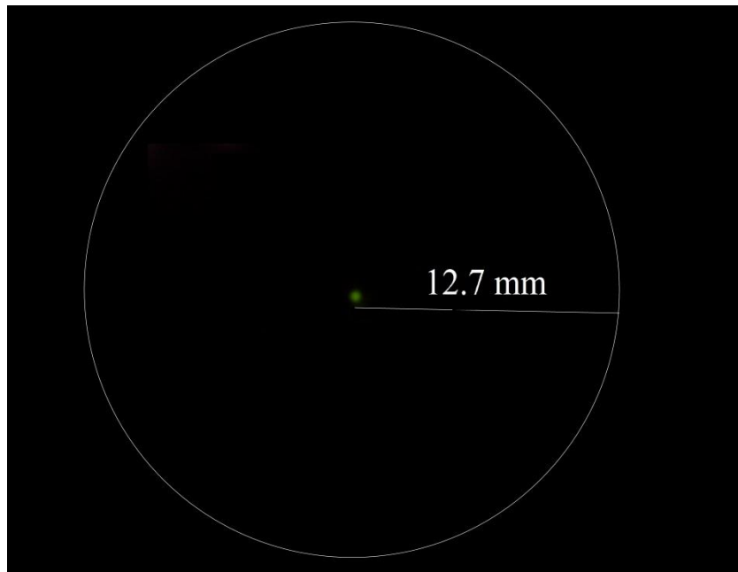
Figure 5.12: Scintillated image of a 1 mm diameter PS-generated electron beam.
