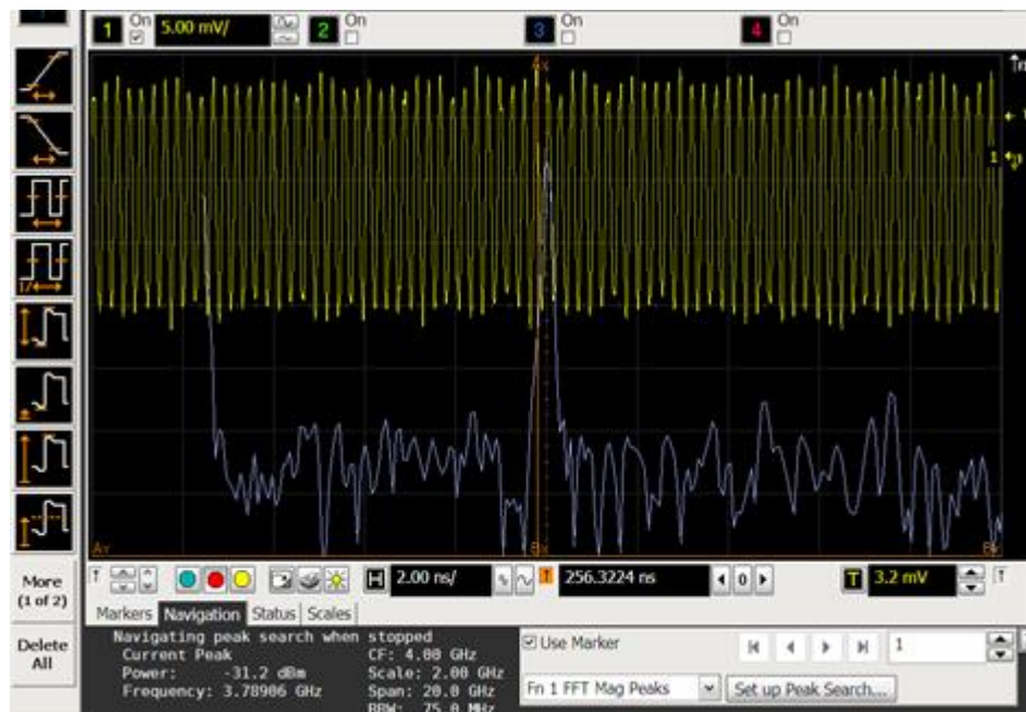
Figure 4.10: Oscilloscope display of an IF signal in yellow and its Fourier transform in blue.
