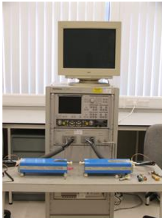
Figure 4.11: Anritsu VNA with 140 - 220 GHz extension modules connected.
