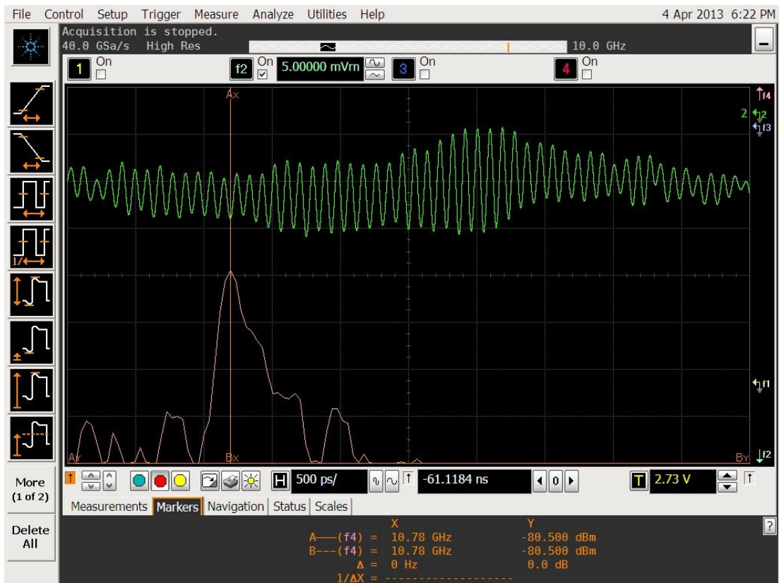
Figure 5.26: Oscilloscope reading of IF signal derived from a BWO pulse, showing pulse amplitude, green, and FFT of signal, purple.
