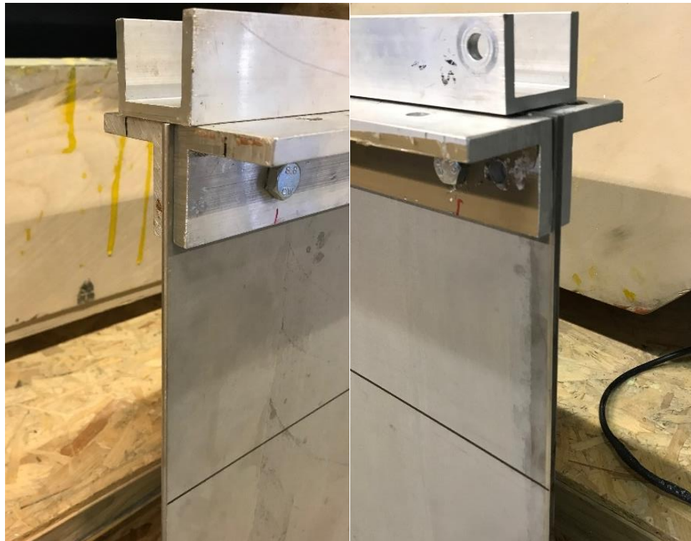
(a) (b) Figure 5-8: Flat plate details: (a) Leading-edge; (b) Trailing-edge.
