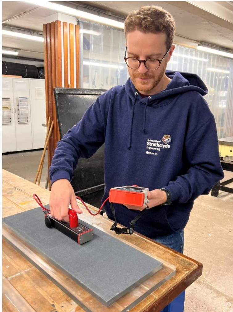
Figure 4-4: Process of taking a roughness measurement of Sand 220 with the TQC Hull Roughness Gauge (“TQC,” 2022).
