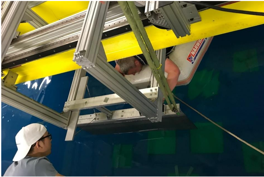
Figure 5-7: Rigging operations of the flat plate on the carriage.
