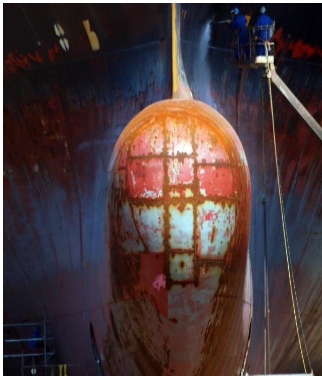
Figure 1-1: Hull cleaning operations. Photo credit: IMO - Lee Adamson.
