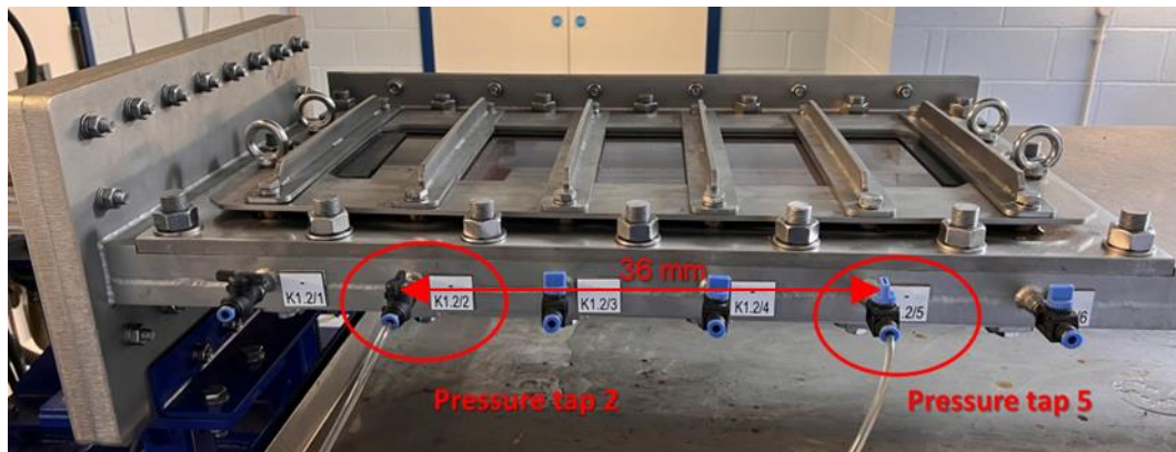
Figure 4-10: Pressure taps distribution numbered from 1 to 6 (left to right) on the test section of the FTFC.
