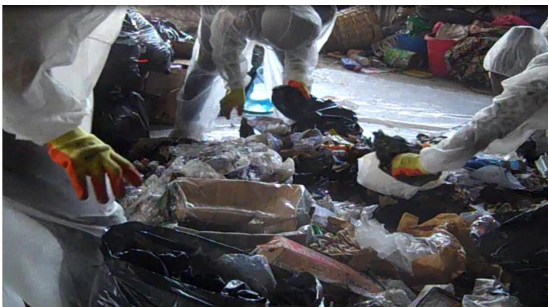
Figure 4.10: High LDPE content found during waste analysis sorting process; of the 71.5 kg of plastic waste sampled, 36.5 kg was 'nylon' sachet water and 35.0 kg was PET plastic bottles.
