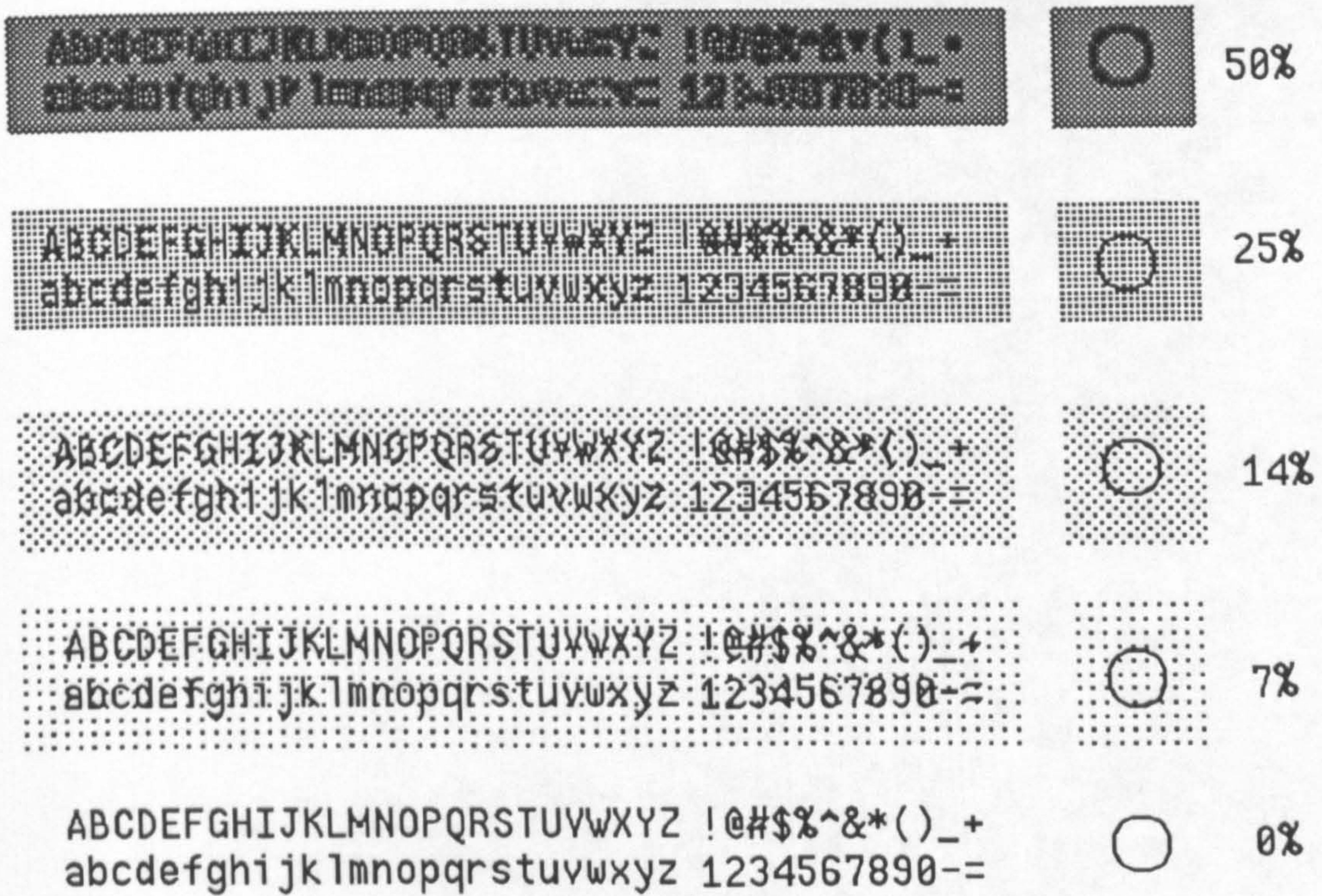
Figure 4.7.8.1.1.1. % grey scale pattern ORed to obscure text and images
