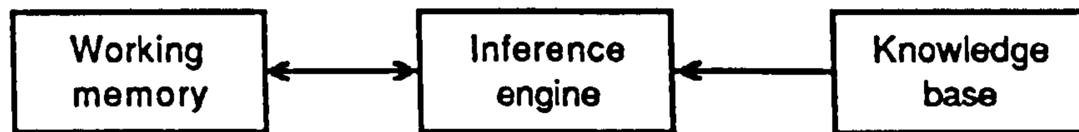
Figure 2.5.9.1. Example of the classical expert system structure
