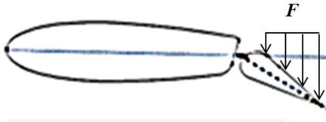
(c) Sketch of vertical axis turbine blade with passive oscillation flap
