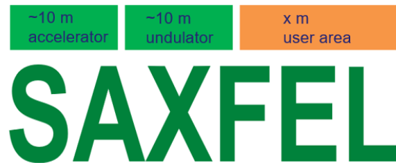
Figure 6.2: Conceptual, the basic layout of SAXFEL, a potential X-FEL in Saudi Arabia. The accelerator part would be based on a hybrid LWFA-PWFA-System, with a plasma photocathode based on principles and insights-driven forward as part of this thesis. Thanks to the ultrahigh brightness provided by such electron beams, an undulator of only \sim 10 m length may be sufficient to generate soft to hard x-ray pulses, which then could be used for experiments in the user area.
