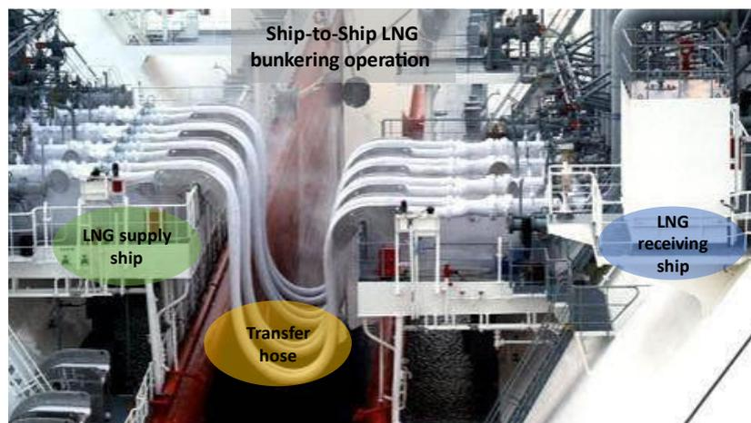
**Figure 9. 4** Ship-to-Ship LNG bunkering operation(KLAW, 2022)
