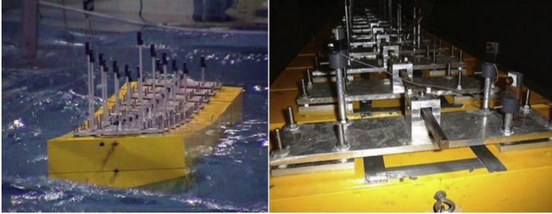
Figure 4.6: Hydroelastic experiments of the floating barge model, pictures from (Lakshmyanarayanan et al. 2019) and (Senjanović et al. 2008).
