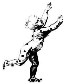
Figure 1.71: LAMB markers set up: circles indicate anatomical markers, squares technical markers and triangles calibrated anatomical landmarks (Rabuffetti and Crenna, 2004).
