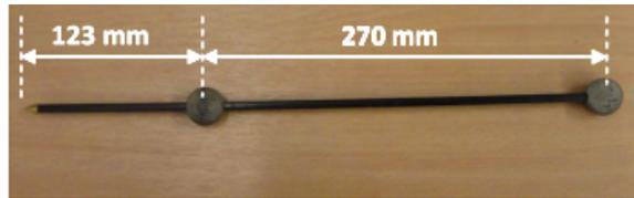
Figure 2.11: Pointer used for anatomical landmark calibration in static trials.
