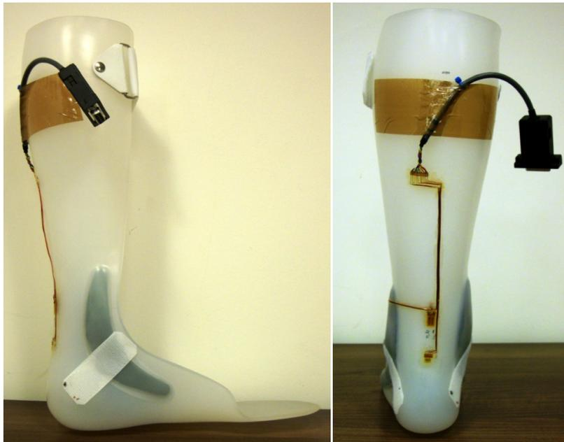
Figure 4.19: Medial and posterior view of the strain gauged AFO.
