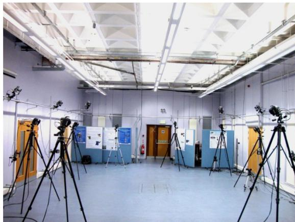
Figure 2.8: Laboratory configuration with camera on high tripods (Vicon 612) and camera on the wall trail (Vicon MX Giganet). Not all the cameras connected to the new system are visible.
