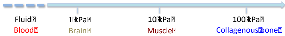
Figure 3.7 Solid tissues exhibit a range of stiffness, as measured by the elastic modulus. (Engler et al., 2006)
