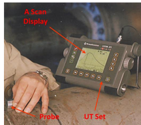
Figure 2-24 Ultrasonic Testing (UT) equipment (TWI.Ltd, 2018d)
