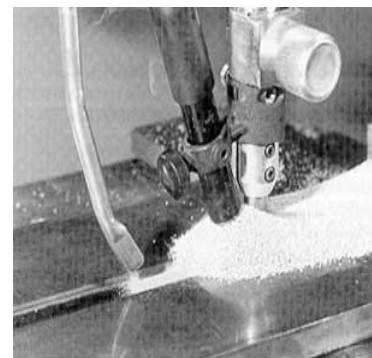
Figure 2-10 Submerged Arc Welding (SAW): Principle (Left), Process in practice (TWI, 2018 a)
