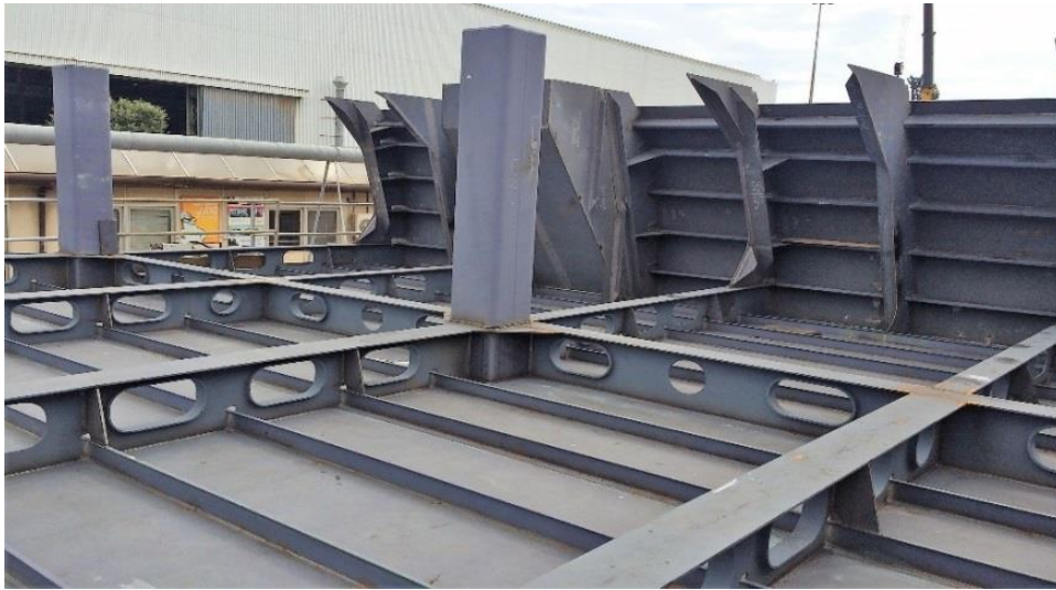
Figure 2-3 Assembly of pre-assembled parts in blocks
