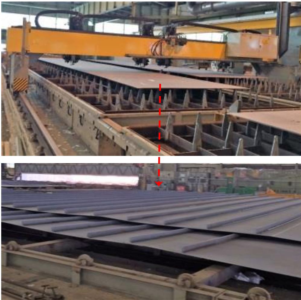
Figure 2-2 Part 1: Panel line and sub-assembly
