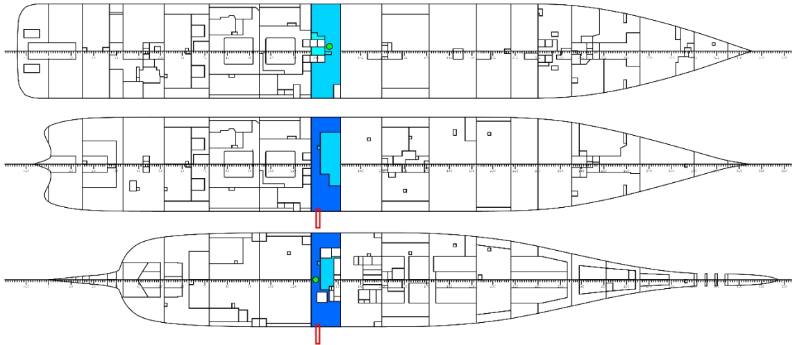
Figure 10-3: Additional progressive flooding extent for Test-case 2, Striking vessel length: 100 m, H_s = 5.0 m and H_s = 10.0 (Breach shown as red square, Initial flooding shown in dark blue, initial progressive flooding shown in light blue, additional progressive flooding shown in lighter blue and flooding sensors shown in green).
