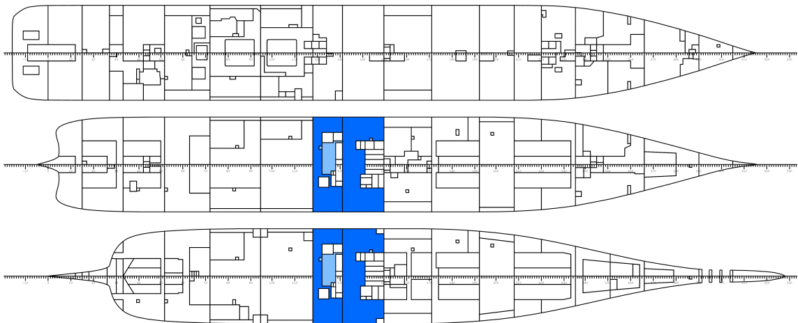
Figure 6-40: Progressive flooding realization 2, P = 0.206 .
