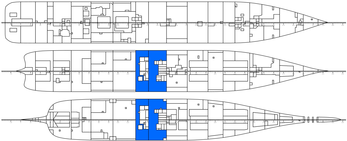
Figure 6-41: Progressive flooding realization 3, P = 0.115 .
