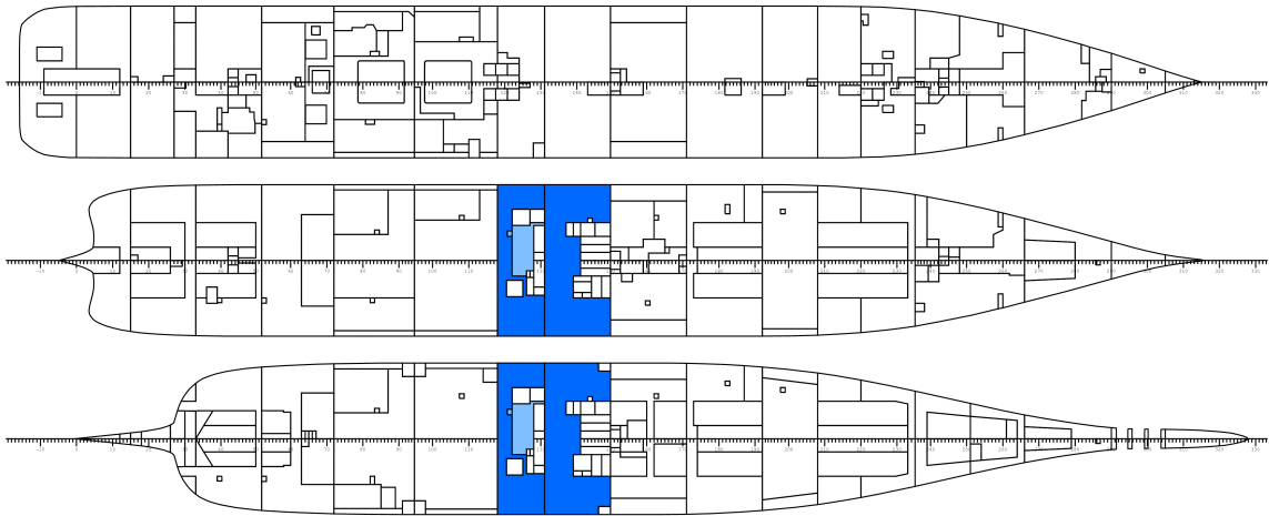
Figure 6-39: Progressive flooding realization 1, P = 0.233 .
