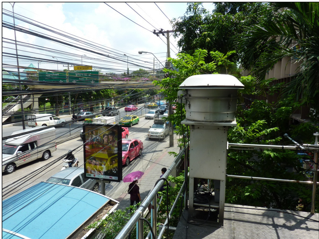
Figure B.2 PM 10 sampling equipment at the roadside site.
