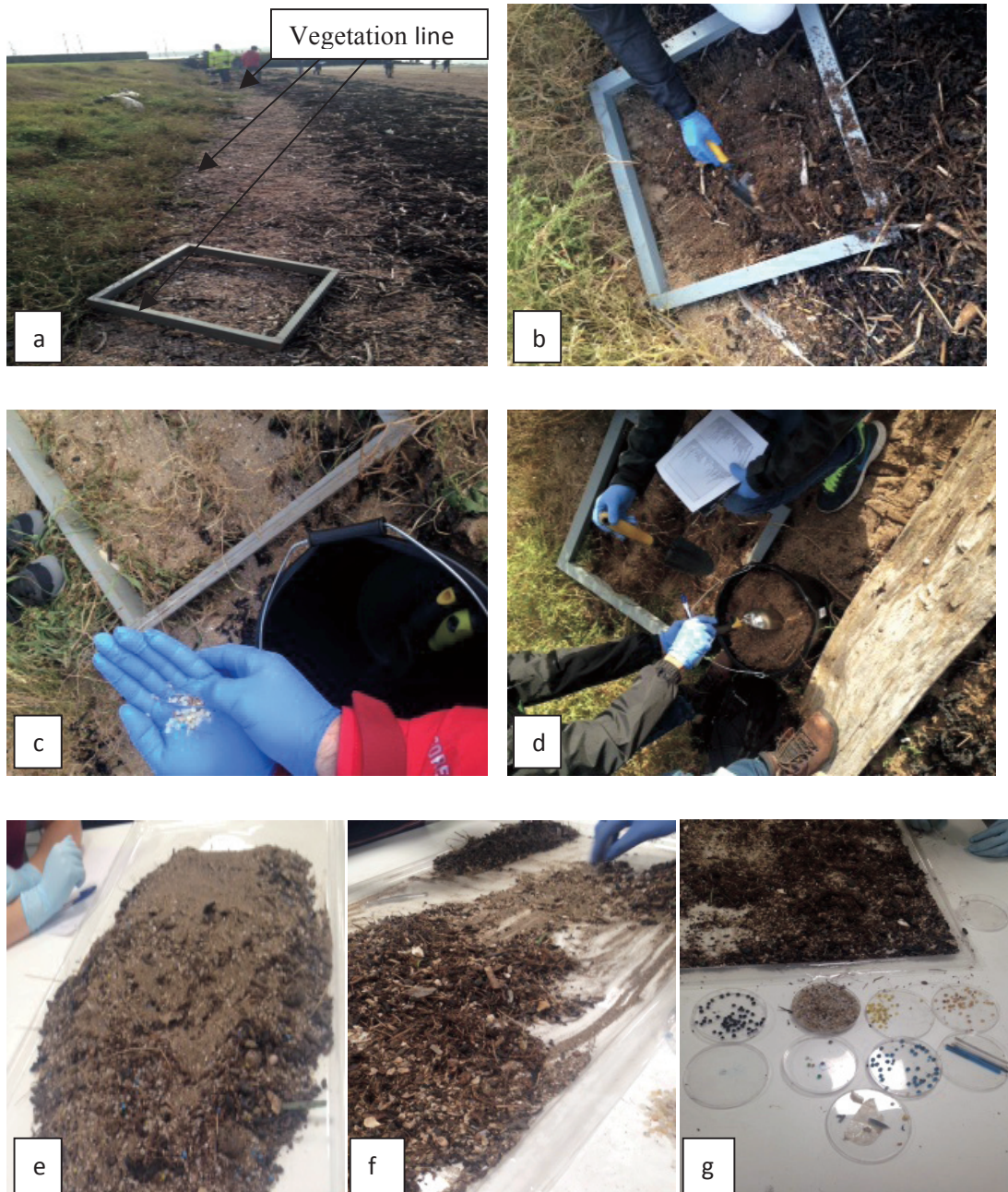
Figure 6-5 Sampling and picking out plastic resin pellets in Limekilns, Scotland, using a quadrat technique. a: quadrat frame at vegetation line, b: digging ~5 cm depth sediment, c: examples of pellets being collected, d: obtaining the sample in bucket filled with sediment, e: sediment after air drying in the lab, f: picking out pellets manually after sieving, g: different pellets collected.
