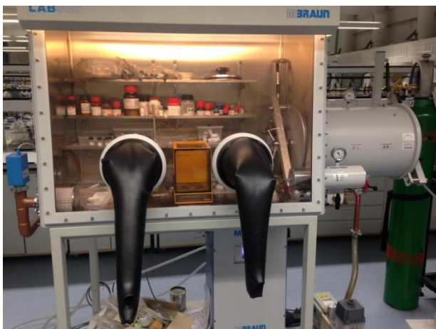
Figure 6.2: Photo of a typical research glove box.
