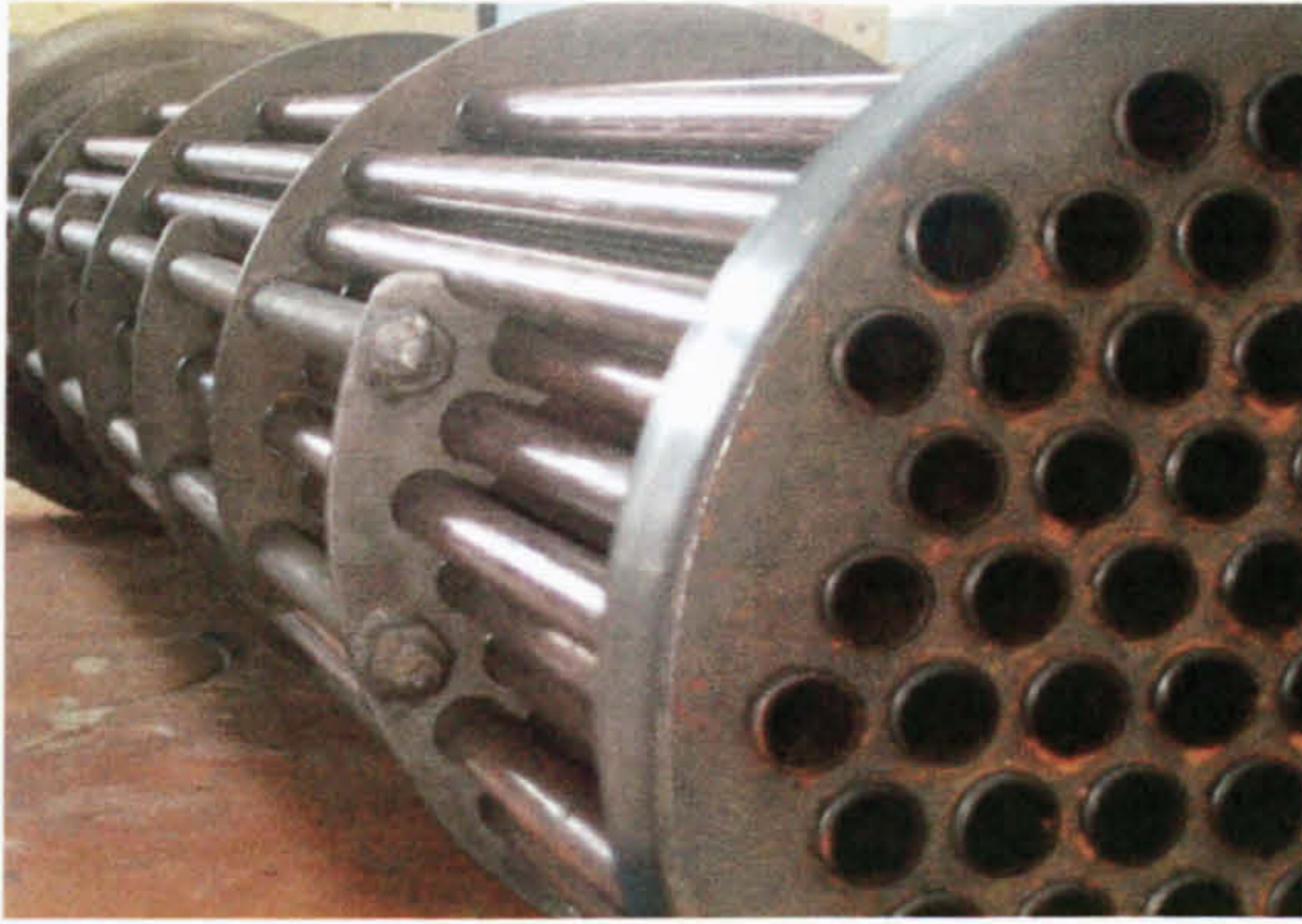
(a) – Tube Bundle with Baffles (Horizontal-cut)
