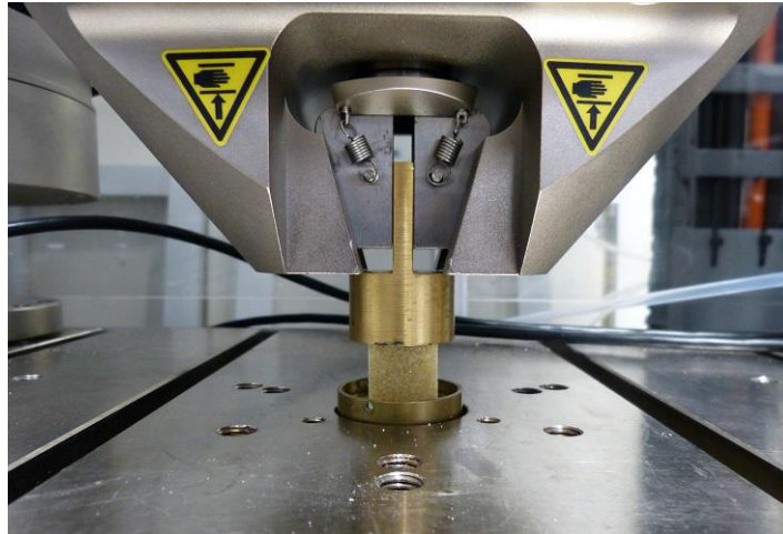
Figure 3-9 - Determination Of Elastic Modulus In Compression
