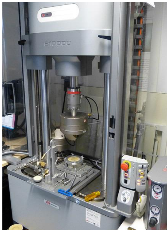
Figure 3-1 - Instron E10000 With Test Rig
