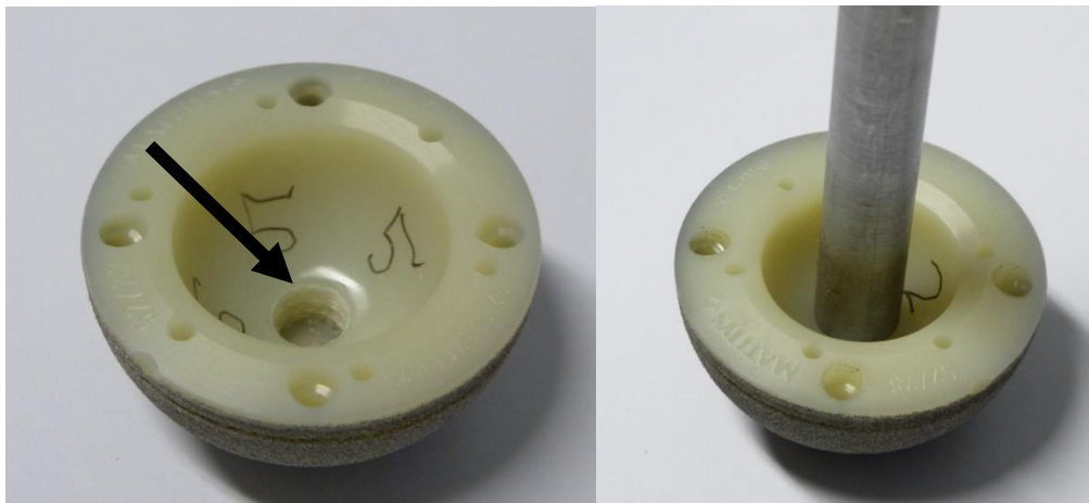
Figure 3-5 - Polyethylene Cup With Threaded Hole And Attachment
