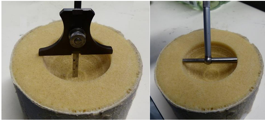
Figure 3-7 - Depth And Telescoping Gauge For Cavity Determination
