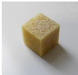
Figure 3-8 – Sliced Cubic Bone Substrate For Measurement Of Properties
