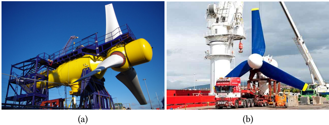
Figure 2.2: The commercial scale prototypes of the Andritz Hydro Hammerfest HS1000 (a) and the Atlantis Resources Ltd AR1500 ready for deployment at the full scale demonstration site in Pentland firth with the Meygen project. Images reproduced from http://subseaworldnews.com/ .
