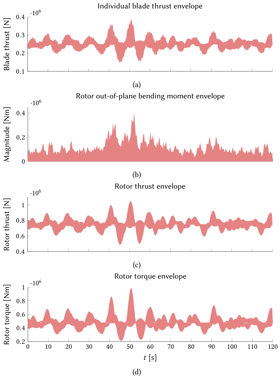
Figure 6.14: Load envelopes for the generic TST operating in irregular seas generated by superimposing the hydrodynamic loads from each load case defined in Table 6.5. The loads represented by these figures were fed as inputs to the full DoF drivetrain model. The figures show a large load peak present around 50s caused by the constructive interference large waves passing in sea-state 8.
