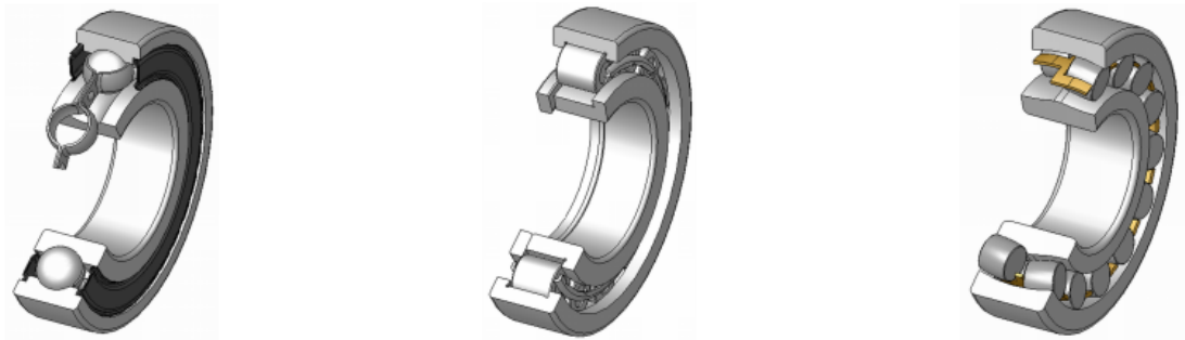
Figure 2.9: Three common types of rolling element bearings showing the outer raceway, rolling elements, cage and inner raceway. (From left) Ball bearing, cylindrical bearing and spherical roller bearing. Wind turbine components are shown due to the difficulty of finding publically available TST component images. Reproduced under licence from https://creativecommons.org/licenses/by/2.5/deed.en
