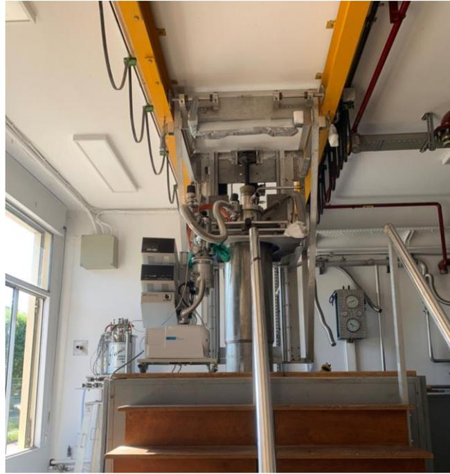
Figure 7.17: High field magnet for HTS double-pancake coil magnetization
