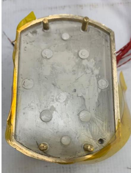
Figure 3.6: Finished HTS -stacked ring magnet sample with impregnation (without cover)
