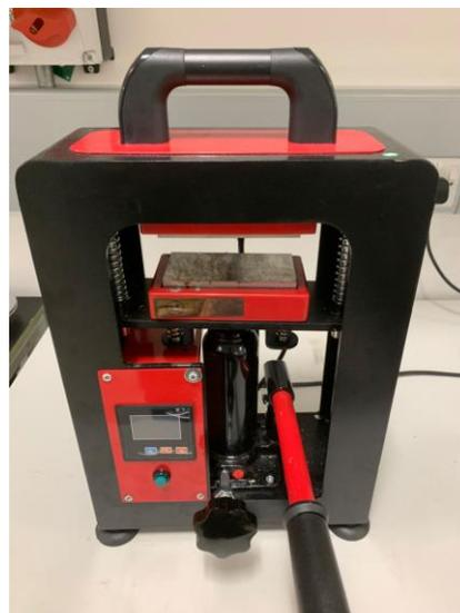
Figure 7.9: Heating and pressing machine for soldering joints
