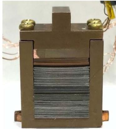
Figure 2.15: HTS stacks that trapped 17.89 T at 6.5 K
