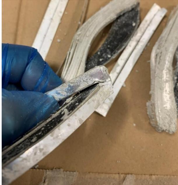
Figure 6.1: Damaged HTS-stacked ring magnet after FC magnetization
