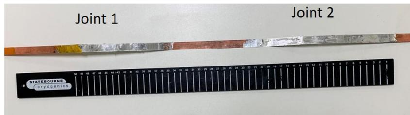
Figure 7.10: The soldered bridge-type joints
