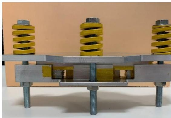
Figure 5.2: The pressure mould for fabrication of HTS stacks
