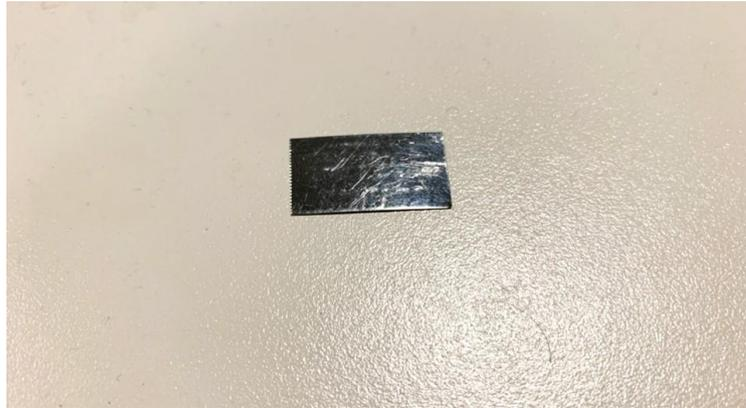
Figure 5.1: A piece of HTS tape with PbSn coating
