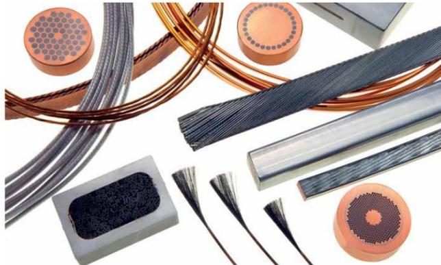
Figure 2.1: Products based on LTS materials
