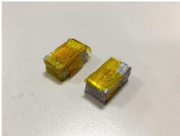
Figure 5.4: Soldered HTS stacks
