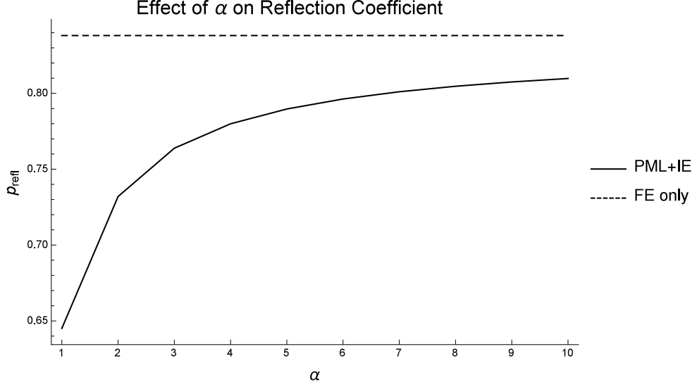
Figure 3.9: The effect of the stretching function parameter \alpha in equation (3.6) on the reflection coefficient calculated via equation (3.234) for both the FE only formulation (dashed line) and the PML+IE formulation (full line) with constant stretching for a steel waveguide, n_1 = 201 nodes in length, with the stretching function parameter \beta = 10 .
