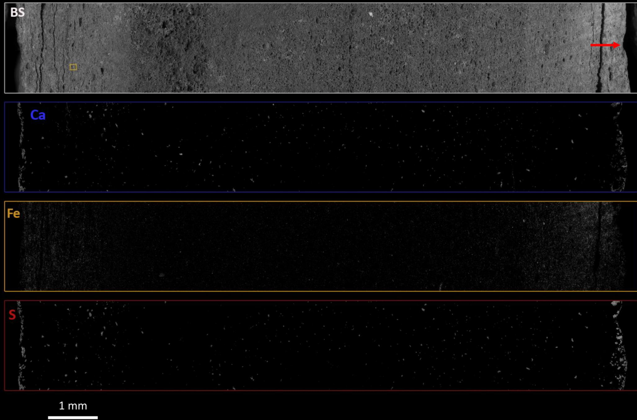
**Figure 5.18** LVSEM backscatter (BS) image and EDX maps for selected elements of the unreacted B1 chip. Red arrow in the BS image indicates a feature serving as a marker between before and after leaching images.
