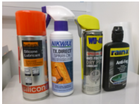
Figure 4.1 Hydrophobic coatings used to try and prevent fouling of the sample chute
