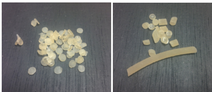
Figure 5.2 Example of pellets produced by a pelletizer for samples 1,2 and 3 (left) and example of manually cut pellets used for pellet analysis of samples 4 – 19 (right).
