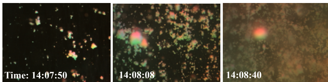
Figure 4.14 Fouling over 50 seconds of running at 2 kg h -1 400 rpm
