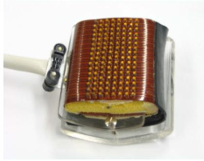
**Figure 2.7** – An example of an early high-density sEMG array as developed by Blok et al.<sup>2</sup> ©2002, American Institute of Physics.
