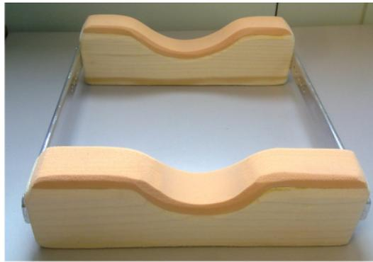
**Figure 6.2** – Two foam covered blocks were used as armrests. The base of each was made from wood and two metal rods maintained a fixed difference. The rods had various holes in the ends so that the separation of the blocks could be adjusted for physiological variation in arm length.
