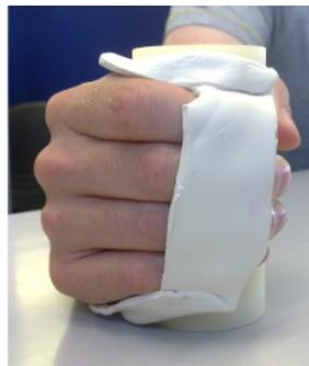
**Figure 6.3** – A thermosetting acrylic sheet was cut and moulded around a hollow cylinder. A slit allowed the finger tips to slide underneath a section, thus isometric extension and flexion of the fingers was possible. A cord looped through the cylinder and provided isometric resistance against thumb extension. During the experiment the device was mounted to a rod in the desk (not shown).
