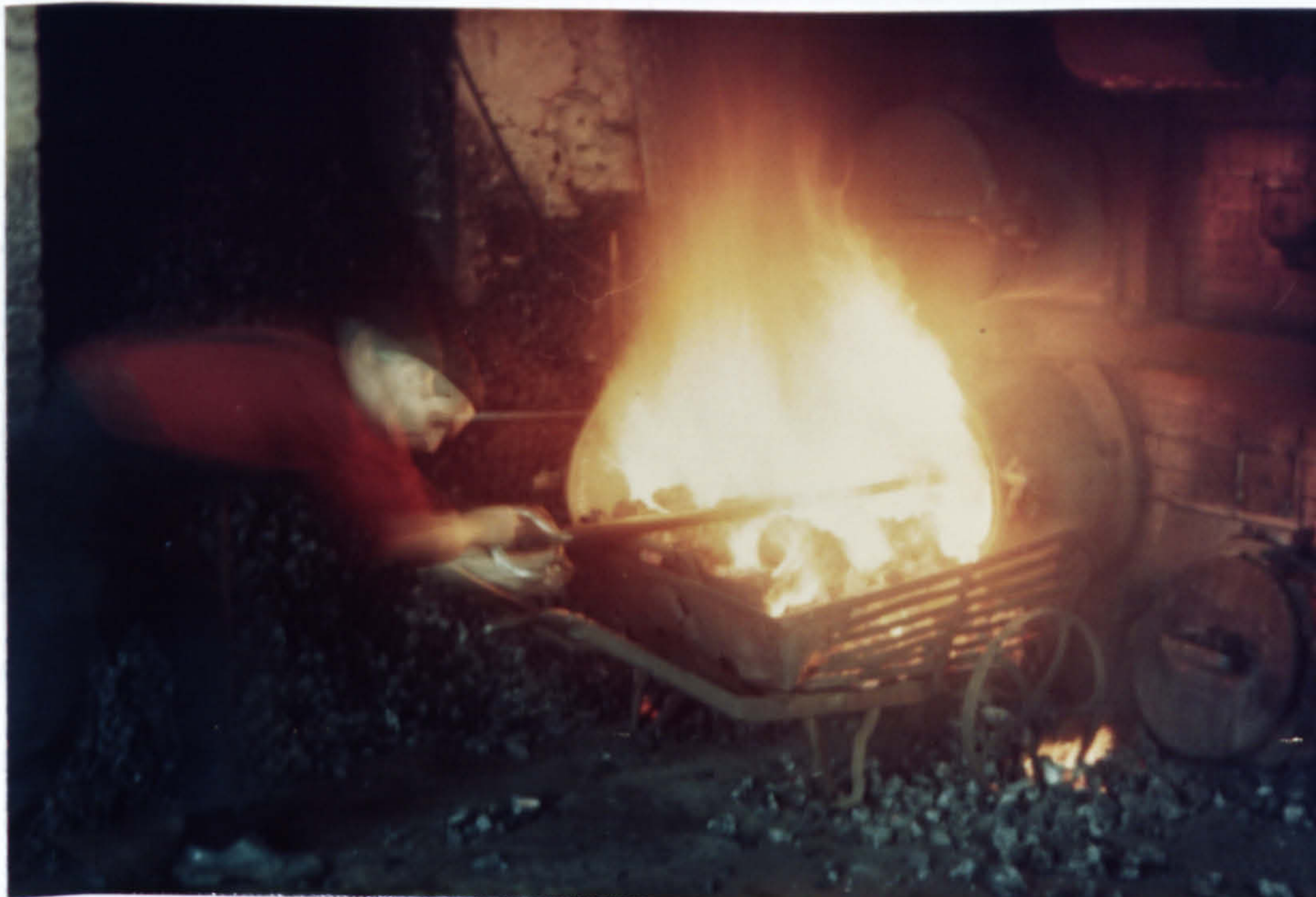
Raking incandescent coke from retort into iron coke-barrow.
