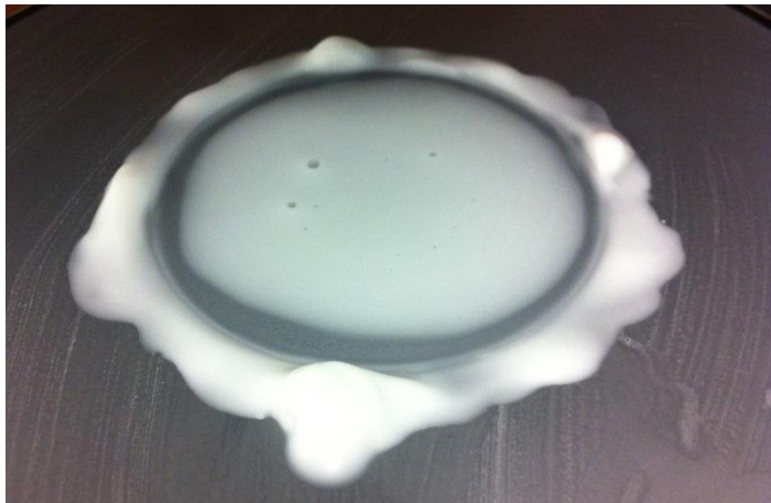
Figure 7.20- Material ejected from rheometer during DST at mass fractions >0.54 , showing granules
