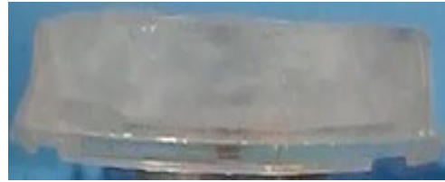
Figure 3.15- 20% v/v glycerol-water mixture at 500RPM with rheoscopic fluid
