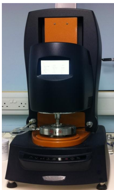
Figure 7.8- Rotational rheometer (TA Discovery HR-2) used for experiments (left) and its parallel plate geometry (right)
