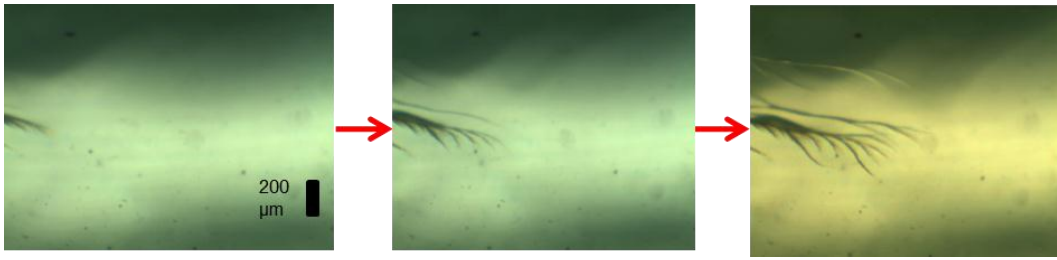
Figure 4.5- Example microscopic observation (5x magnification) in 5mm gap shear cell showing growing cracks. \Phi=0.59 ; 72.4 \text{ N/m}^2 stress. Time gap between images was approximately 0.05s.
