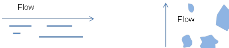
Figure 3.11- Rheoscopic fluid mechanism. Flow along observer's line of sight (left). Flow perpendicular to observer's line of sight (right).
