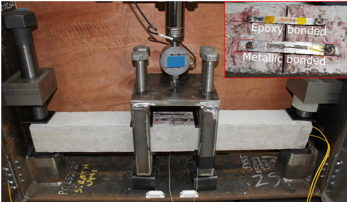
Figure 7.17: Experimental setup of concrete crack monitoring fatigue test. Insert: sensor attachment.
