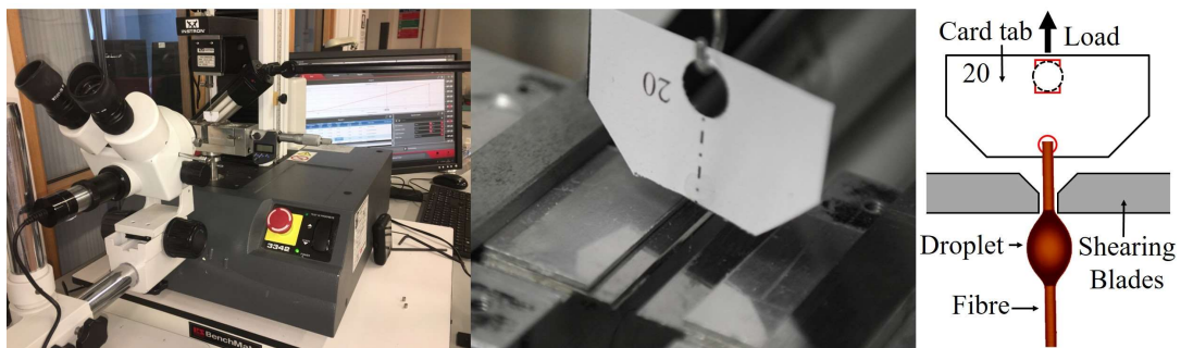
Figure 2:7: Microbond test experimental jig
