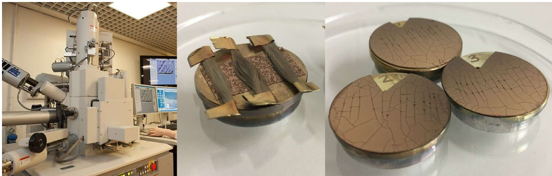
Figure 2:9: Scanning electron microscope, fibre bundle, and mounted/coated microbond droplet SEM specimens.
