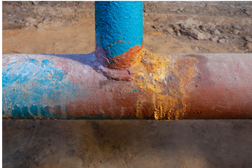
Figure 2.4: Example of corrosion on a pipe at a saddle weld 3
