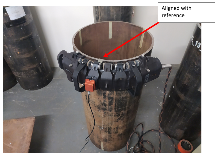
Figure 7.11: Spyne setup on a vertical pipe with the MTi-100 IMU attached
