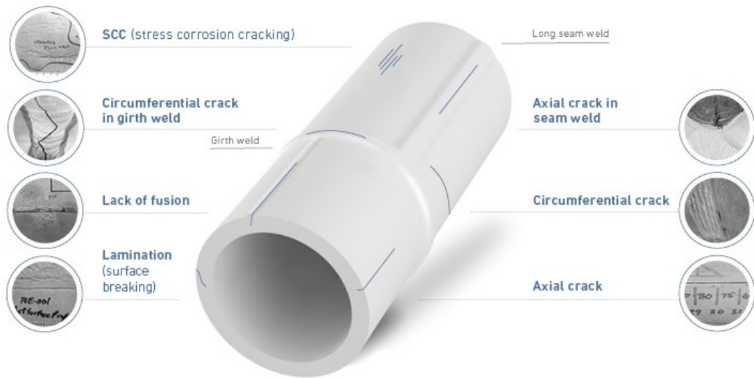
Figure 2.5: Example of different types of crack on a pipe 4
