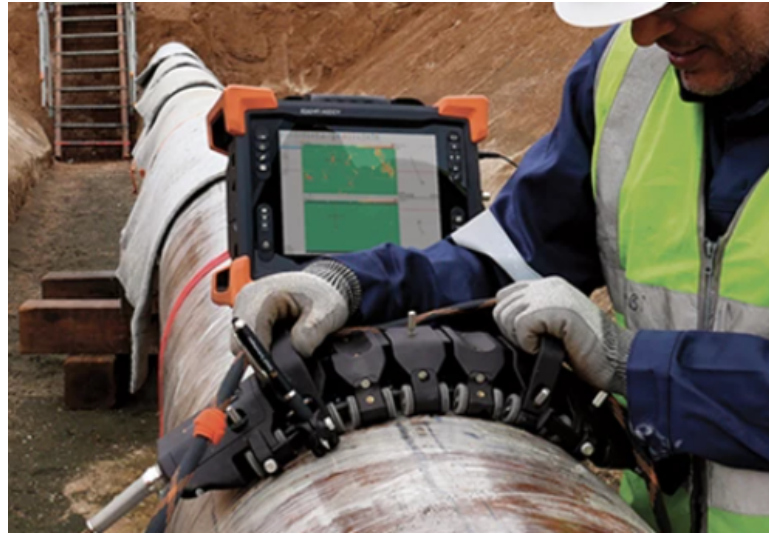
Figure 7.1: An image of the Eddyfi Spyne system being used in field.
