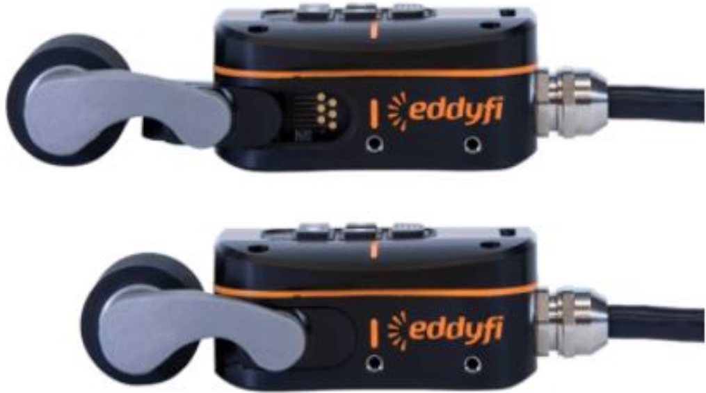
Figure 2.23: Eddyfi PEC Probe with Encoder 16
