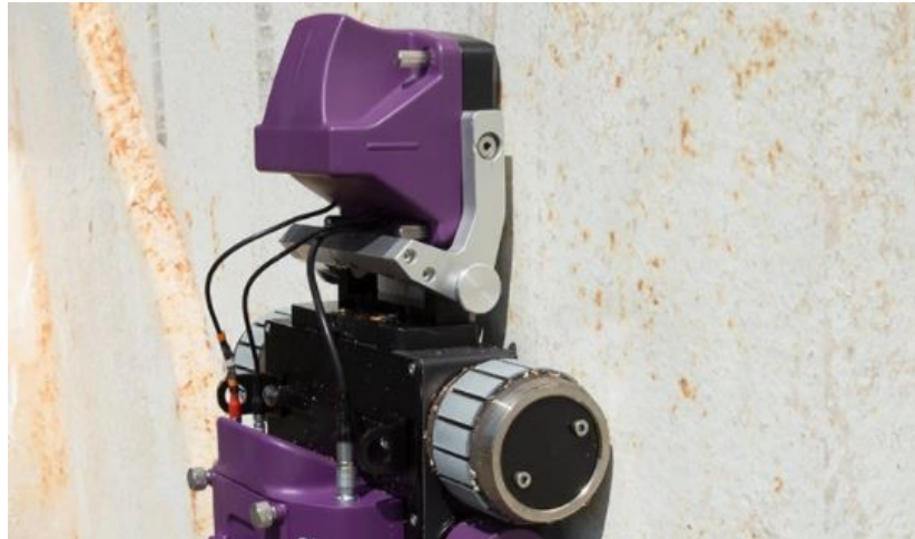
Figure 2.20: Scorpion 2 using Magnetic Wheels with Rubber Coverings 13
