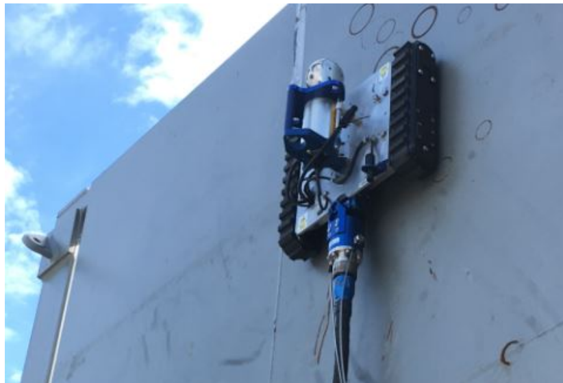
Figure 2.21: Magg 480 using Magnetic Tracks 14
