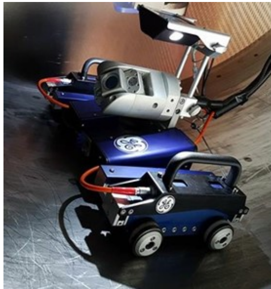
Figure 2.32: Petrobot GE Fast Platform [90]
