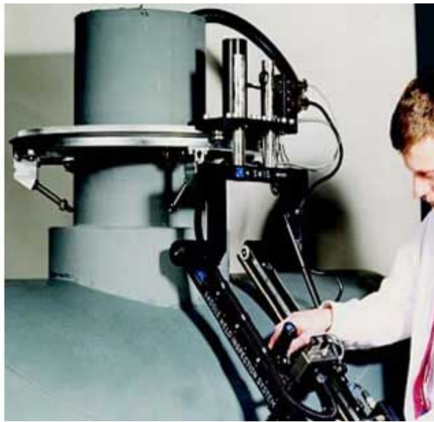
Figure 2.16: Phoenix SWIS Saddle Weld Scanner 9
