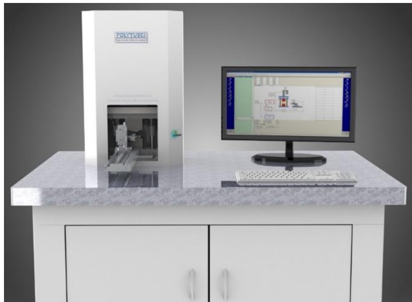
Figure 104. The final model of hot embossing machine system
