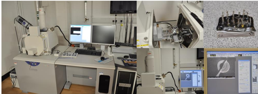
Figure 68. The SEM equipment, the sample preparation and observation
