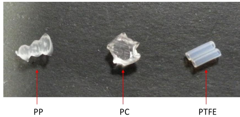
Figure 31. Polymer samples after DSC test
